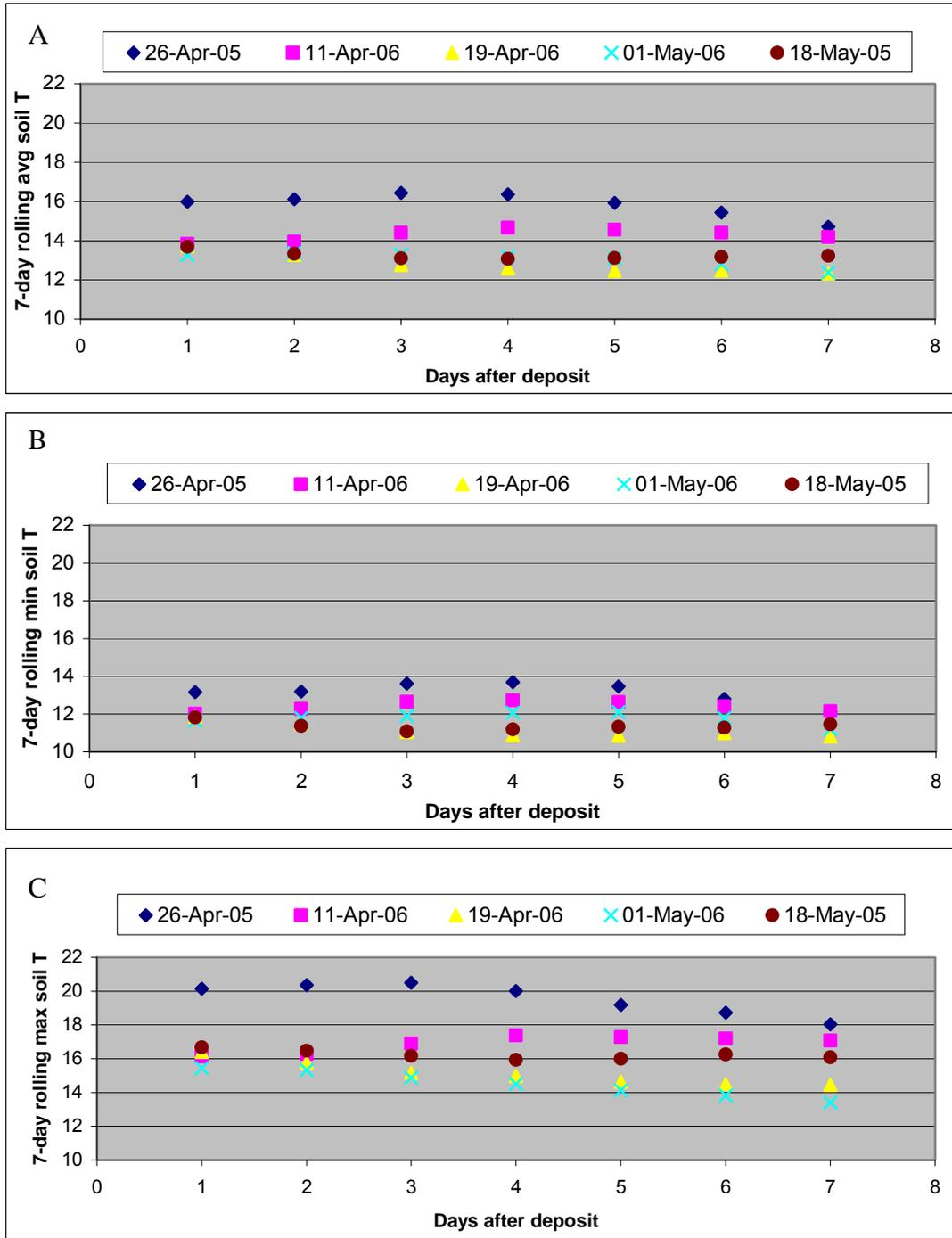
Figure 3-7 The 7-day rolling average (A), minimum (B) and maximum (C) soil temperatures ( $^{\circ}\text{C}$ ) for each day of the week following the deposits on 26 April 2005, 18 May 2005, 11 April 2006, 19 April 2006, and 1 May 2006
