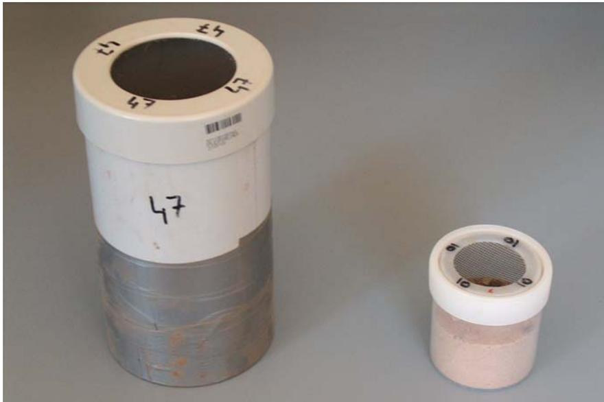
Figure 2-2 Field pot (left) and laboratory pot (right)
