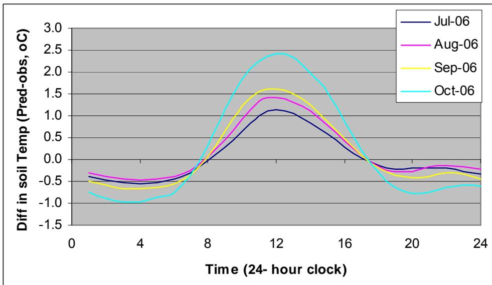
Figure 5-5 The difference between the average hourly soil temperatures predicted by FlyAlert and the soil temperatures measured at the experimental site for July to October in 2005 (A) and 2006 (B)
