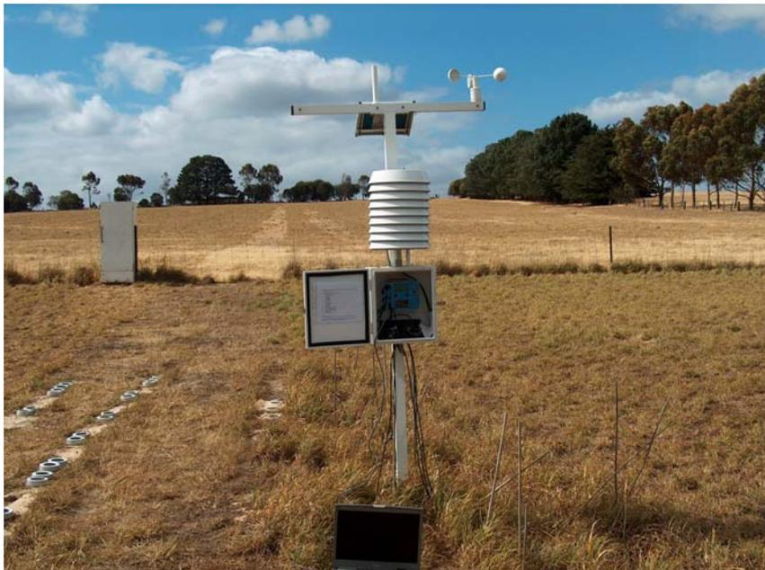
Figure 2-6 The solar powered weather station and data logger located at the centre of the experimental site, immediately adjacent to the field pots
