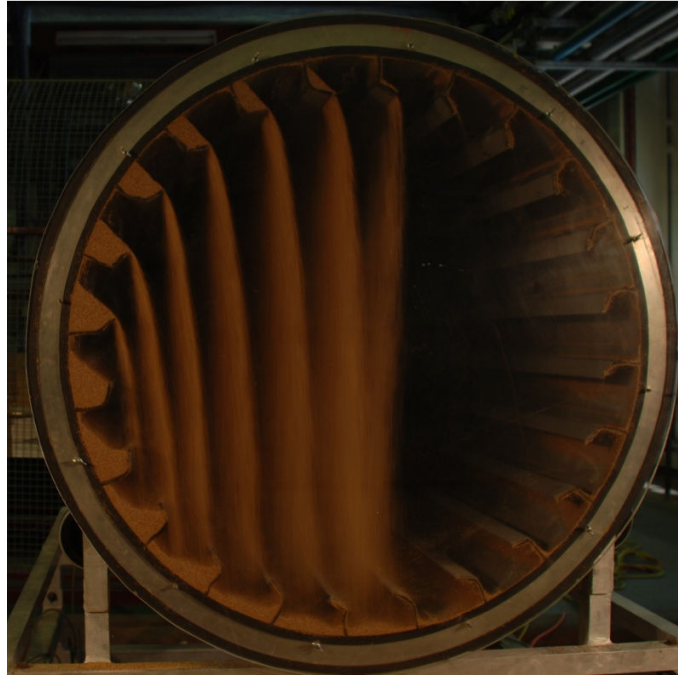
Figure 1.2: Cross-section of typical flighted rotary dryer showing the solids cascading
