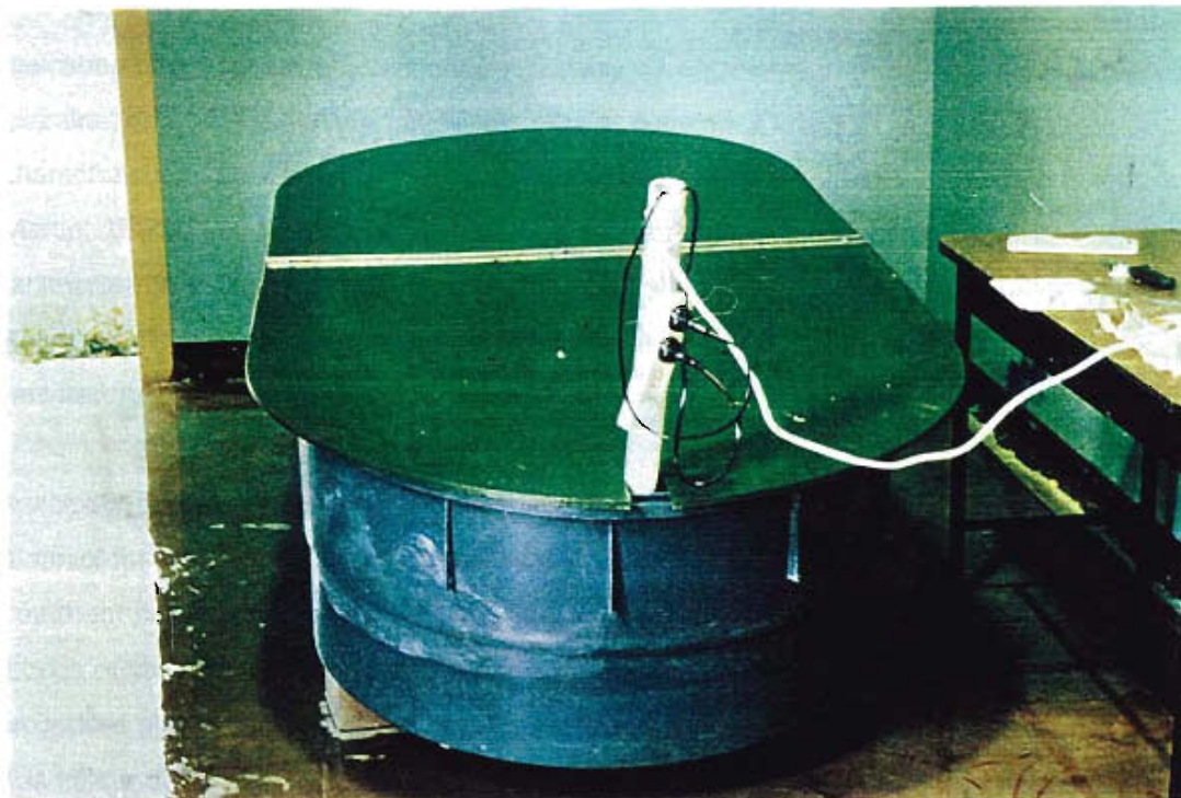
Figure 6.1 A plastic oval tank covered with a marine ply lid was used to keep the animals in the pilot transmission experiment and in the third transmission study. The power point on the pole was connected to two immersion heaters, which provided a temperature of 32°C.
