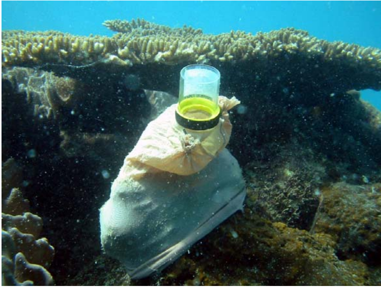
Fig. 4.1. Larval trap that is placed over adult sponges used to collect larvae.
