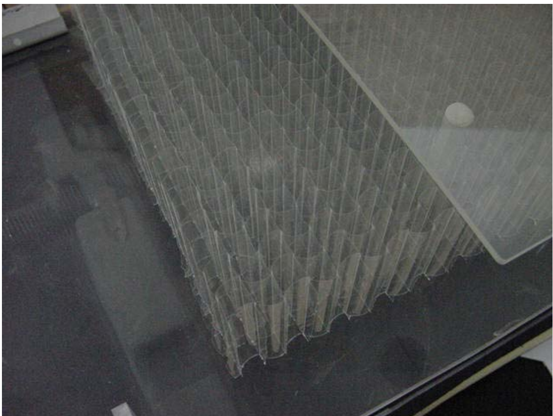
Figure 3.5. 50 mm high honeycomb material in cutaway section of a solar collector
