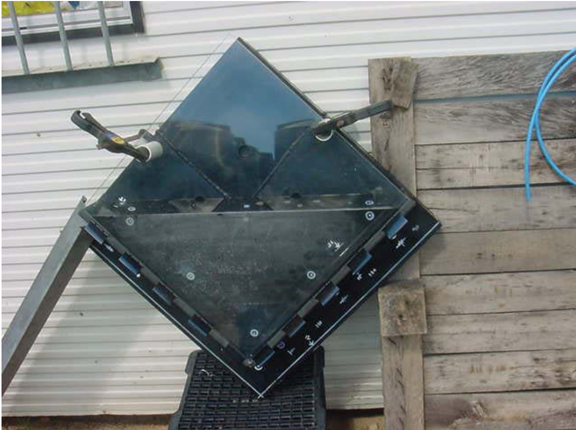
Figure 8.4. 50 mm fold back clips clamping glazing onto prototype base with 6 mm o-ring (trial section filled with water – approximately 300 mm head).
