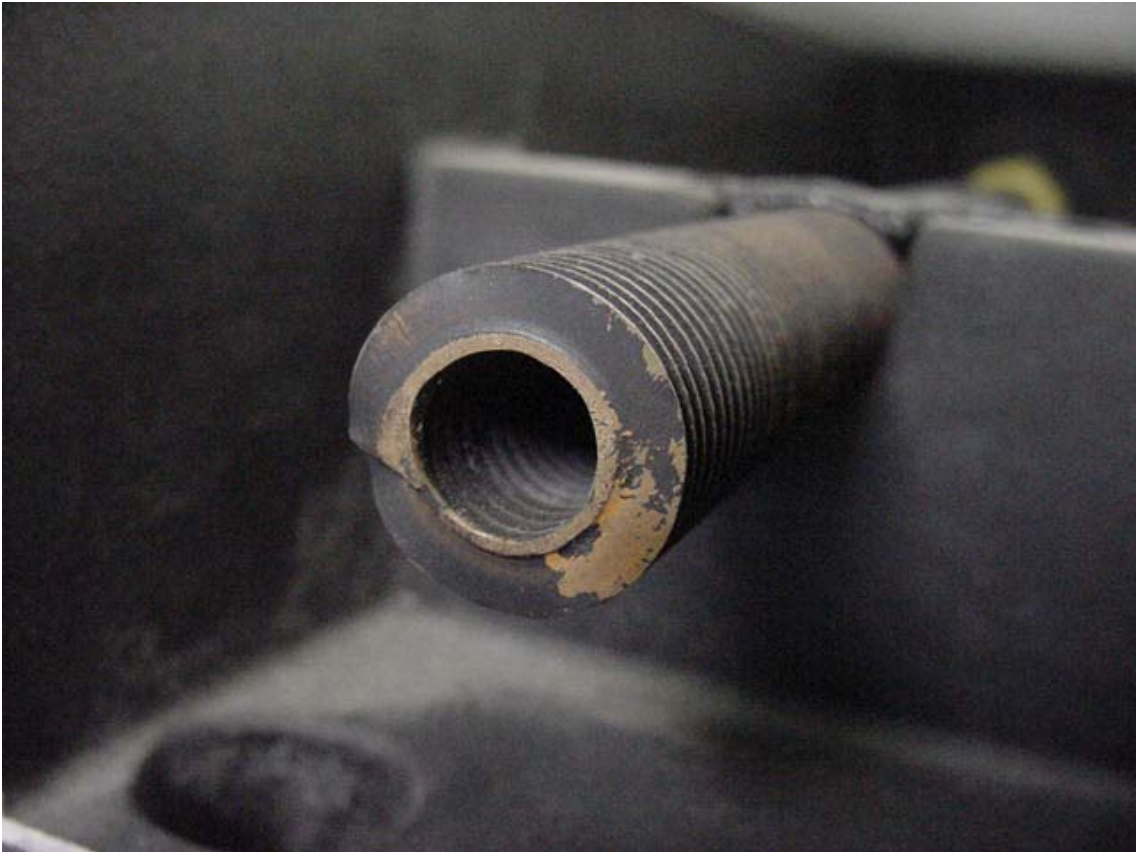
Figure 5.4. Photograph showing undulating inner tube surface
