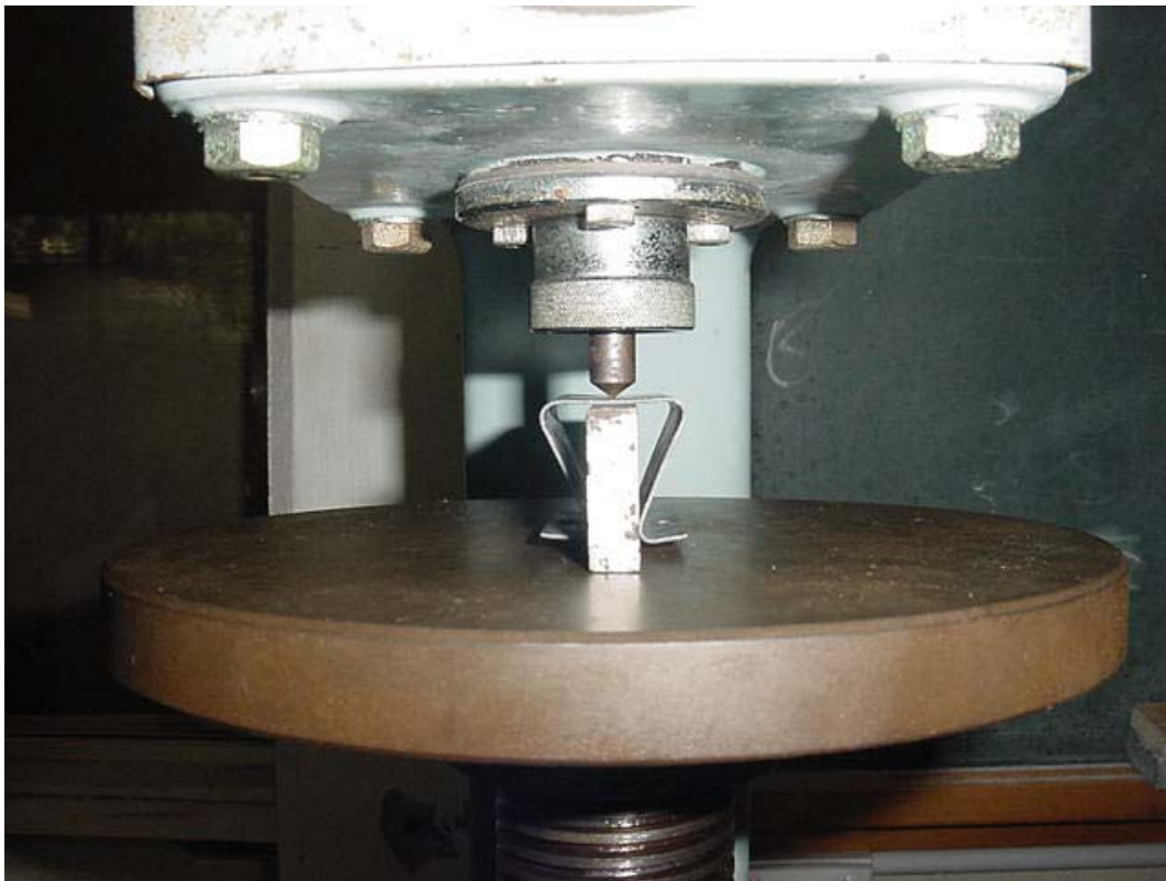
Figure 8.7. Clip being tested for Rockwell hardness at JCU.
