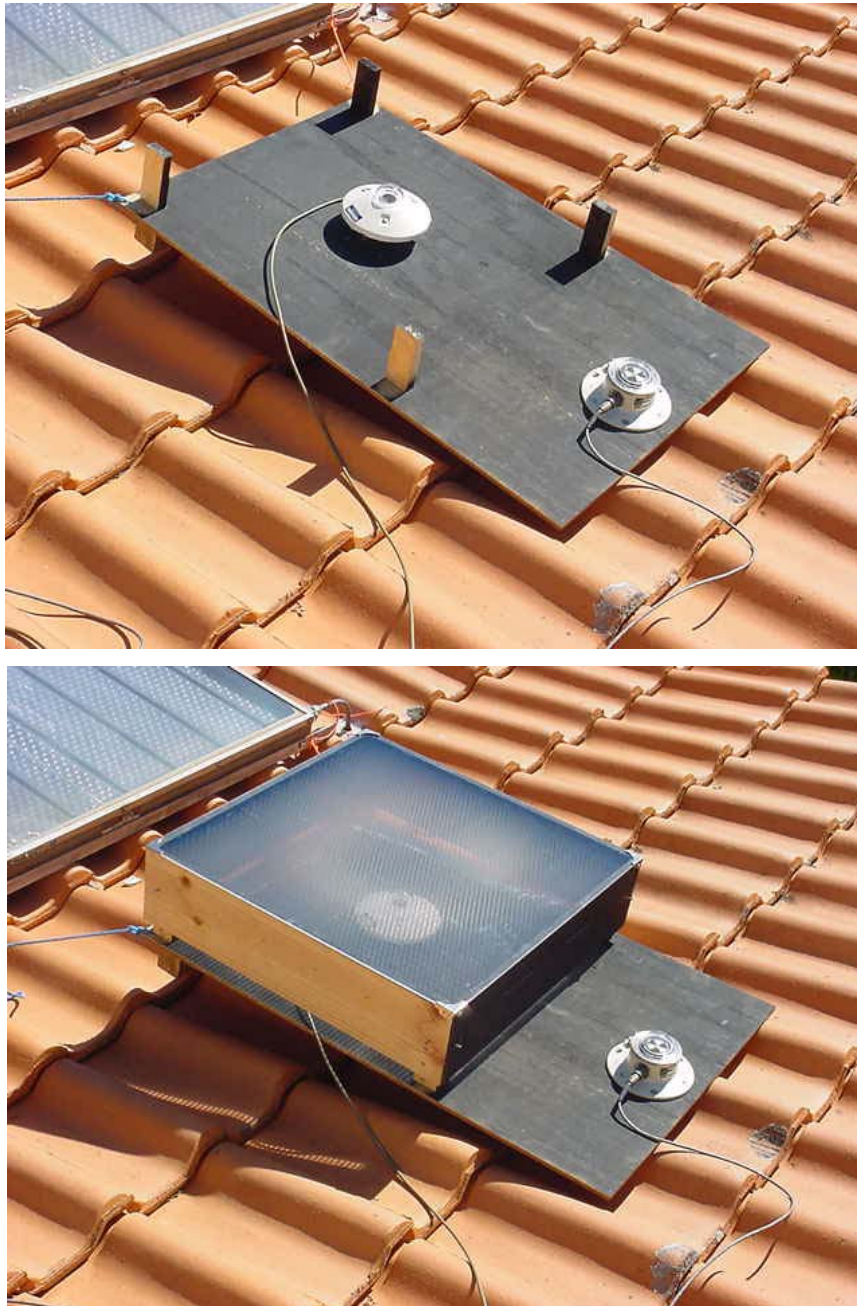
Fig. B.1. Apparatus for the transmission test of the top cover system (3 mm acrylic cover + 50 mm cellulose acetate honeycomb).
