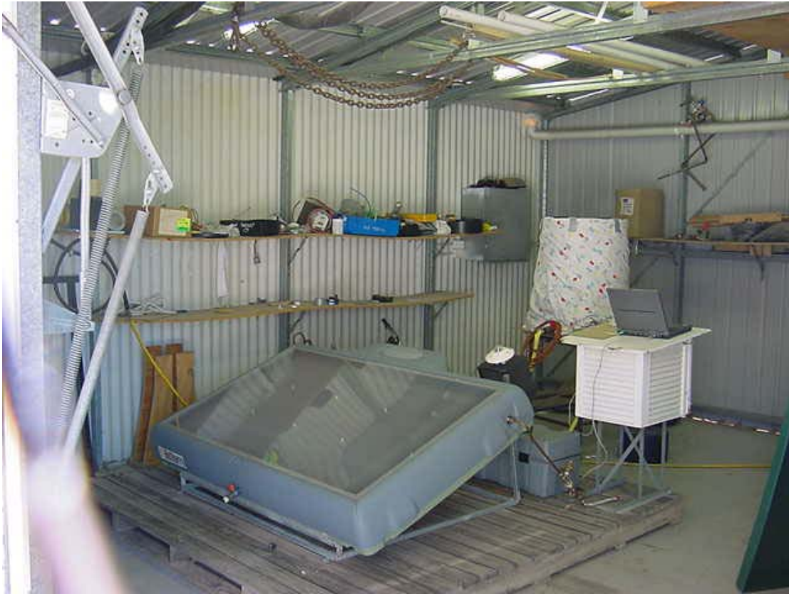
Fig. 3. Experimental set up for indoor heat loss test
