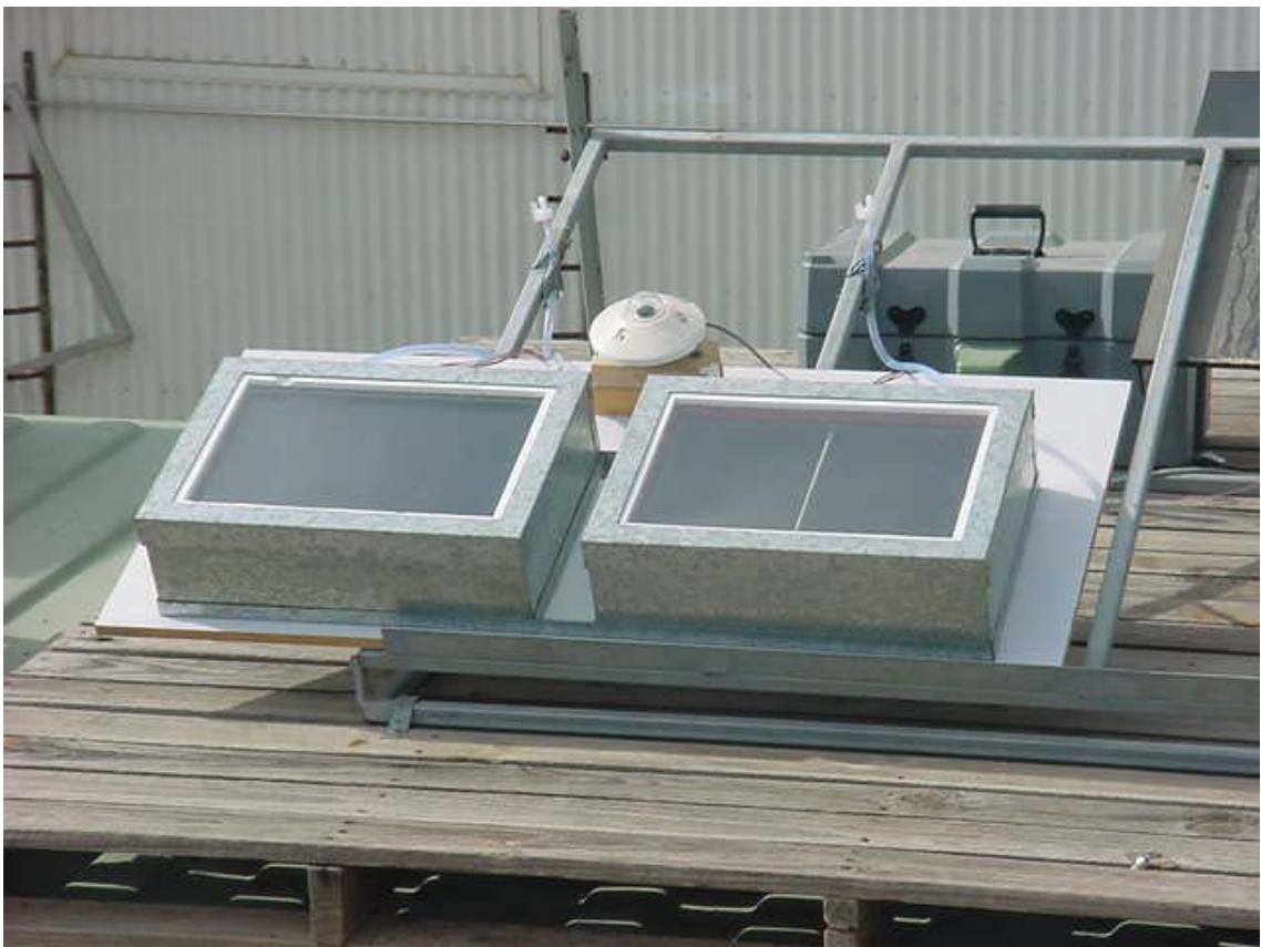
Figure 6.8. General arrangement of experimental apparatus at 20° tilt angle
