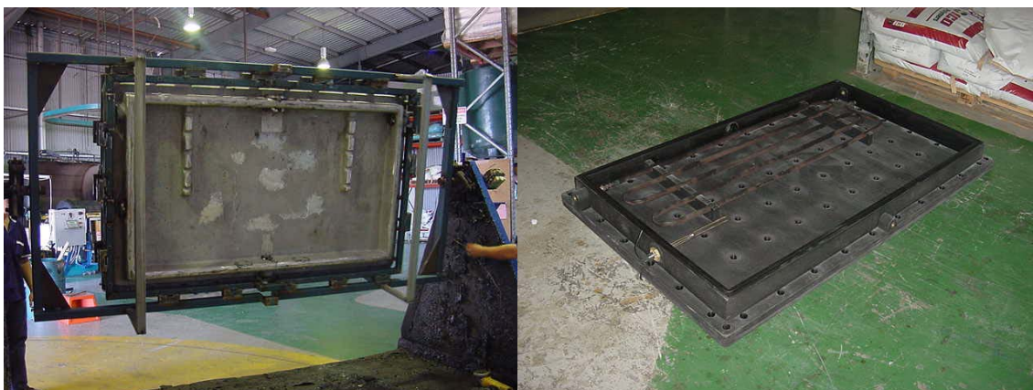
Figure 7.2. Photographs of the cast aluminium base mould and the first product from the mould
