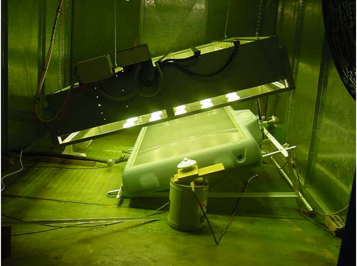
Fig. 1. Hot Harry™ indoor performance testing at P.T.L. with low iron glass filter.
