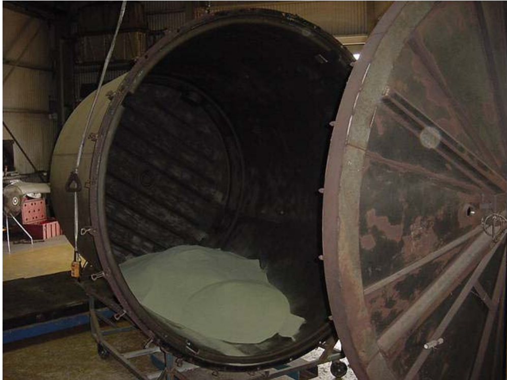
Figure 7.3. Photograph of 9000 litre tank mould loaded with polyethylene resin
