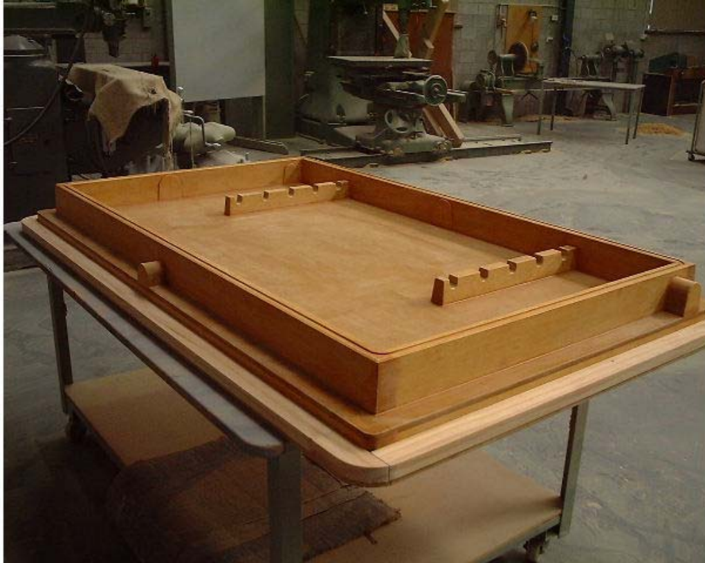
Figure 7.1. Photograph of a timber plug for a cast mould
