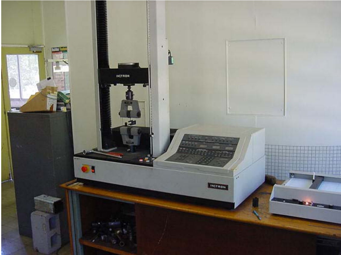
Figure 8.6. Clip being tested on Instron materials testing machine at JCU.
