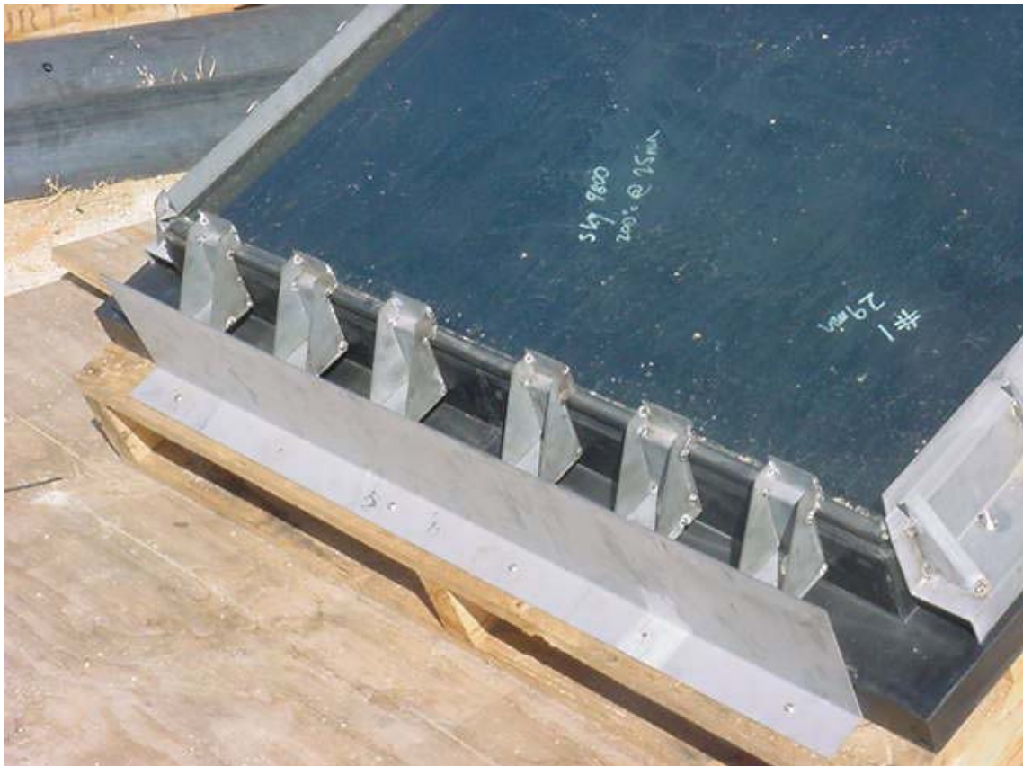
Figure 8.1. Early prototype collector with two variations of bolted clamps to retain inner glazing.
