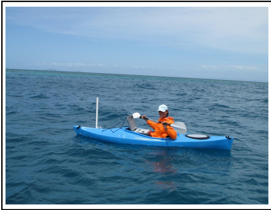
Fig. 3.2: Manual acoustic tracking carried out from a 3m kayak (Dagger Drifter) with acoustic hydrophone (Vemco V110) mounted to bow and acoustic receiver (Vemco VR100) positioned within cockpit. Kayak can be manoeuvred through 360° to pick up direction of signal and then paddled in direction of tagged individual until signal gain is maximised. GPS is then used to mark the location of the individual fish every 15 minutes.
