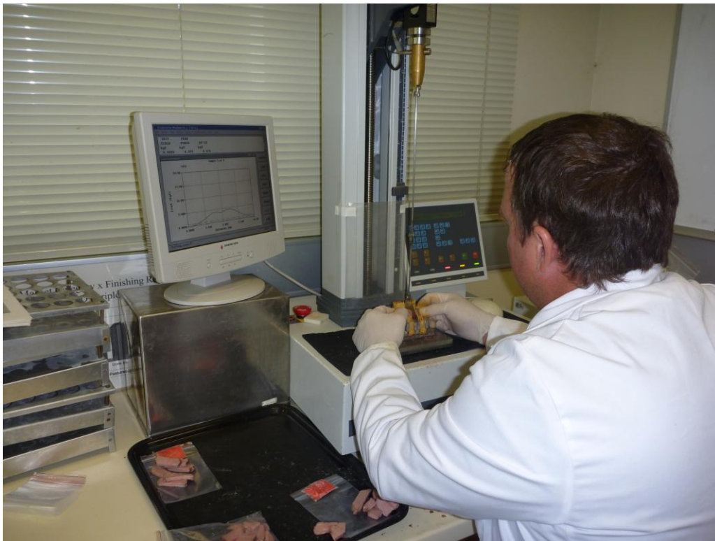
Figure 5.1. Performing the Warner Bratzler Shear Force assays at The University of New England's Armidale meat science laboratory
