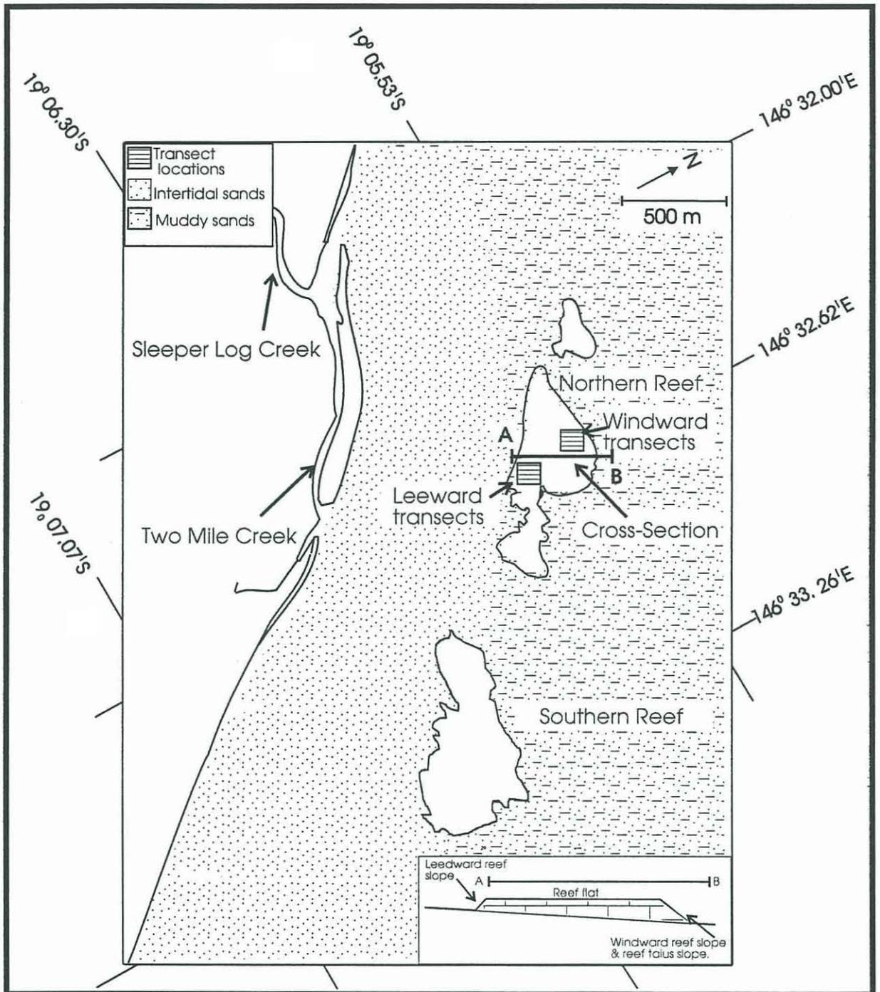
**Figure 4.1.** Transect locations from Paluma Shoals and schematic cross-section. The grids represent the location of the transects from the windward and the leeward reef flat. Each 10 m transect were taken SW-NE or shore-normal.
