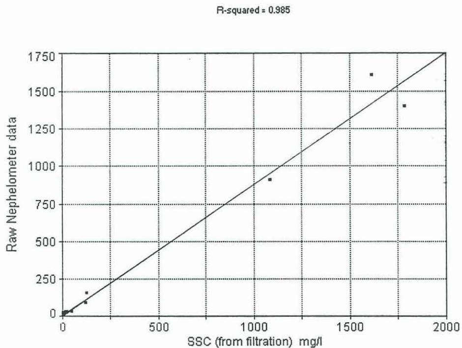
**Figure 3.5.** Calibration curve between raw nephelometer output and SSC as determined by filtration of water samples (From Larcombe *et al.*, 1995).
