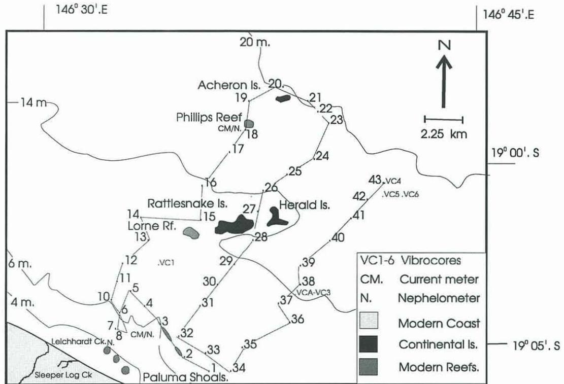
**Figure 3.1.** Positions of seismic lines, seismic stations, vibrocores, current meters and nephelometers.
