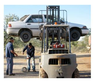
Plate 3.6 Exhaust system on the field vehicle being resecured with baling wire at Adels Grove near Riversleigh
