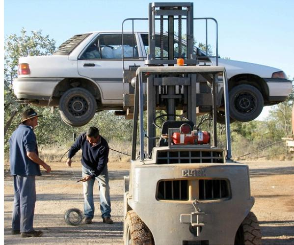
**Plate 3.6 Exhaust system on the field vehicle being resecured with baling wire at Adels Grove near Riversleigh**
