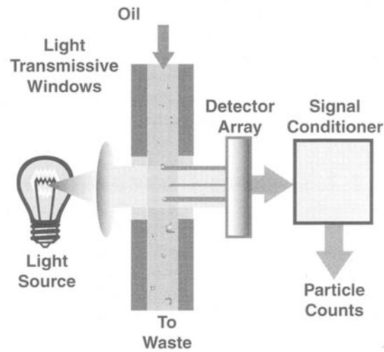
**Figure 2.12:** Operation of light extinction particle counters [3].
