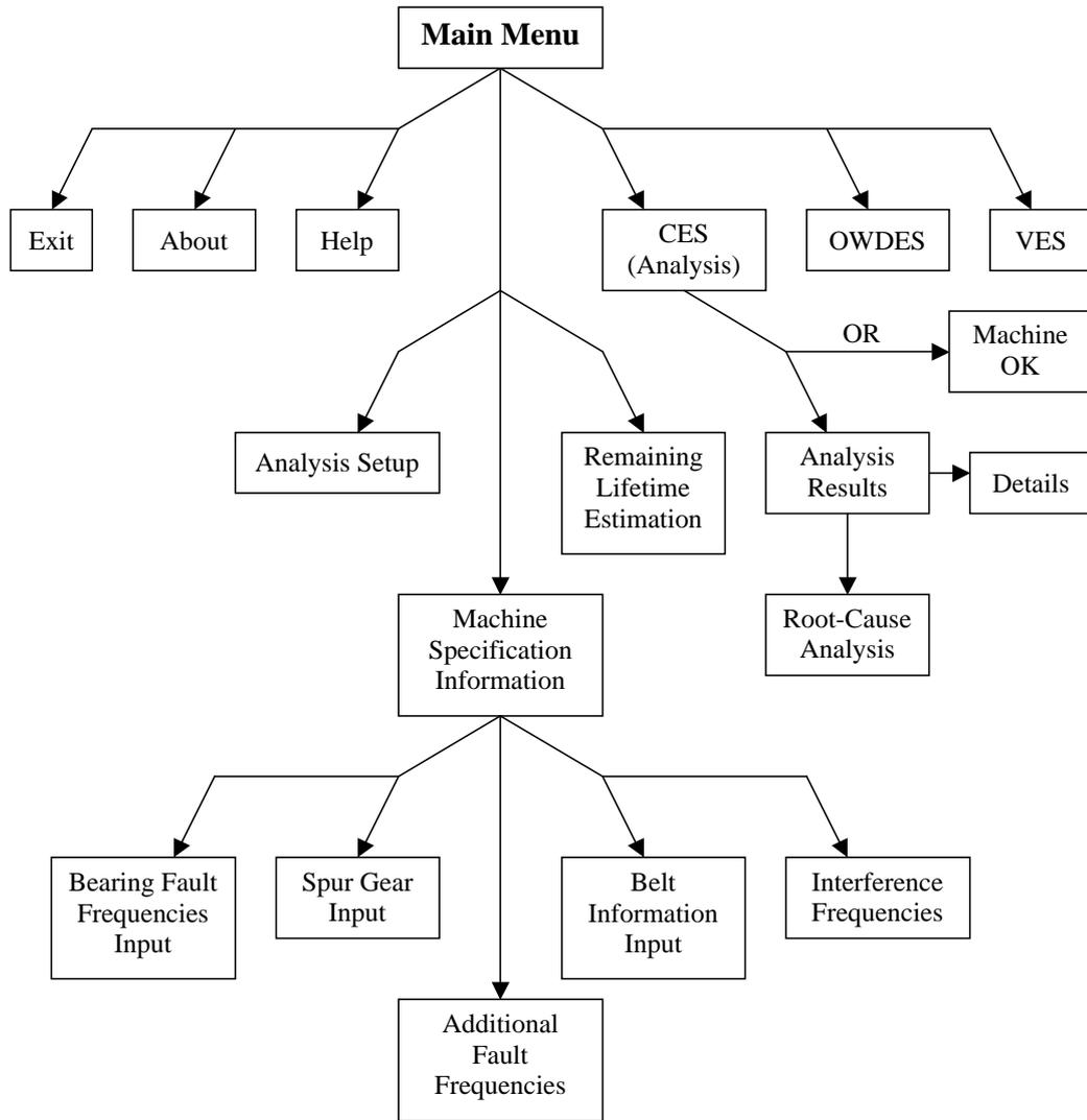
**Figure H.1:** Schematic diagram of the Main menu. OWDES and VES have individual schematic diagrams shown in Sections H.3 and H.4.
