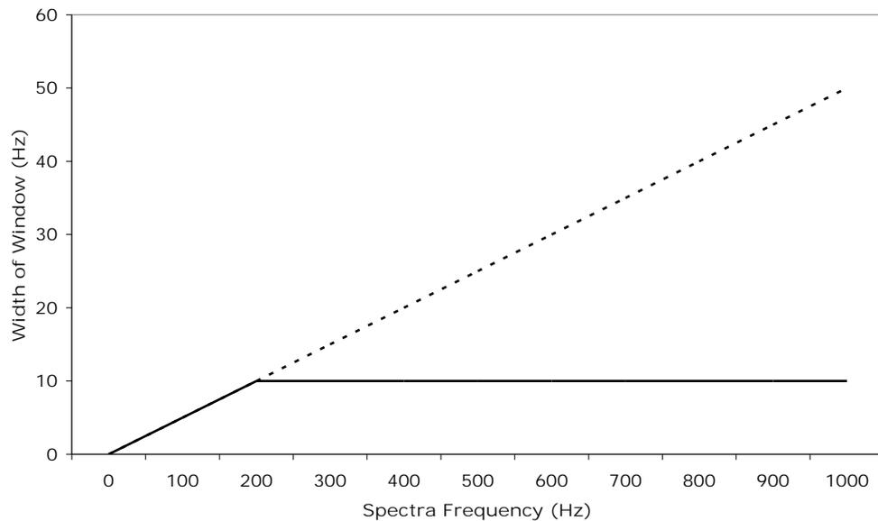
**Figure 5.5:** *The influence of the percentage deviation and maximum size in Hz factors on the frequency window used to detect peaks in frequency spectra. Solid line is window size limited by both factors, while dotted line shows window size without maximum size limit. In this figure, the ‘percent deviation’ is 5 %, while the ‘maximum size in Hz’ frequency window is 10 Hz.*
