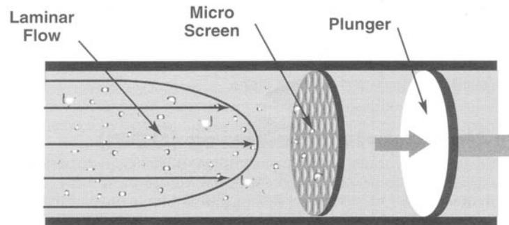
**Figure 2.13:** Flow decay counter principle [3].
