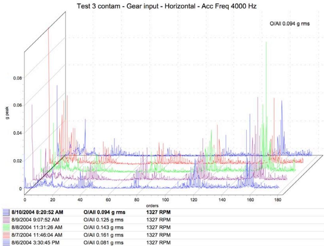
Figure 4.13: Waterfall plot of acceleration spectra from the contamination test.
