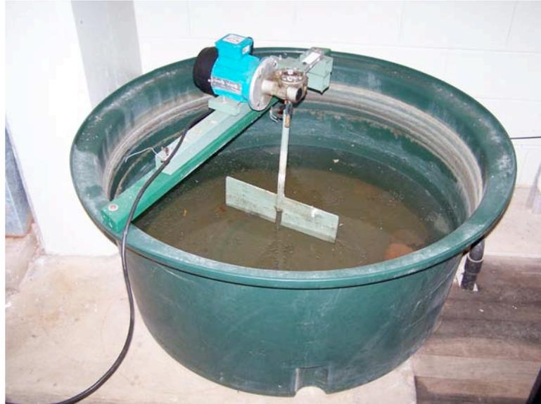
**Figure 3.2:** *Photo of the worm gearbox test rig. Note that the water level is not at operating level, and the strain gauge is not connected to the wheatstone bridge at the time of the photo.*
