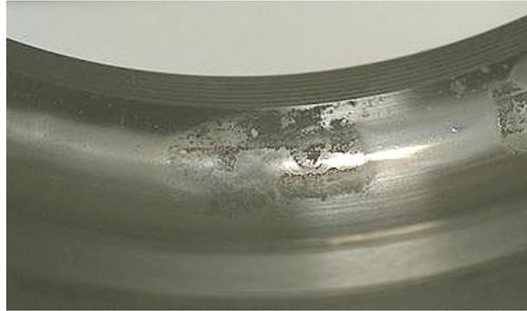
**Figure 2.20:** *Deep seated rust development in the outer ring of a deep groove ball bearing [50].*
