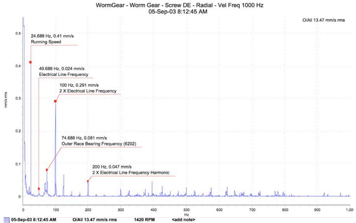
**Figure 4.20:** Velocity-frequency spectrum at the drive end of the worm gearbox for the lack of lubrication test.
