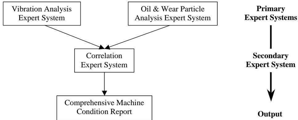
**Figure 3.3:** *Data process flow chart of the expert systems.*
