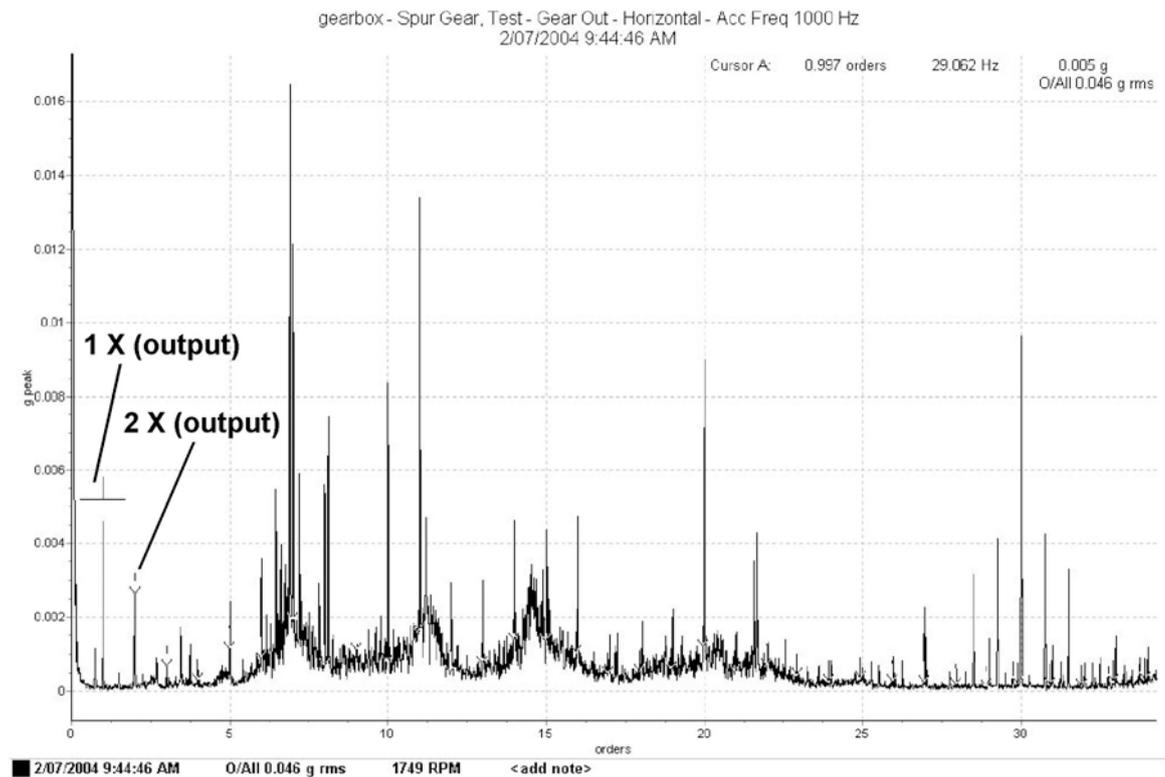
**Figure 5.11:** 1000 Hz horizontal acceleration spectra (at output gear) of worn spur gears with a bent output shaft.
