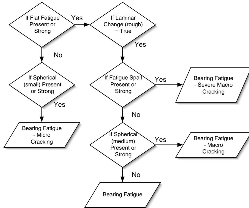
Figure D.12: Bearing Fatigue.
