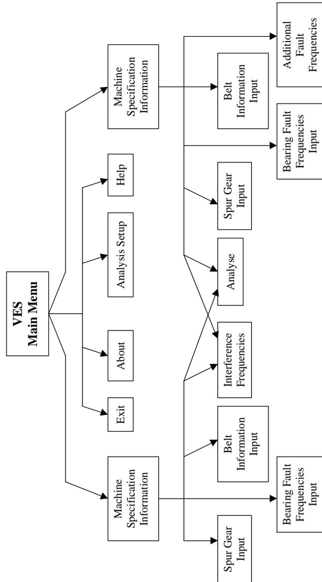
Figure H.20: Schematic diagram of the VES menu structure.
