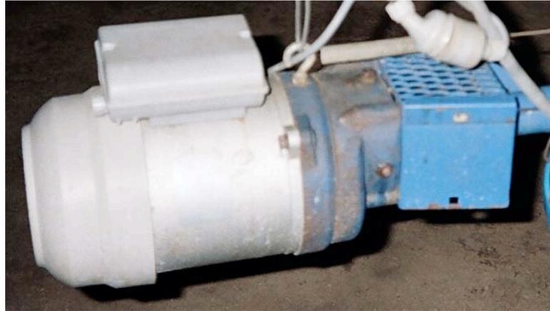
**Figure 7.9:** *Photo showing grain auger gearbox and close coupled electric motor.*
