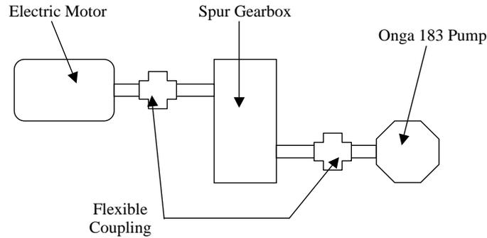
**Figure 3.1:** Schematic diagram of the experimental spur gearbox test rig.
