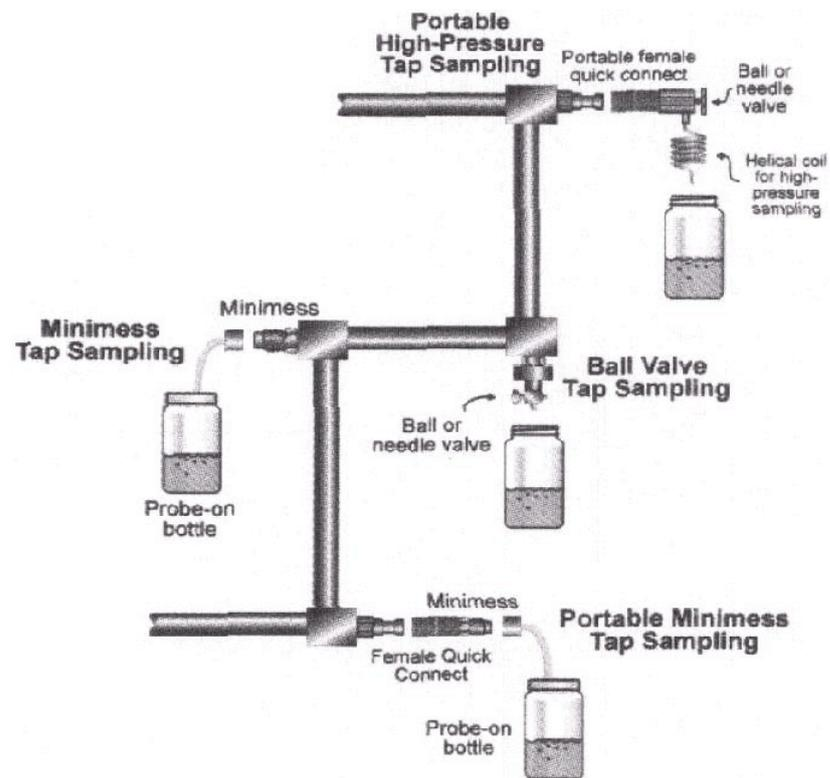
Figure 2.8: Common sampling arrangements from pressurised lines [9].
