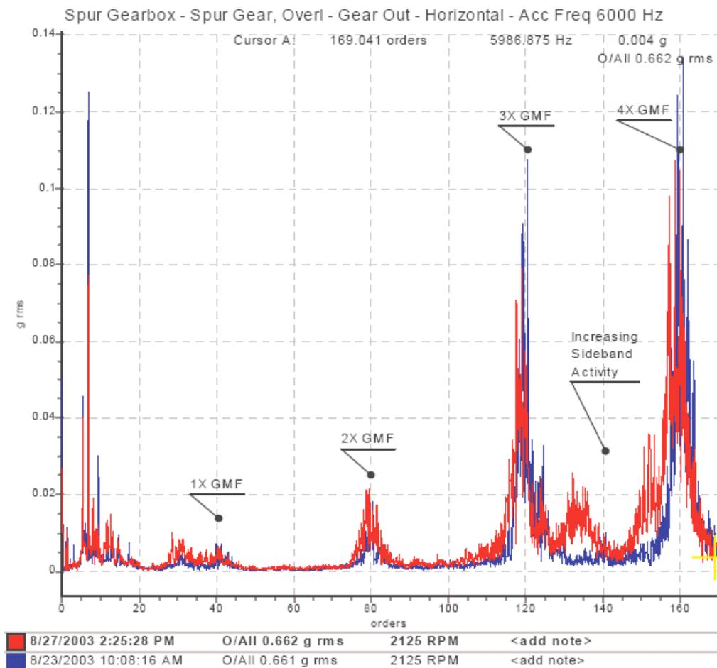
Figure 4.10: Vibration spectra of output gear collected during the cyclic load test.
