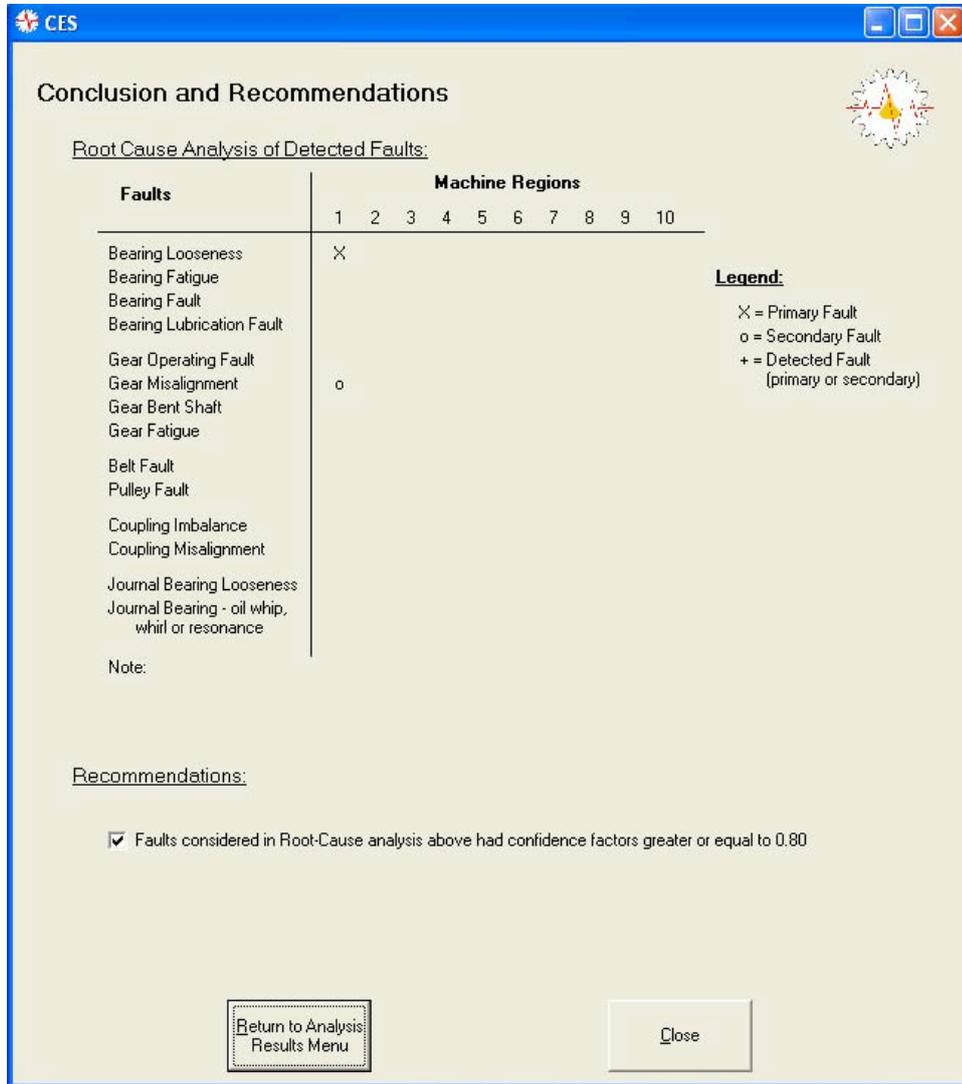
**Figure H.13:** The Root-Cause Analysis results window, showing an example where bearing looseness caused gear misalignment.
