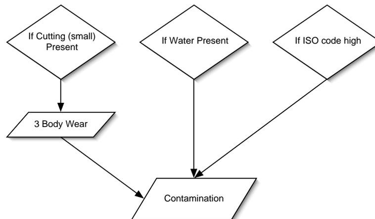
Figure D.3: Contamination (3 body wear).
