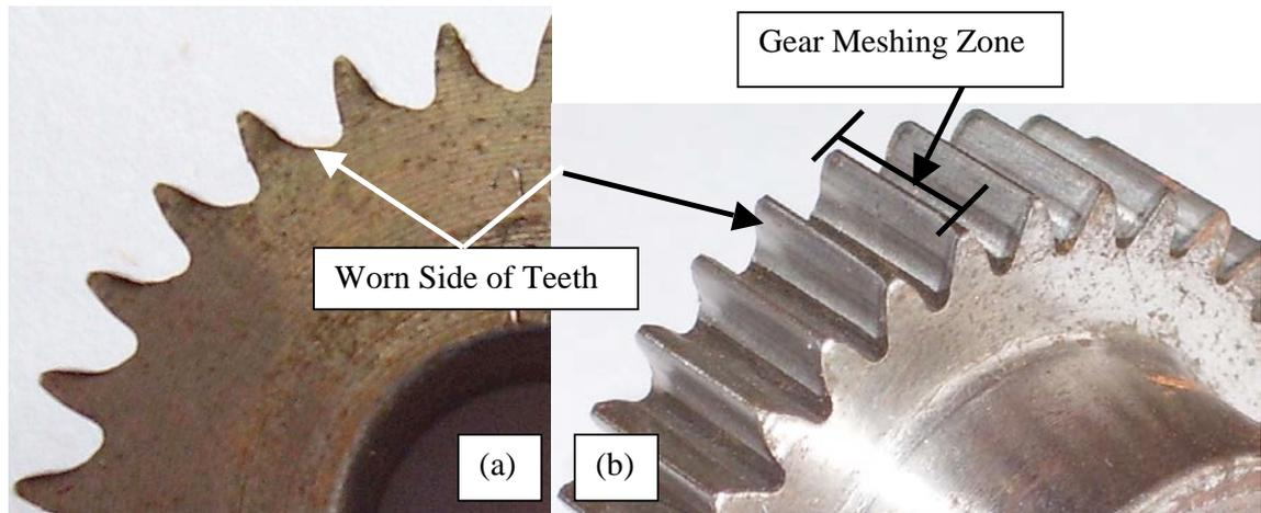
**Figure 8.6:** Gear tooth profiles — post test (a) end view, (b) original profile visible due to offset in gear mesh.
