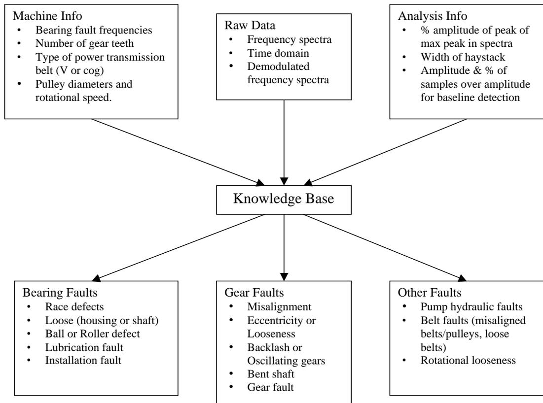
**Figure 5.2:** Flow chart of knowledge base inputs and outputs. Note: refer to Table 5.1 for a complete list of all detectable faults.
