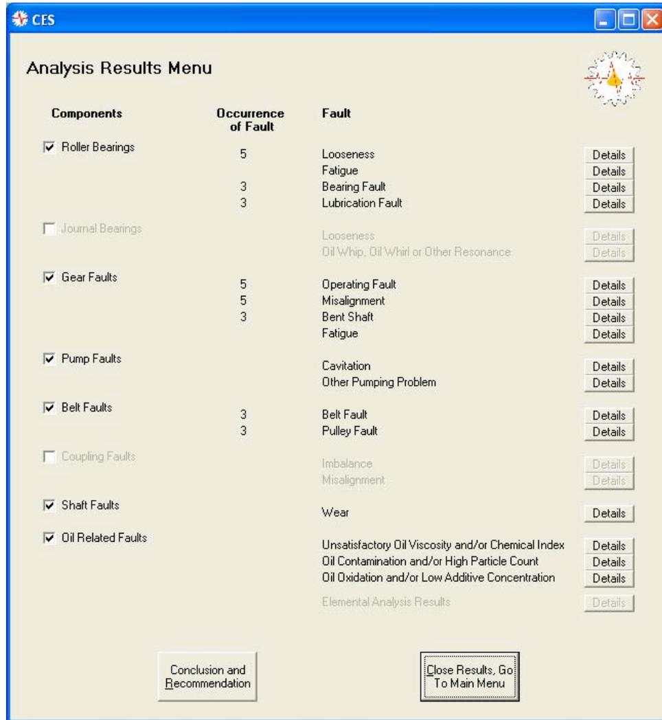
Figure H.11: The Analysis Results menu of the Combined Analysis Expert System.
