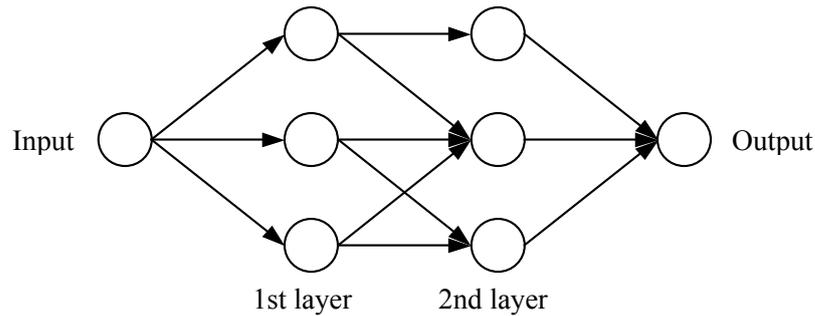
**Figure 2.30:** *Layout of a multilayer perceptron (2 layers shown).*
