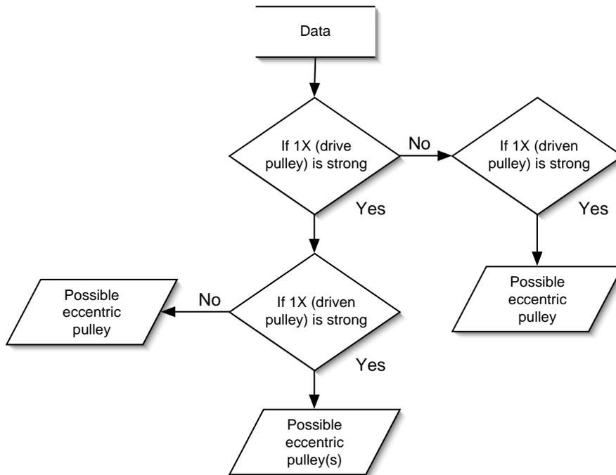
Figure C.20: Belts — Eccentric Pulley(s).
