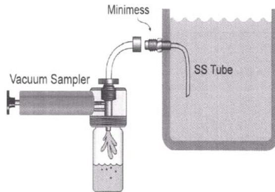
**Figure 2.6:** *Probe-on vacuum sampling [9].*
