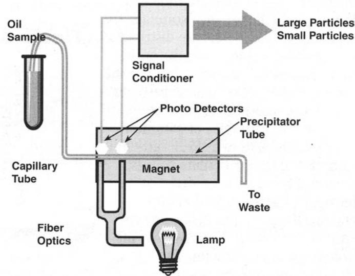
**Figure 2.11:** Operation of direct reading ferrograph [3].
