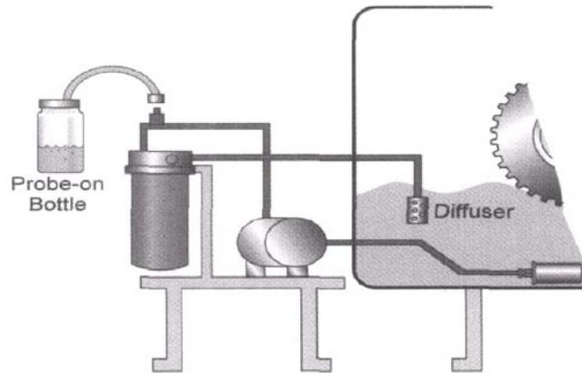
**Figure 2.4:** *Kidney loop oil filtration system [9].*
