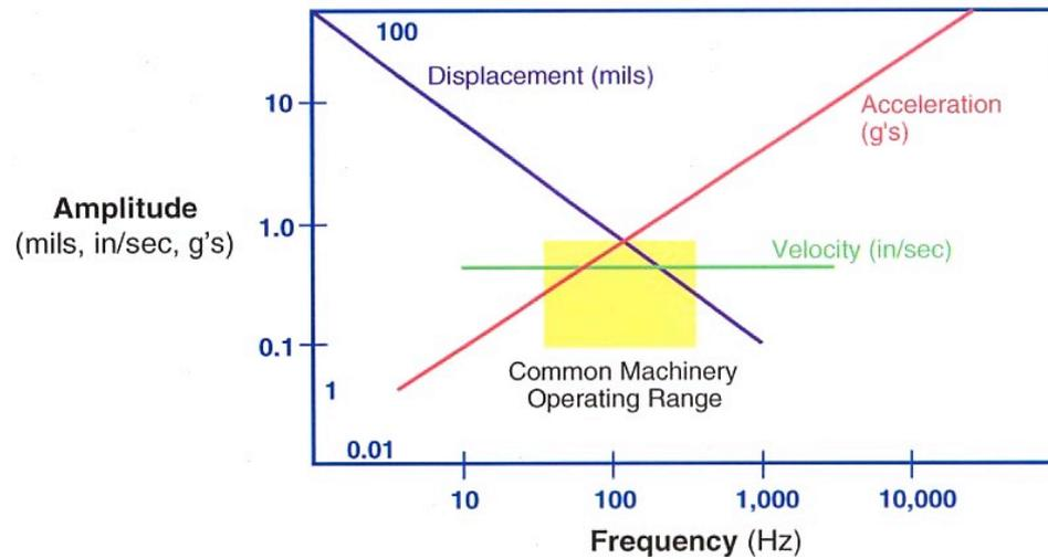
**Figure 2.27:** Frequency response of various vibration sensors [57].
