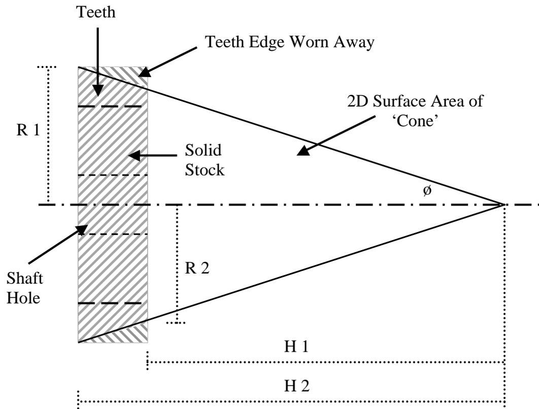
Figure 8.4: Calculation of gear volume wear using conical machining model.
