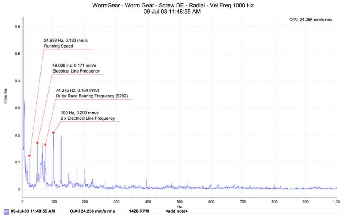
**Figure 4.17:** Velocity-frequency spectrum at the drive end of the worm gearbox for the contamination test.
