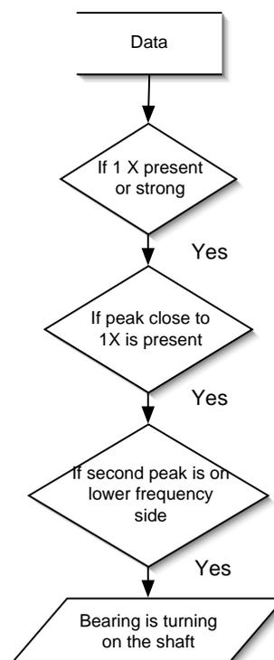
**Figure C.9:** *Rolling Element Bearing — Turning on Shaft.*
