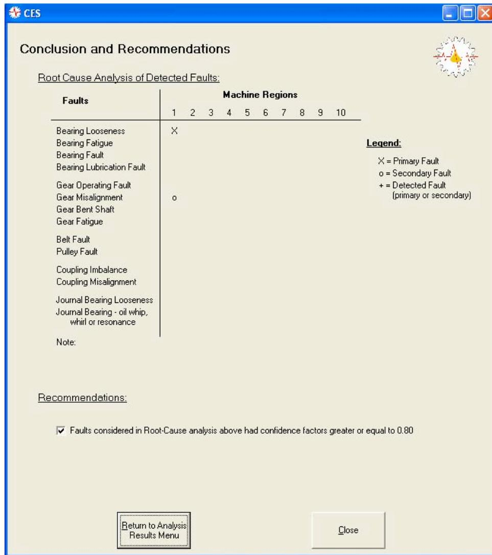
**Figure 7.8:** The Root-Cause Analysis results window, showing an example where bearing looseness caused gear misalignment.
