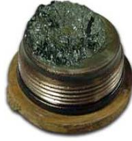
**Figure 2.10:** *Magnetic insert mounted on oil drain plug [14].*
