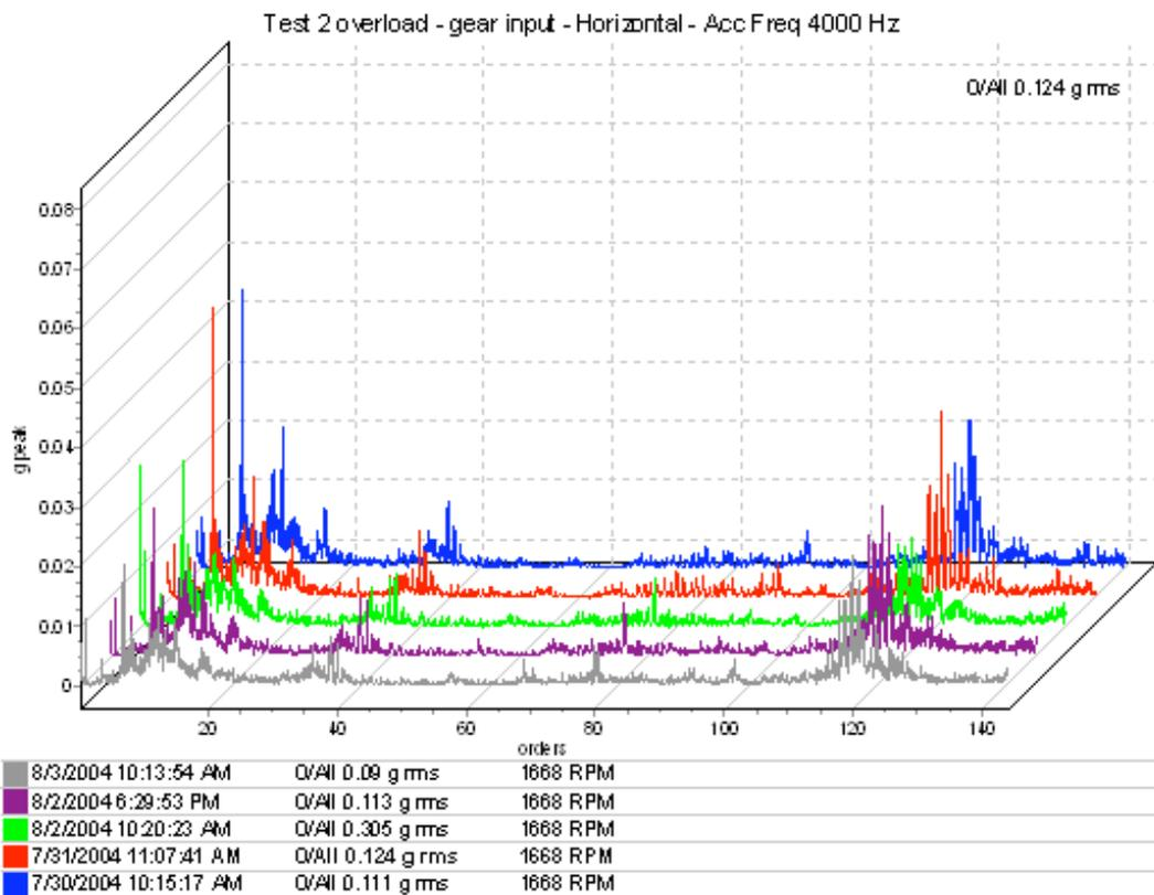
Figure 4.6: Trend of input gear frequency spectra (normalised to input gear speed).
