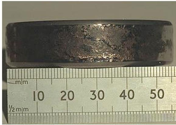
**Figure 2.21:** *Fretting corrosion of the outside surface of a bearing [50].*
