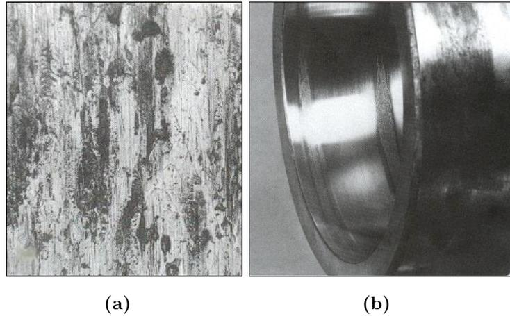
**Figure 2.22:** *Smearing on the surface of (a) a roller from a spherical roller bearing magnification 100x (b) the outer ring from a spherical roller bearing [50].*
