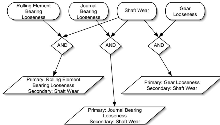
**Figure E.7:** Possible Causes for Shaft Wear.
