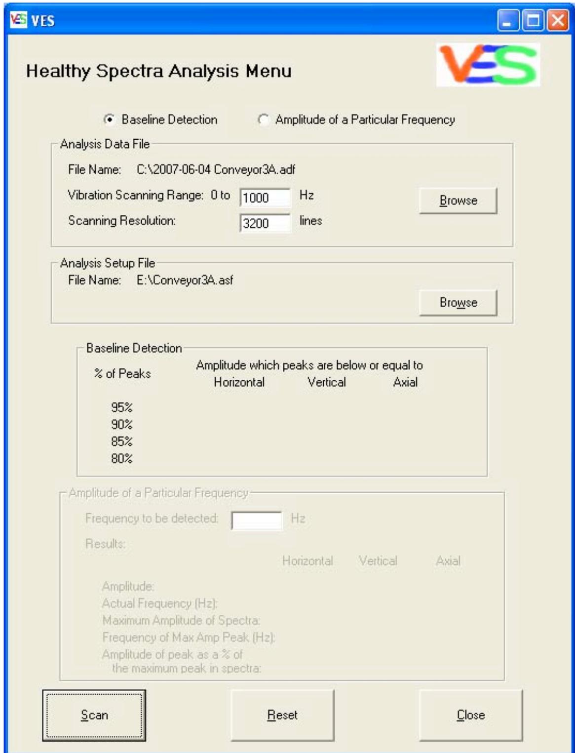
**Figure 5.10:** The VES Healthy Spectra Analysis menu. This menu allows (a) Amplitude detection of a particular frequency (selected in figure), (b) Baseline analysis.
