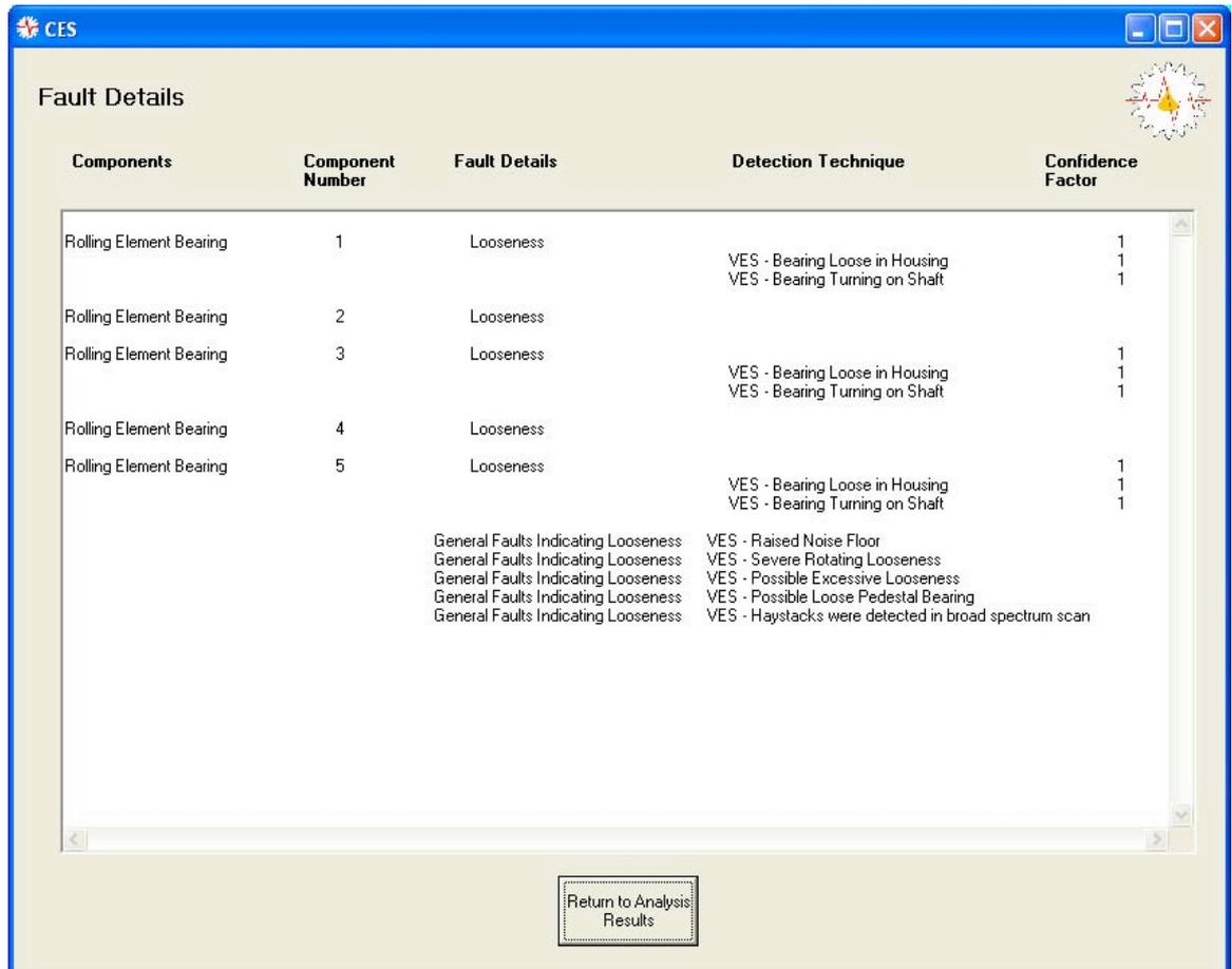
Figure H.12: The Analysis Results — Details menu of the Combined Analysis Expert System.
