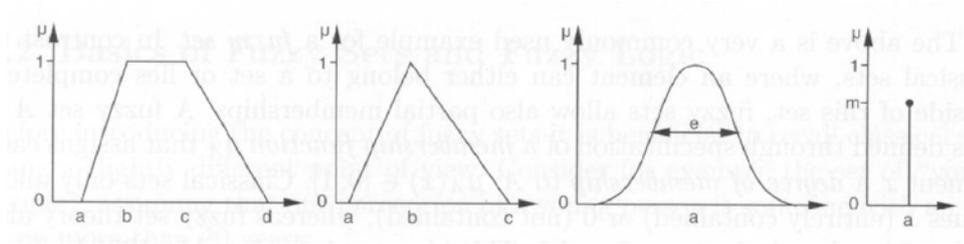
**Figure 2.31:** Graphs of common fuzzy set functions [90]. The functions are (left to right): Trapezoidal, Triangular, Gaussian and Singleton.
