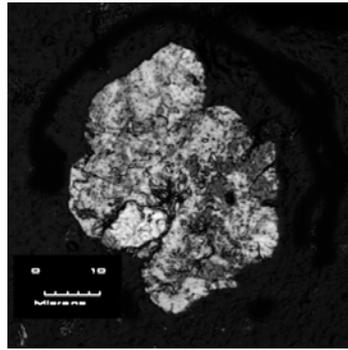
**Figure 4.4:** Laminar particle generated during the normal operation test.
