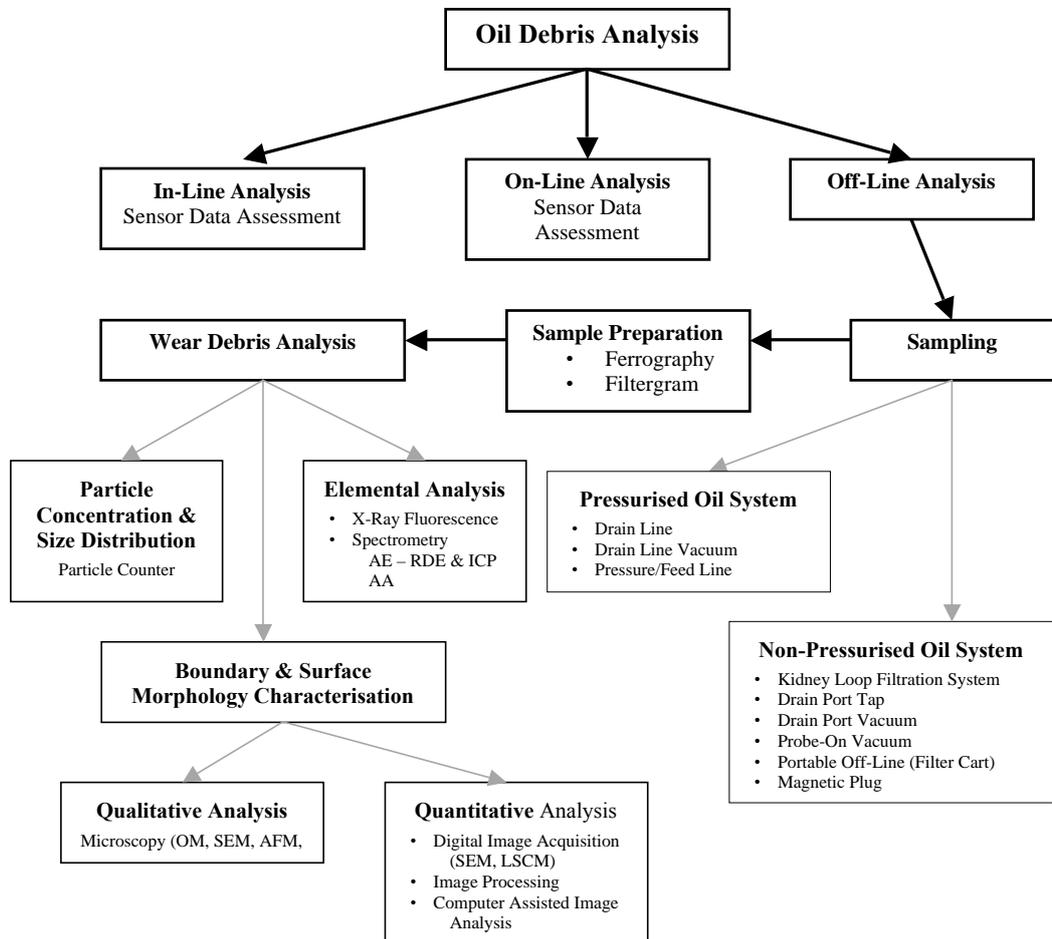
Figure 2.2: Flowchart of oil debris analysis.
