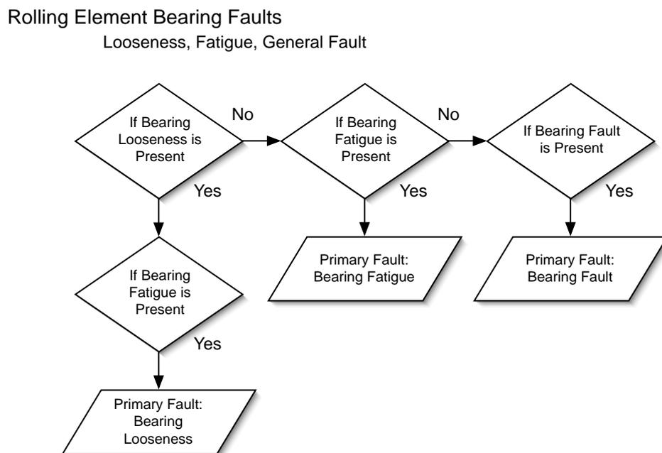
**Figure E.1:** *Rolling Element Bearing — Looseness, Fatigue and General Faults.*
