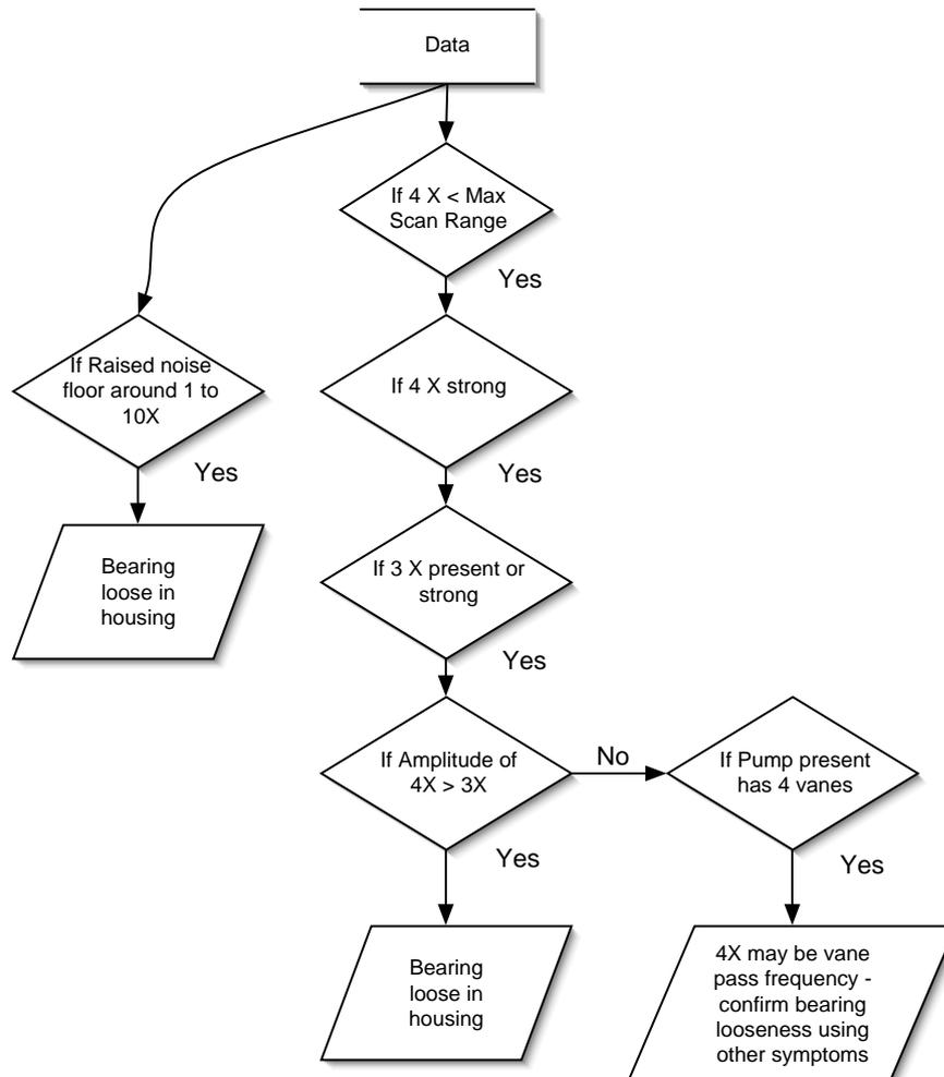
Figure C.8: Rolling Element Bearing — Loose in Housing.
