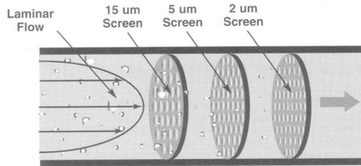
**Figure 2.14:** Operating principle of pore blockage particle counter, and typical screen sizes [3].
