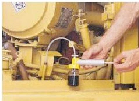
Figure 2.9: Drop tube vacuum sampling — sampling oil through dip-stick [3].
