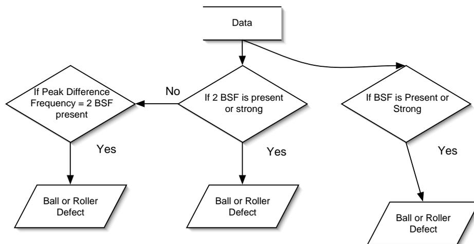
Figure C.4: Rolling Element Bearing — Ball or Roller Defect.
