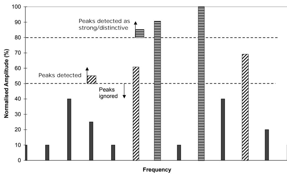
**Figure 5.6:** Normalised amplitude peak detection principle. The low and high normalised alarm threshold values are operator defined, and in this case set at 50 % and 80 % respectively.
