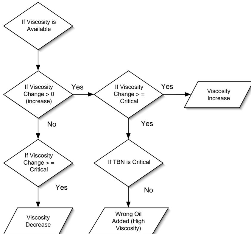
Figure D.16: *Viscosity Analysis.*
