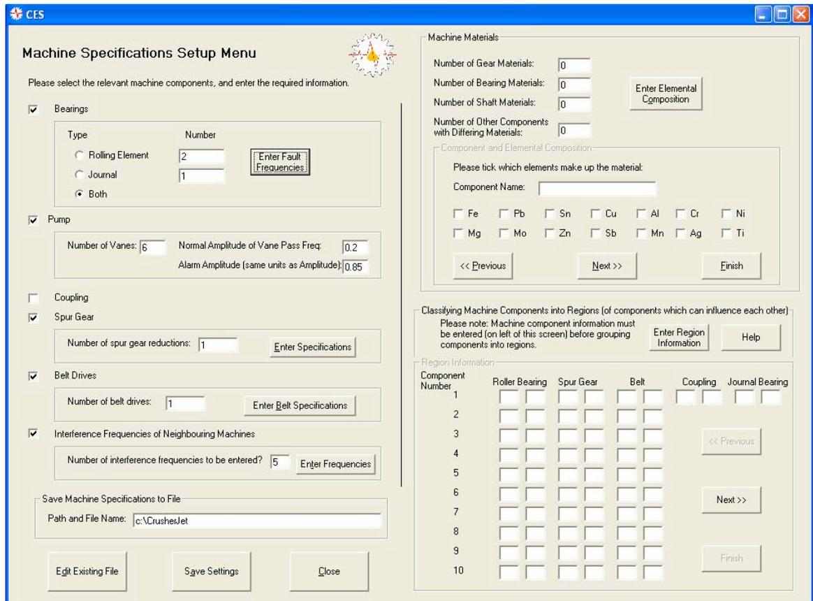
**Figure H.4:** The Machine Specifications Setup menu. The sub-menus for entering bearing fault frequencies, spur gear specifications, belt drive specifications, and interference frequencies, as well as the menu for additional fault frequencies are identical to those of the VES With Machine Historical Data case (Figures in Section H.4.2), except for differences in logo and application icon.
