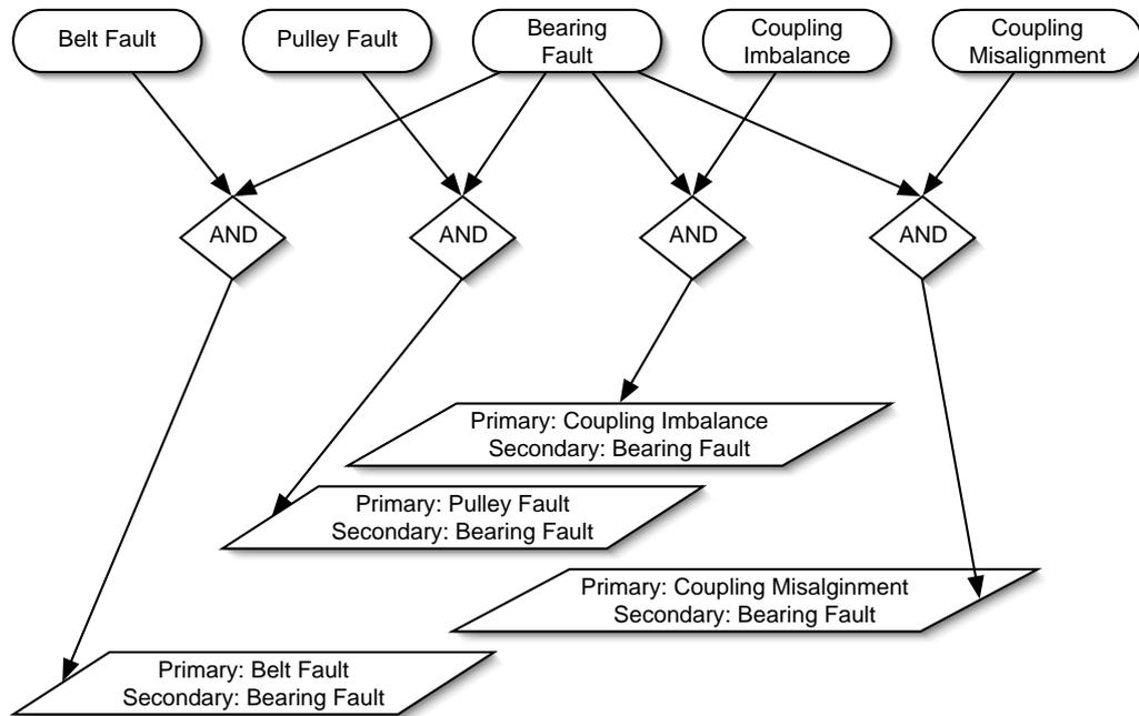
**Figure E.3:** *Rolling Element Bearing — Belt, Pulley or Coupling Related Fault.*
