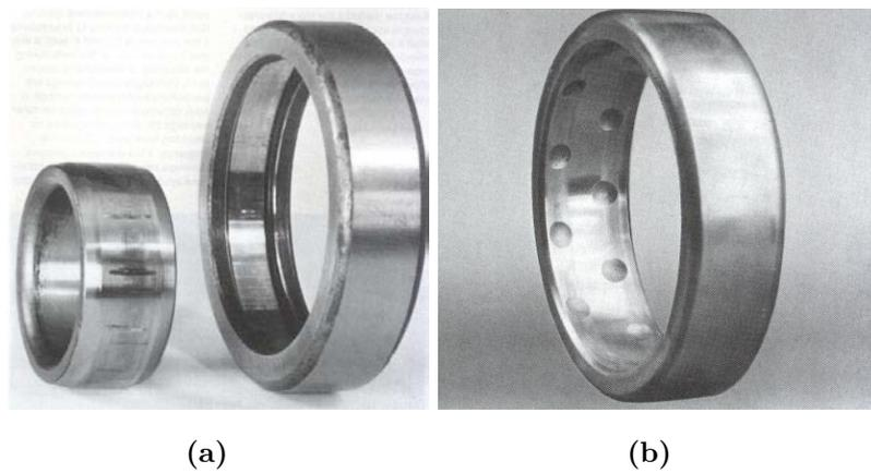
**Figure 2.25:** *Bearings damaged by external vibration (a) fluting of outer and inner ring of a spherical roller bearing (b) outer ring of a self aligning ball bearing showing spherical cavities [50].*
