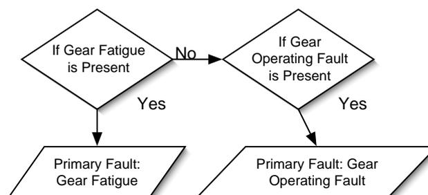
**Figure E.5:** *Spur Gears — Fatigue & Operating Fault.*
