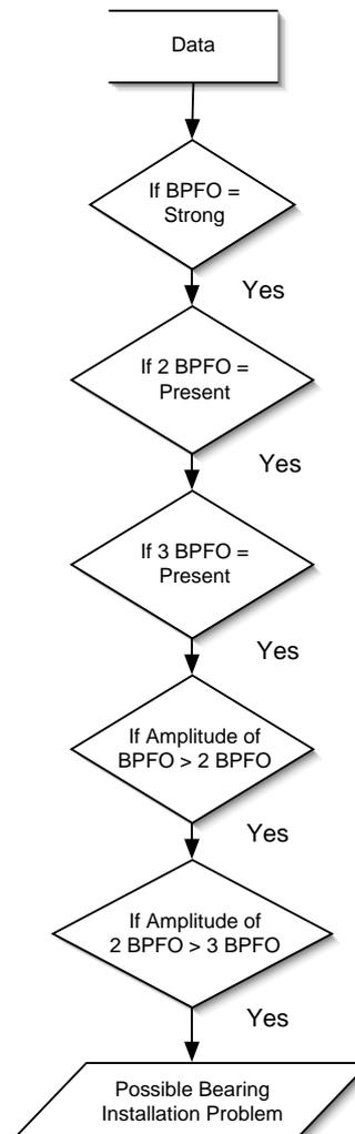
**Figure C.7:** *Rolling Element Bearing — Installation Fault.*
