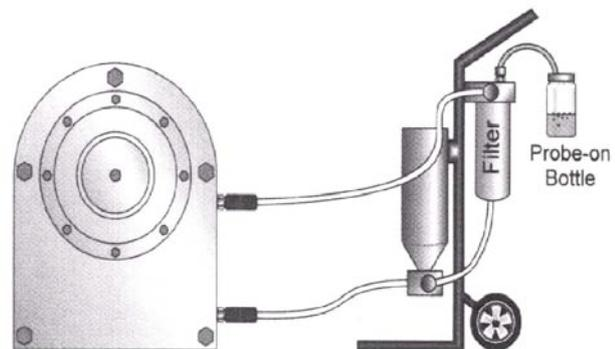
**Figure 2.7:** *Portable off-line sampling setup using portable filter cart [9].*
