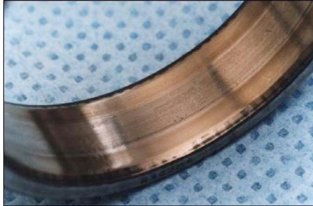
**Figure 2.24:** *Outer race of a spherical roller bearing worn by abrasive particles [50].*
