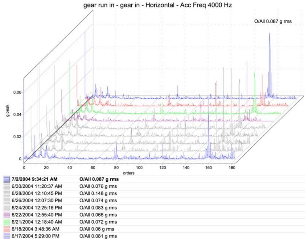
**Figure 4.15:** Waterfall plot of 4000 Hz acceleration at the input side of the gearbox, for the bent shaft test. The rotational speed of the input shaft was 1327 RPM, the 4000 Hz corresponding to 180.9 orders.
