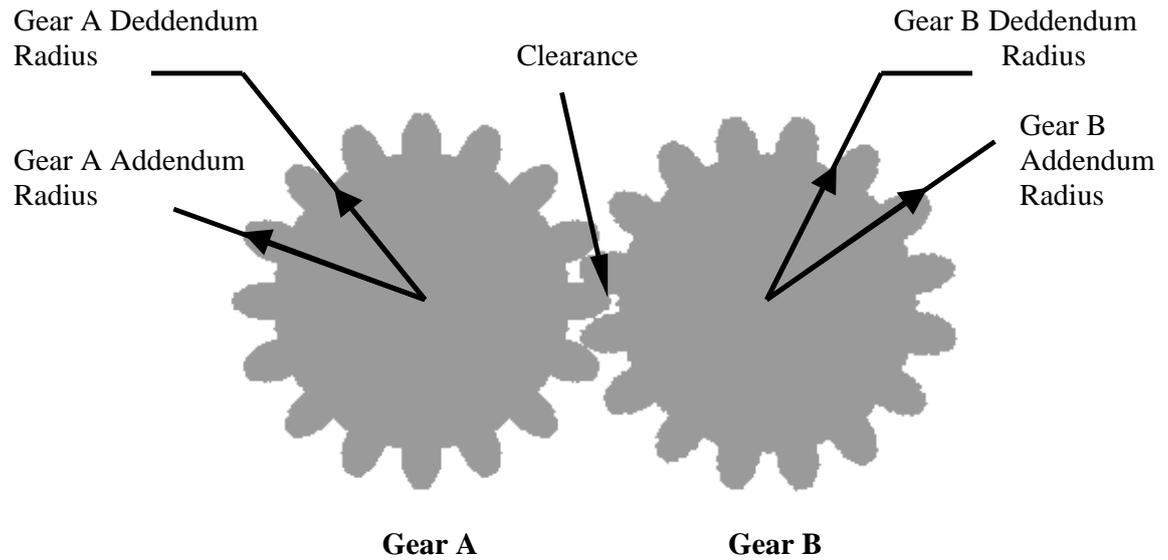
**Figure 8.3:** *Meshing of Gear Teeth within Addendum and Dedendum Radii of Each Gear.*
