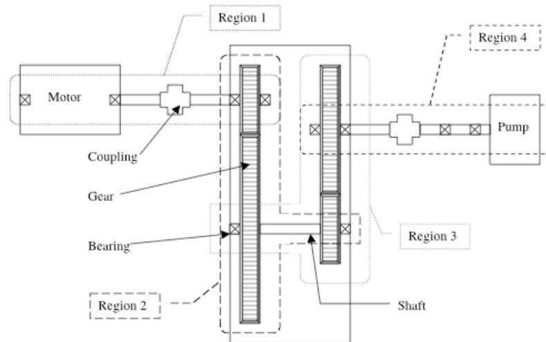
**Figure 7.5:** Schematic diagram of an electric motor, gearbox and pump arrangement, showing possible machine region boundaries.
