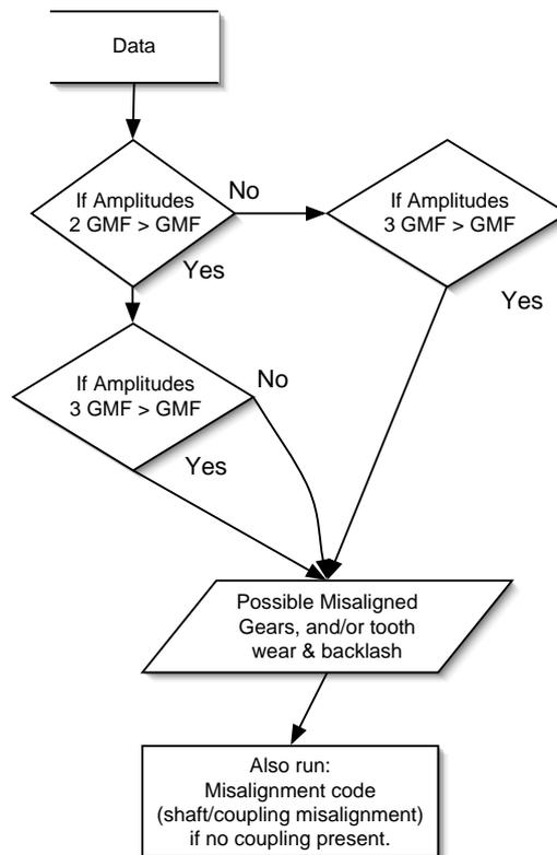
Figure C.13: *Spur Gears — Misalignment.*
