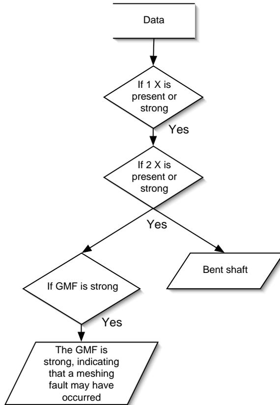
NOTE: this flow chart is run once for the input gear, and once for the output gear of each gear set.
