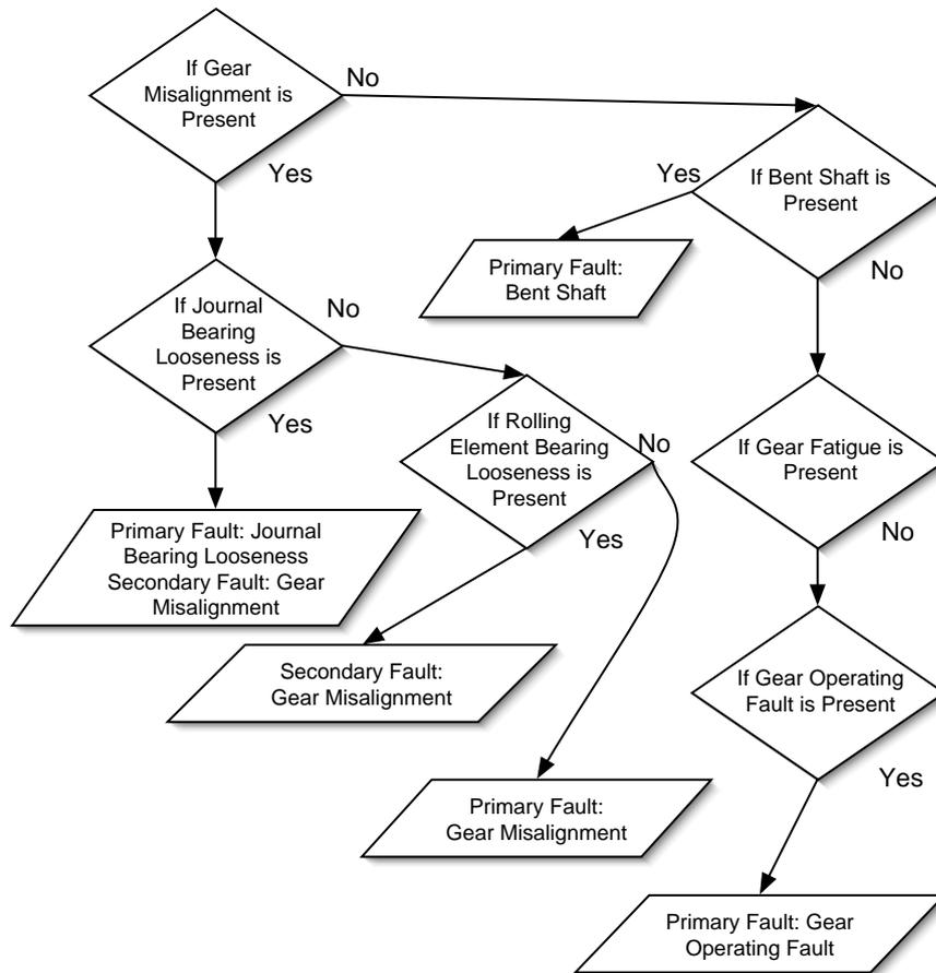
Figure E.6: Spur Gears — Fatigue, Misalignment & Operating Fault.
