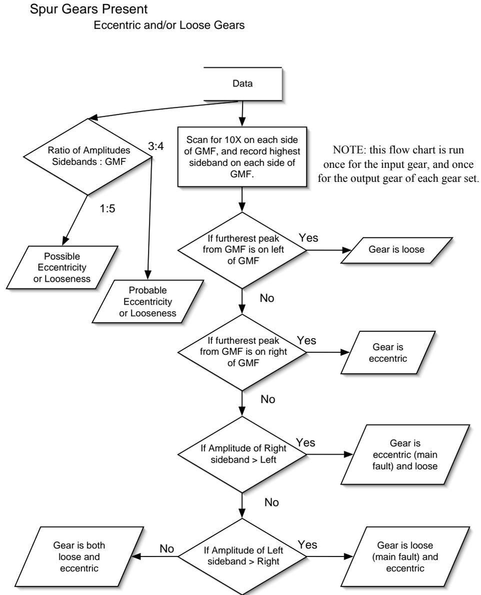
Figure C.12: *Spur Gears — Eccentricity & Looseness.*
