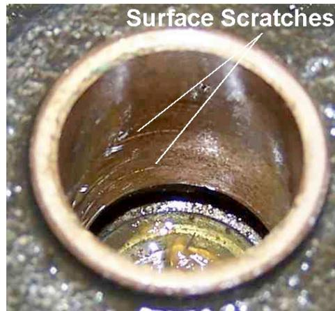
**Figure 5.14:** *Scratched surface of brass bush supporting intermediate drive shaft.*
