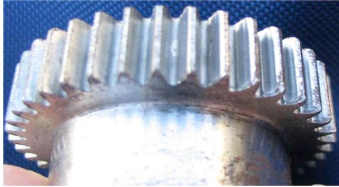
**Figure 4.14:** *Photo of one of the gears from the contamination test.*
