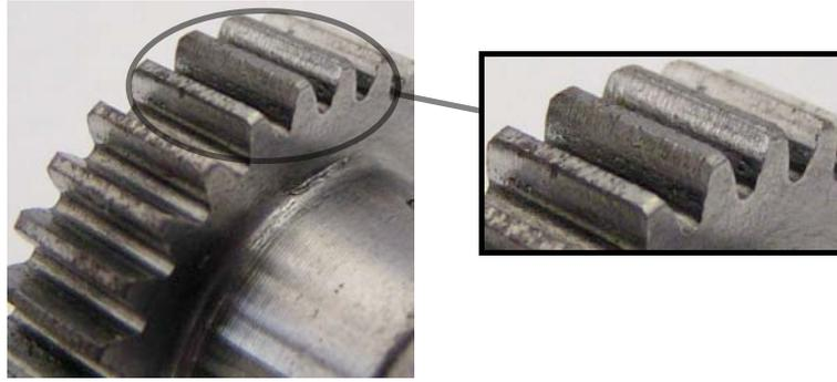
**Figure 4.12:** *Photo of gear teeth after cyclic load test.*
