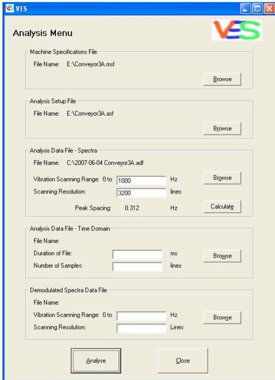
**Figure H.23:** The VES Analyse menu. The menu shown here looks identical for both analysis methods (With or Without Machine Historical Data), however the software code varies in the peak detection algorithm.
