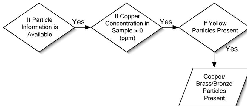
Figure D.15: Copper/Brass/Bronze Particles.
