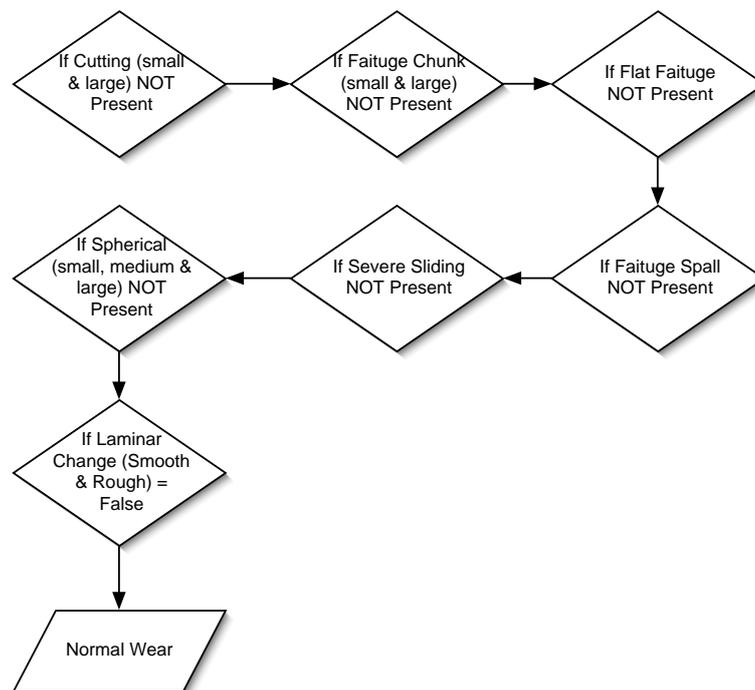
Figure D.1: *Normal Wear.*
