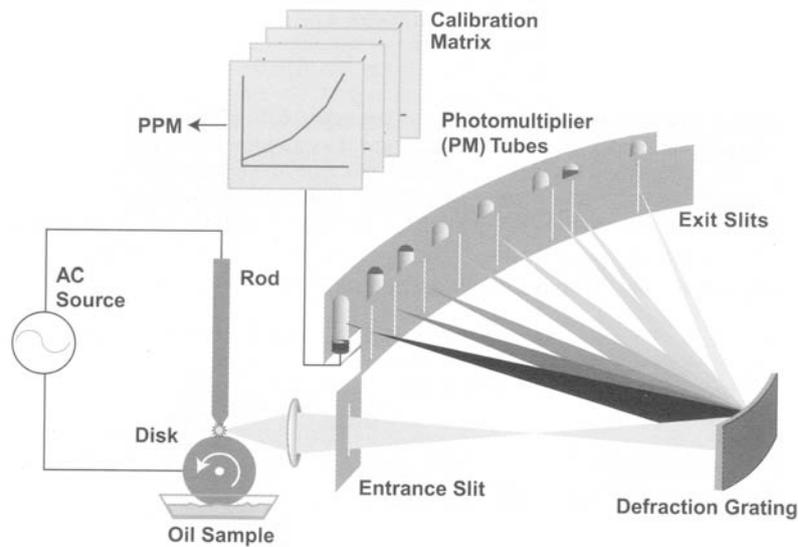
**Figure 2.16:** Operation of a rotary disk spectrometer [3].
