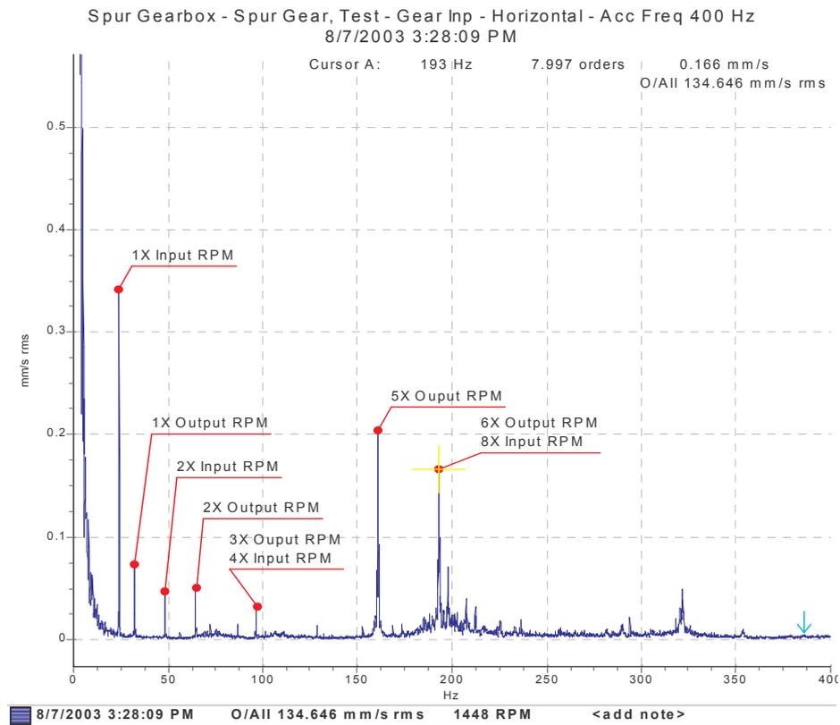
**Figure 4.2:** *Velocity-frequency spectrum at the input side of the gearbox.*
