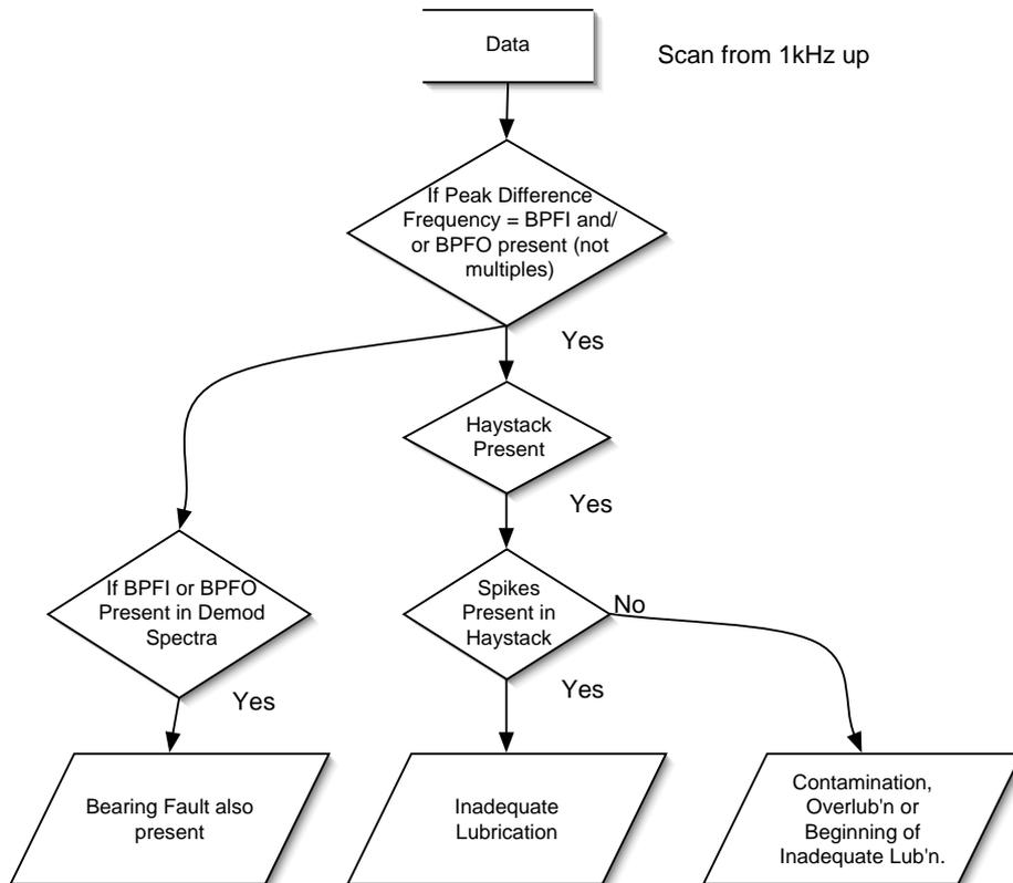
Figure C.6: Rolling Element Bearing — Inadequate Lubrication.
