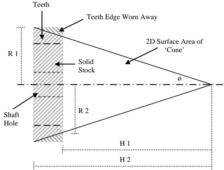
**Figure G.1:** Calculation of gear volume wear using conical machining model.
