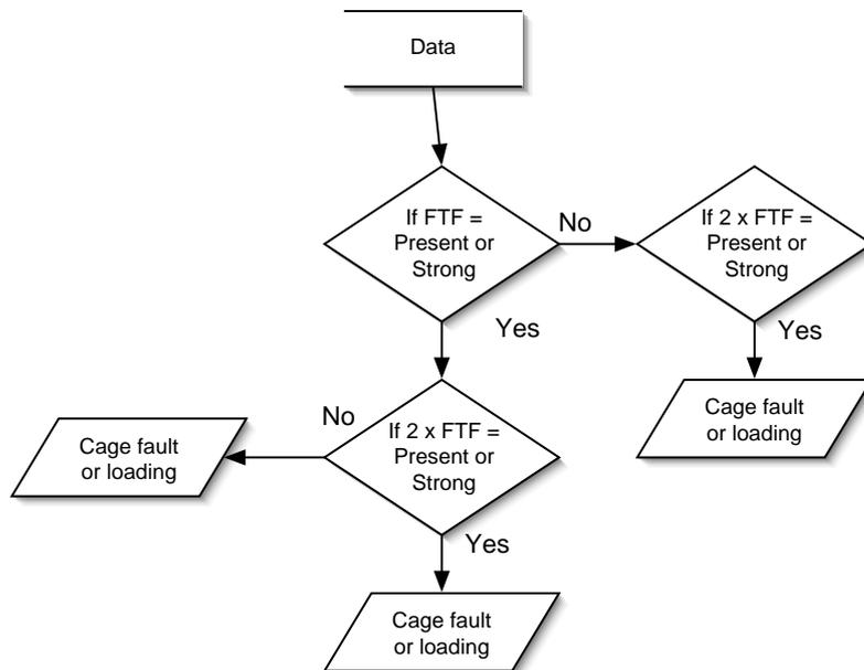
Figure C.3: Rolling Element Bearing — Cage Fault or Loading.
