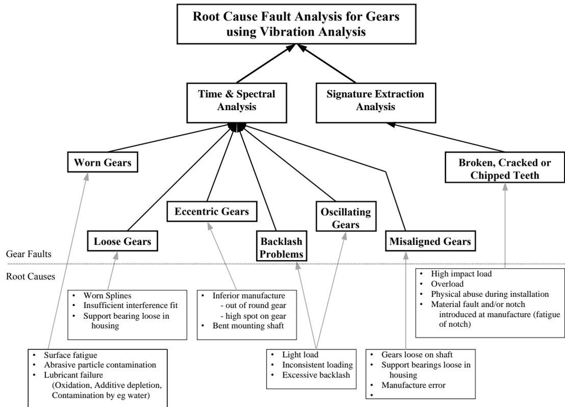
**Figure 2.28:** Flowchart of primary faults (root-causes), secondary faults, and detection technique.
