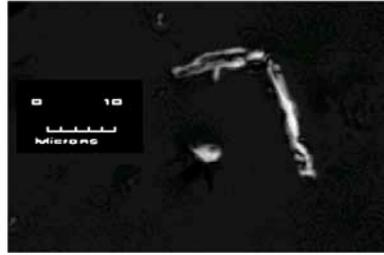
**Figure 4.8:** *Cutting wear particle generated during the constant overload test.*
