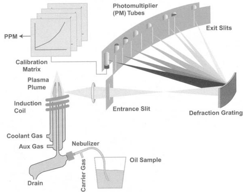
**Figure 2.17:** Operation of inductively coupled plasma spectrometer [3].
