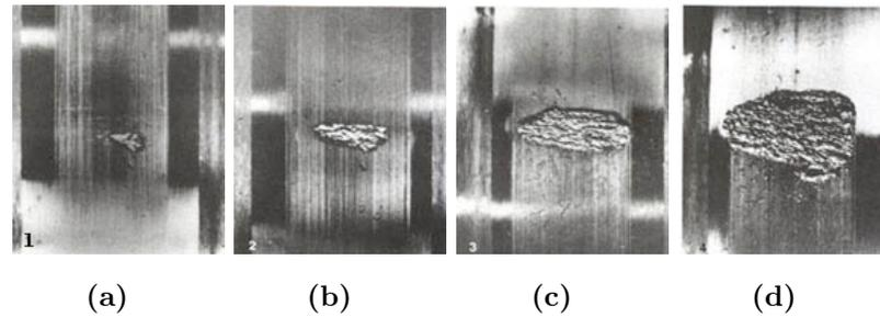
**Figure 2.19:** *The development of flaking — increased run time from (a) to (d) [50].*
