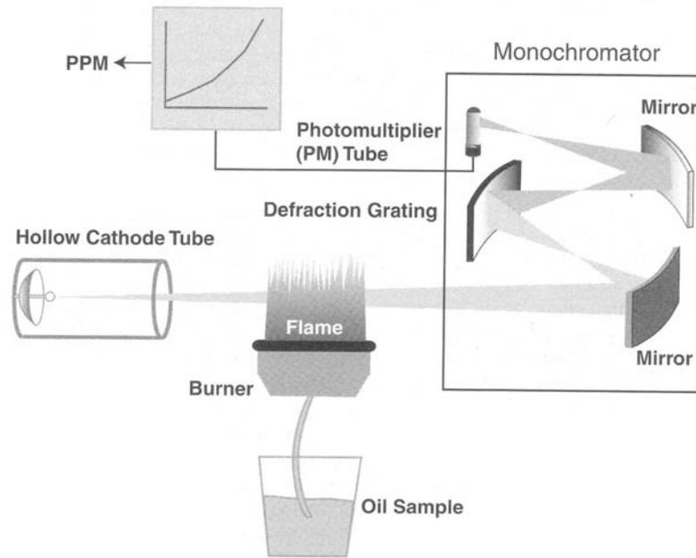
**Figure 2.18:** *Atomic absorption spectrometer [3].*
