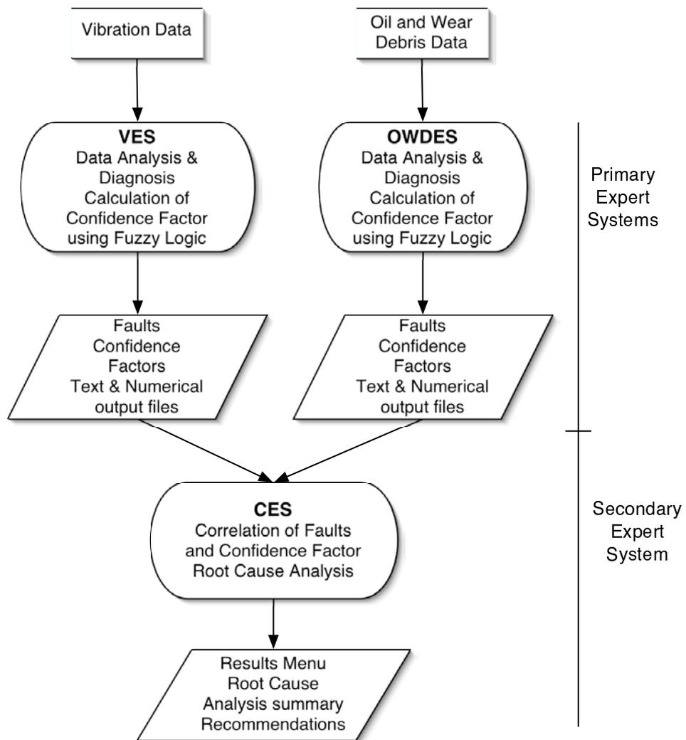
**Figure 7.1:** Data flow between the vibration, oil & wear debris, and combined analysis expert systems.
