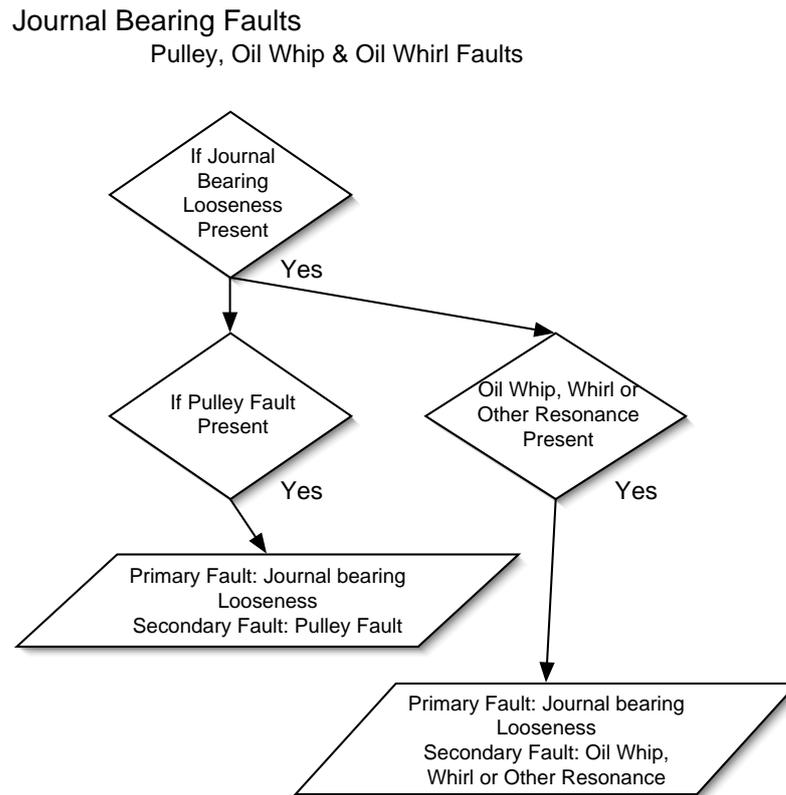
**Figure E.4:** *Journal Bearing — Pulley or Lubrication Fault.*
