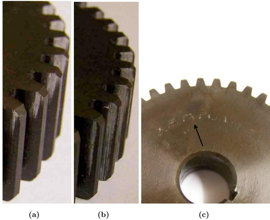
**Figure 5.13:** *Wear marks on the output gear of reduction 1. (a) wear on side of gear teeth, typical for misalignment, (b) wear extending across whole of width of gear teeth, (c) wear marks of neighbouring pinion gear, indicating looseness.*
