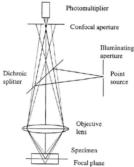
**Figure 2.15:** *Sketch of a laser scanning confocal microscope [34].*
