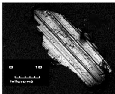
Figure 4.11: Sliding wear particle collected during the cyclic load test.
