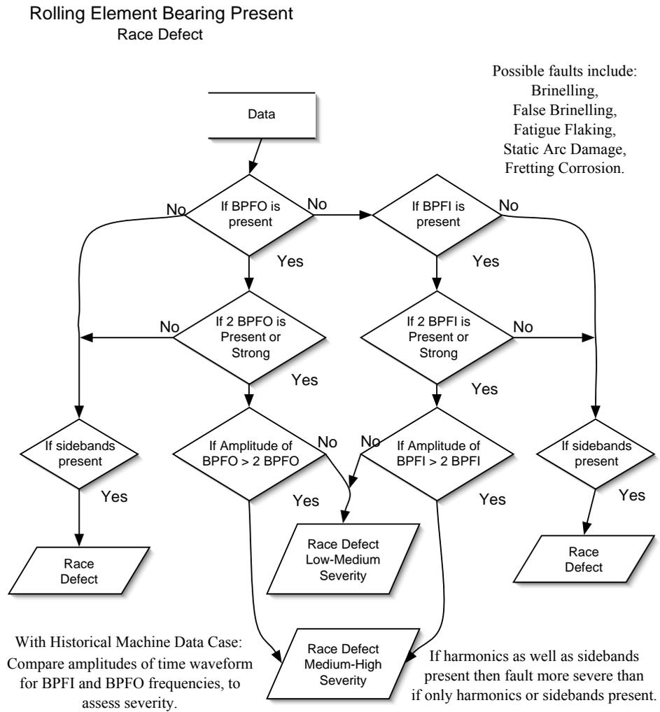
**Figure C.5:** *Rolling Element Bearing — Race Defect.*
