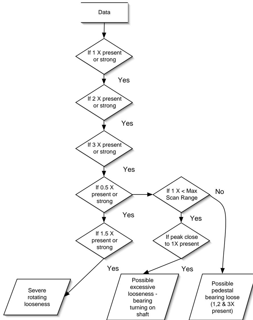
Figure C.10: Rolling Element Bearing — Rotating Looseness.
