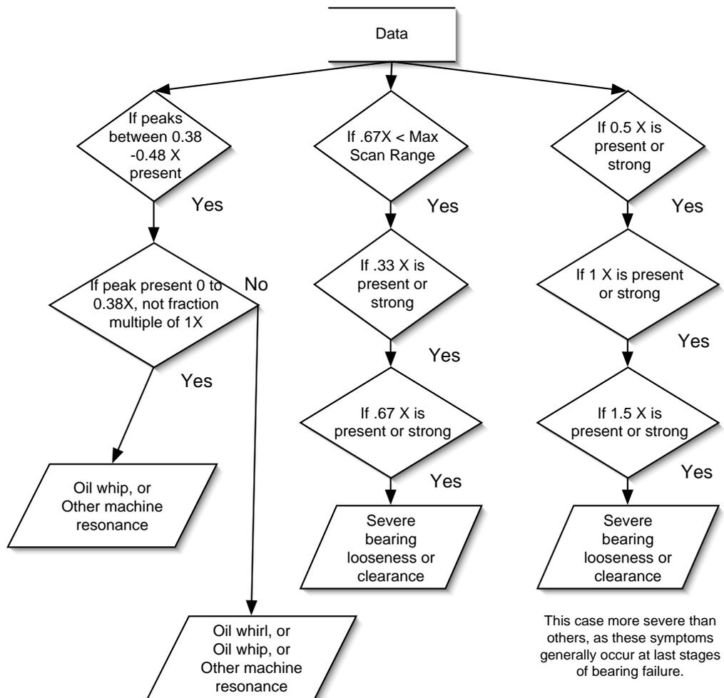
Figure C.11: Journal Bearing — Rotating Looseness and Lubricating Fault.
