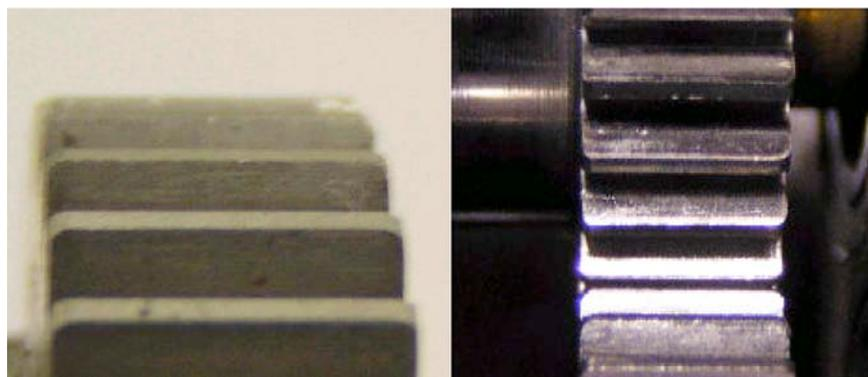
**Figure 4.5:** Gear tooth surfaces before (left) and after (right) the normal operation test.
