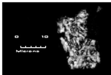
Figure 4.7: Fatigue particle generated during the constant overload test.
