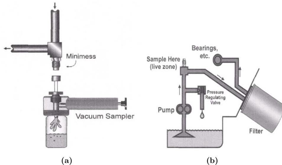
**Figure 2.3:** Sampling positions (a) Drain-Line Vacuum Sampling (b) Pressure or Feed Line Sampling [9].
