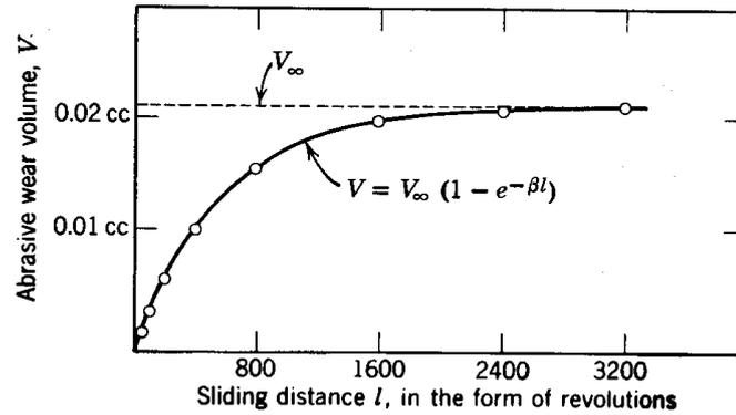
Figure 8.2: Abraded wear volume as a function of sliding distance [117].
