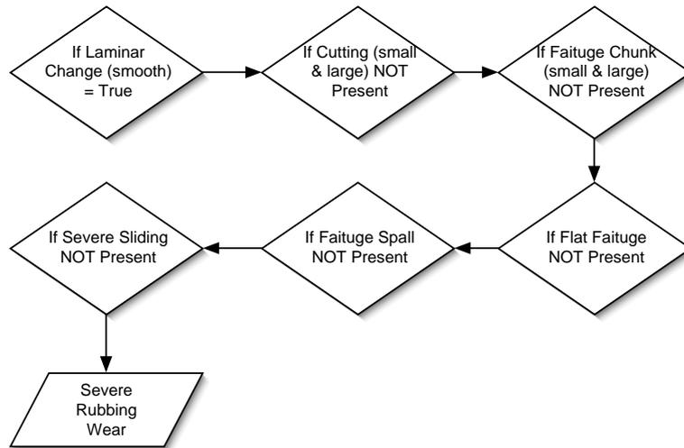
Figure D.2: Severe Rubbing Wear.
