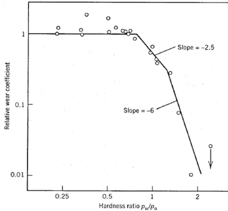
**Figure 8.1:** Variation of relative wear coefficient vs hardness ratio [117].
