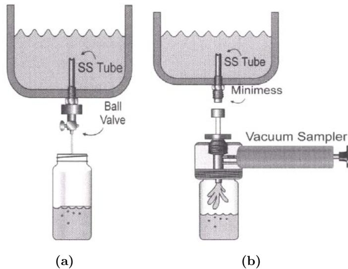
**Figure 2.5:** *Drain Port (a) Tap Sampling, (b) Vacuum Sampling [9].*
