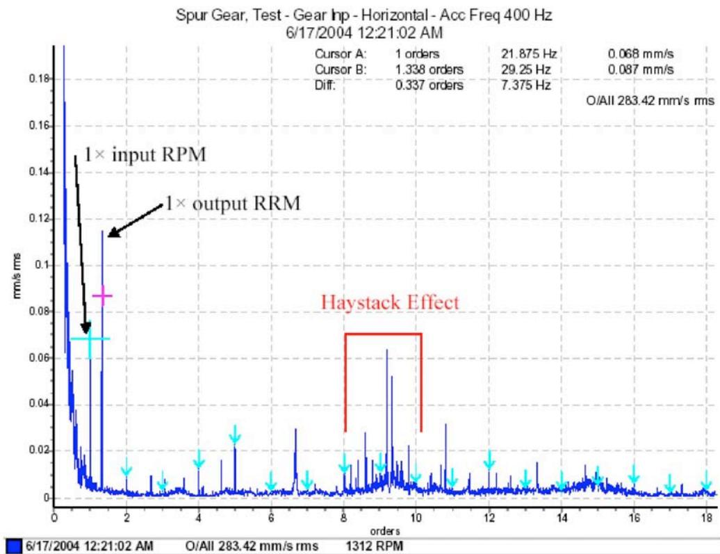
**Figure 4.16:** Frequency spectra of input gear (frequency normalised for speed of input gear) for bent input shaft test.
