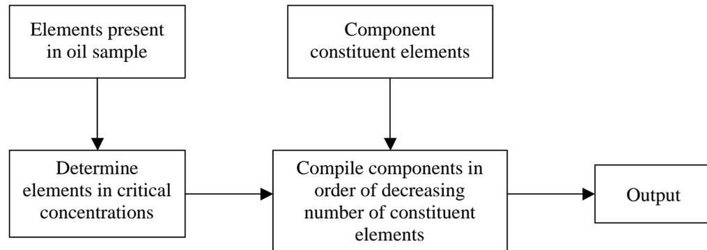
**Figure 6.4:** Operation of elemental analysis algorithm.
