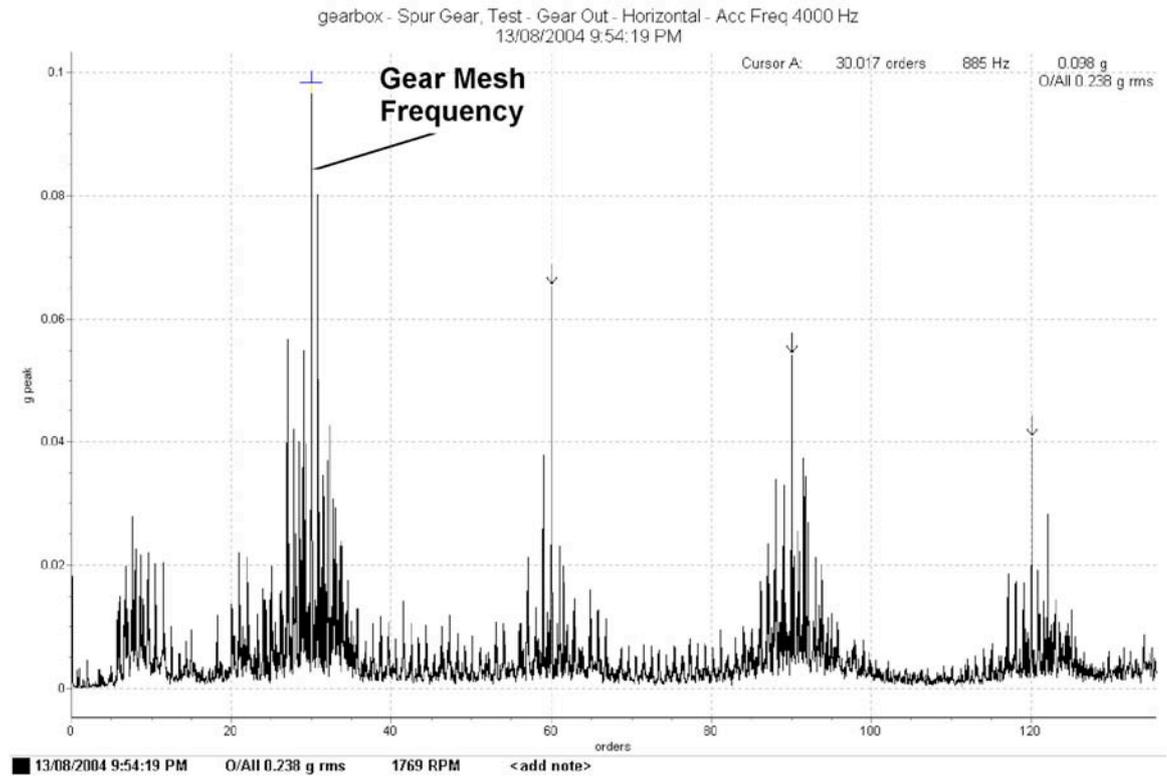
**Figure 5.12:** 4000 Hz horizontal acceleration spectra of the contamination test.
