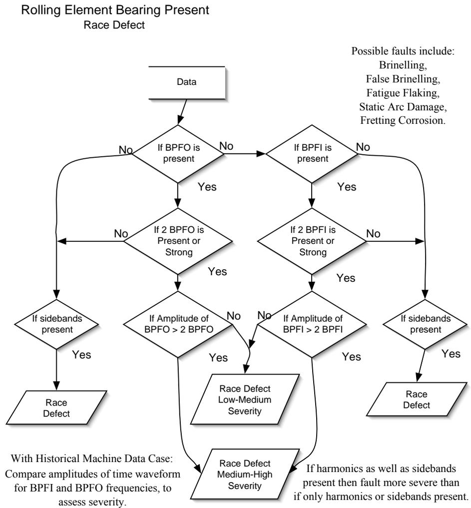
**Figure 5.3:** Knowledge base flow chart for bearing race defect diagnosis.
