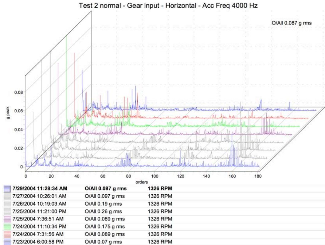
**Figure 4.3:** Waterfall plot of 4000 Hz acceleration at the input side of the gearbox.
