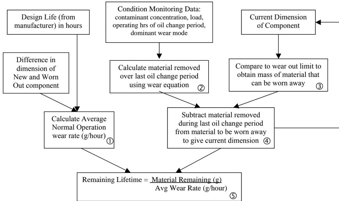
**Figure 8.5:** Calculations required to determine machine remaining lifetime.
