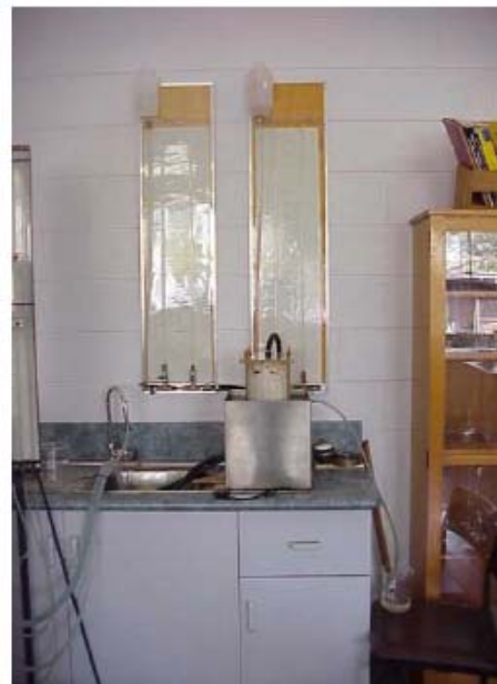
Fig 2.11. Falling head permeameter (a) Schematic diagram, (b) Actual permeameter set-up
