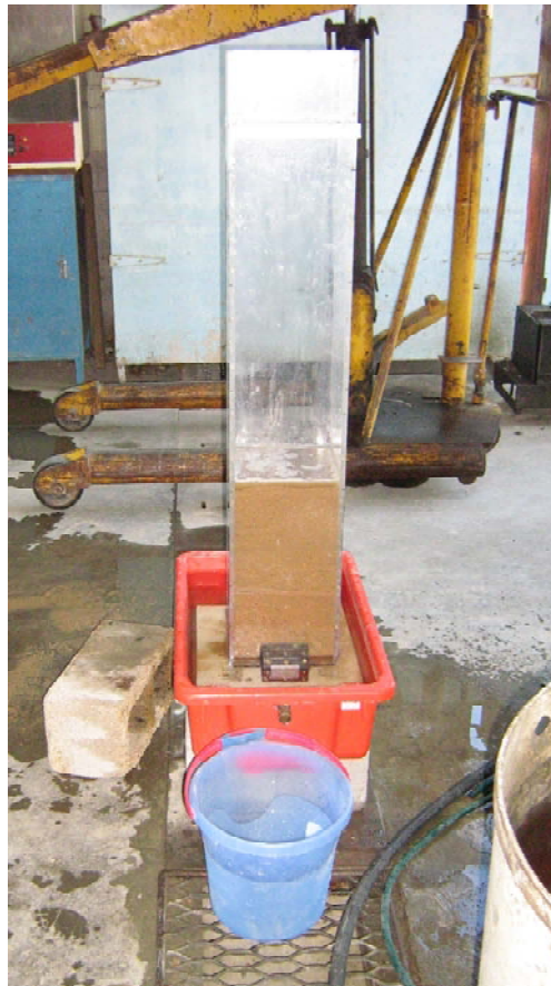
Fig. 4.20. Laboratory model stope setup
