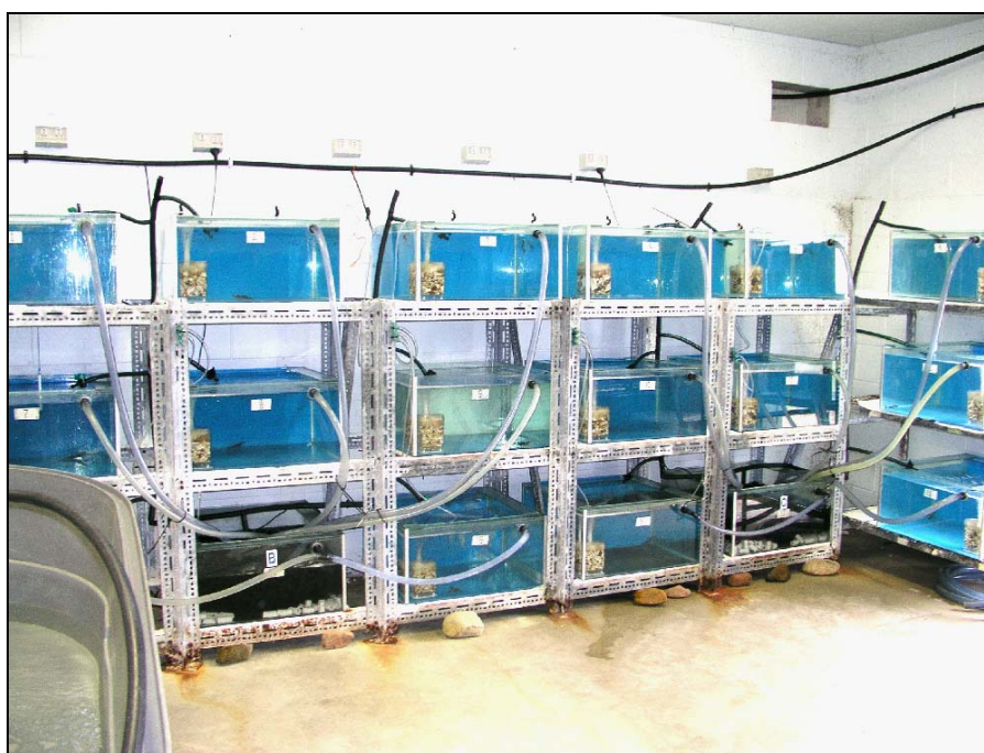
Figure 3.1. Experimental P. monodon were kept individually in recirculation aquaria to determine their moult stages. There were two modules which consisted of 8 aquaria and 1 recirculation tank with filter and each aquarium had an air lift corner filter. Salinity was maintained at 35 ‰ and temperature around 28 – 30 °C.
