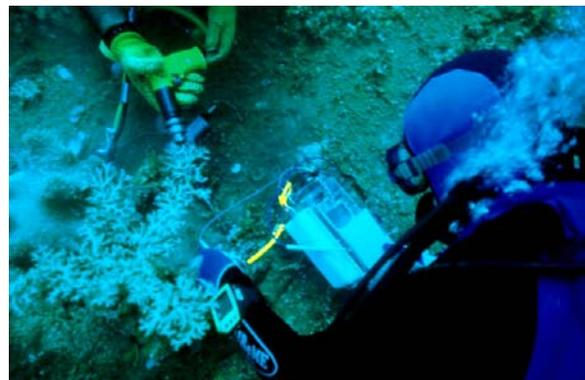
*Figure 8.61: The sealed box containing the meters and showing the drill used to penetrate the concretion and corrosion product (Photograph by Bill Jeffery, 2002).*
