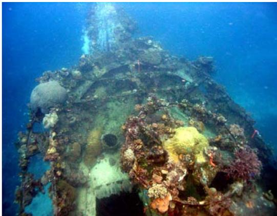
*Figure 8.14: The bow showing the bowsprit, deck sponsons on the port side and the circular structure on 'Unknown G' site (Photograph by Bill Jeffery, 2006).*
