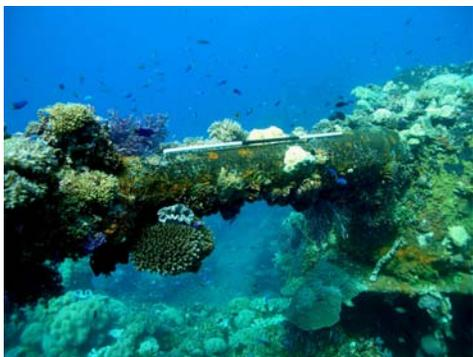
Figure 8.54: Coral loss and renewed corrosion from dynamite fishing on Fujikawa Maru bow gun. Scale 50 cm divisions (Photograph by Bill Jeffery, 2006).
