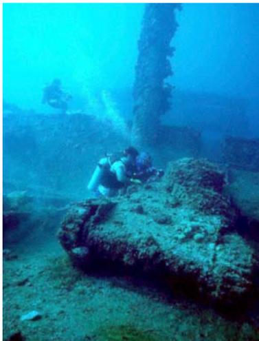
*Figure 8.60: Taking corrosion measurements on the tank on the deck of Nippo Maru (Photograph by Bill Jeffery, 2002).*
