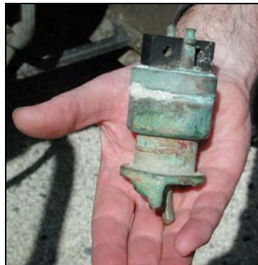
Figure C-6. 56: Electrical contact mine detonation mechanism (Peter Ferrier Collection).
