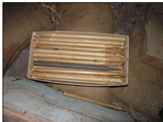
Figure C-6. 32: Unused searchlight carbon arc rods (FQ Collection).
