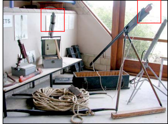
Figure 7. 41: Lifesaving rocket launchers display. Note rockets projectile in barrels tubes (QMM Collection).
