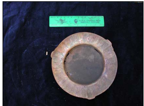
Figure 5. 18: Underside view of 80 pr gas check plate (Peter Ferrier Collection).
