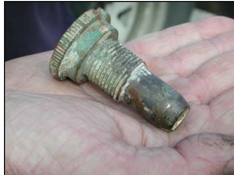
Figure 5.20: Shrapnel round percussion fuse (Peter Ferrier Collection).
