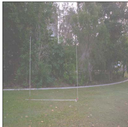
Figure 4.9. Quarter-wavelength whip antenna
