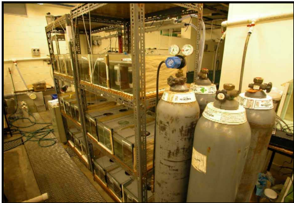
Figure 2.3 Photo of experimental set up in the aquarium room taken from front of tanks, and showing nitrogen gas cylinders with regulator attached to the cylinder in use. PVC lids on each aquarium have access holes, and are depressed about 2 cm below the rim of the aquaria.
