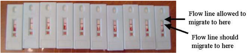
Figure 1-7 Clearance of blood after 60 minutes after allowing liquid front to migrate to end of test strip
