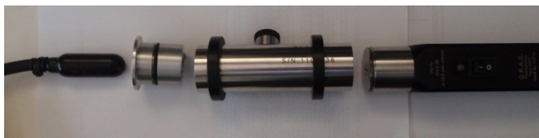
Figure 2.1. G.R.A.S. Pistonphone with HTI-96 hydrophone and adaptor
