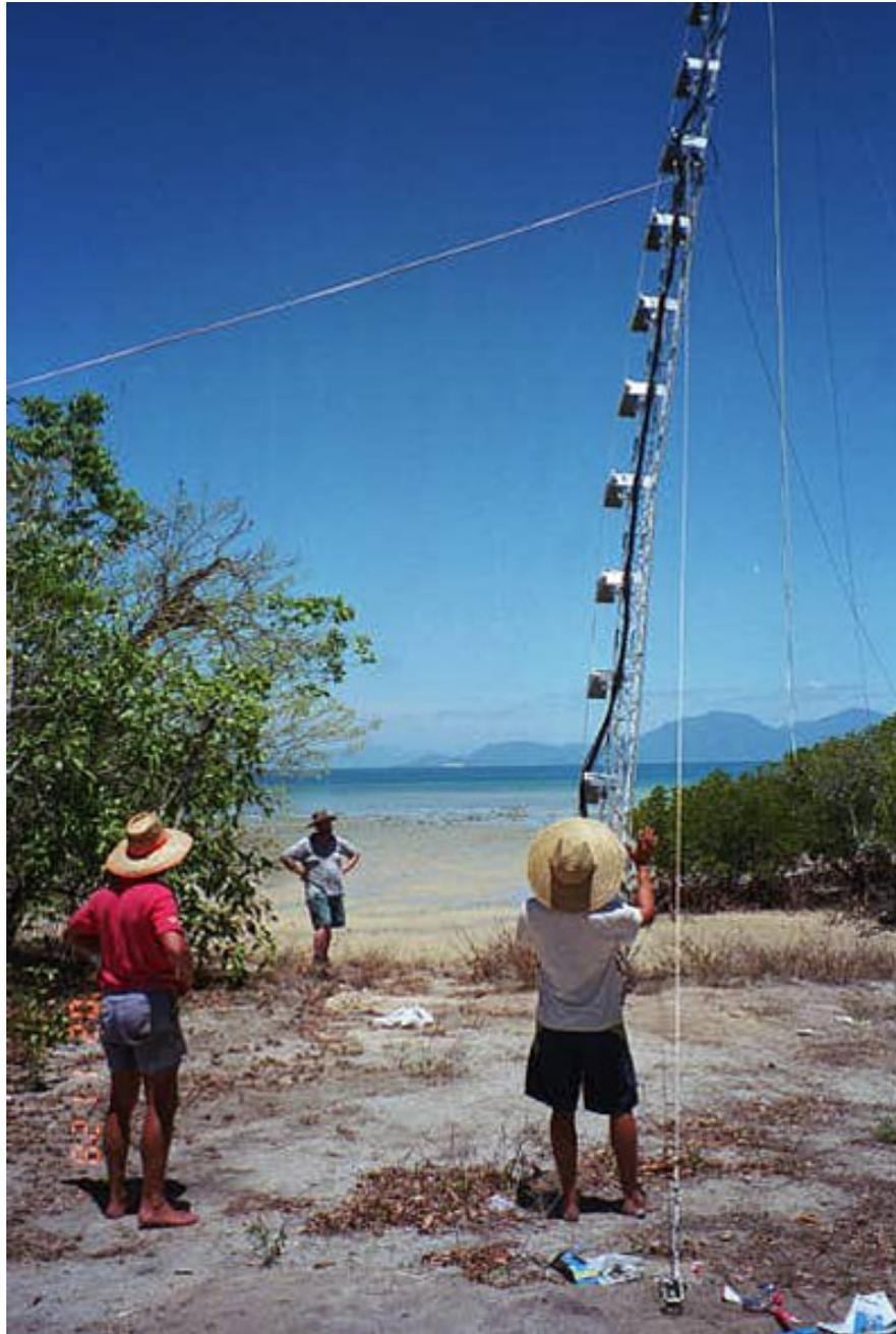
**Figure 9.10:** Raising the array by hand. The white building at the centre of the photo is the end of the jetty 18.6 km distant.
