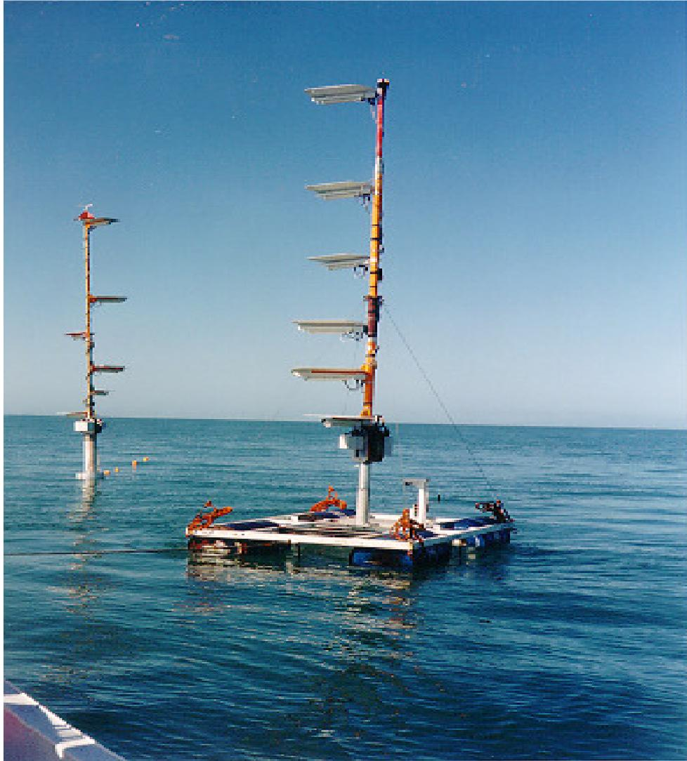
**Figure 5.11:** Buoys used to take measurements. Spar-buoy in back.
