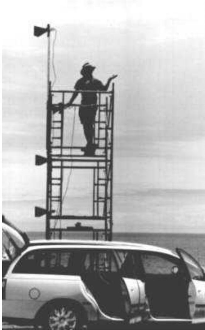
**Figure 9.2:** Ten element array using horns and rigid structure.
