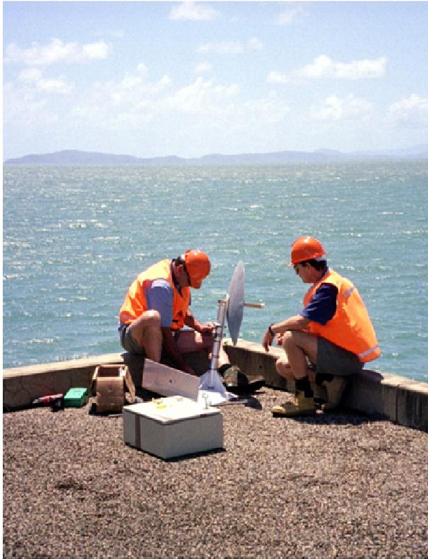
**Figure 9.8:** Transmitter showing penny feed.
