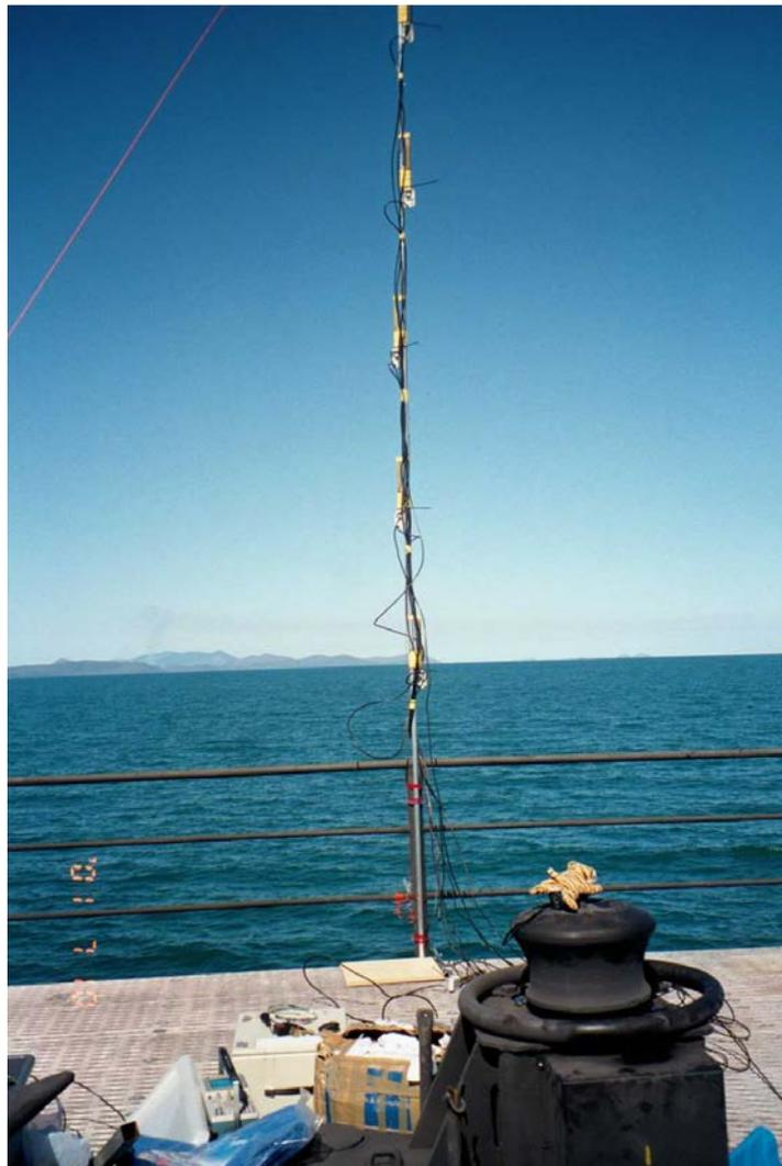
**Figure 9.1:** Ten element array using slotted guides and guyed pole.
