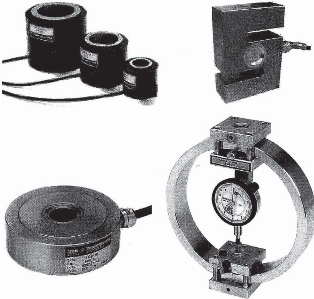
Figure A.6 Load cells and proving ring (Photograph: N. Sivakugan)
