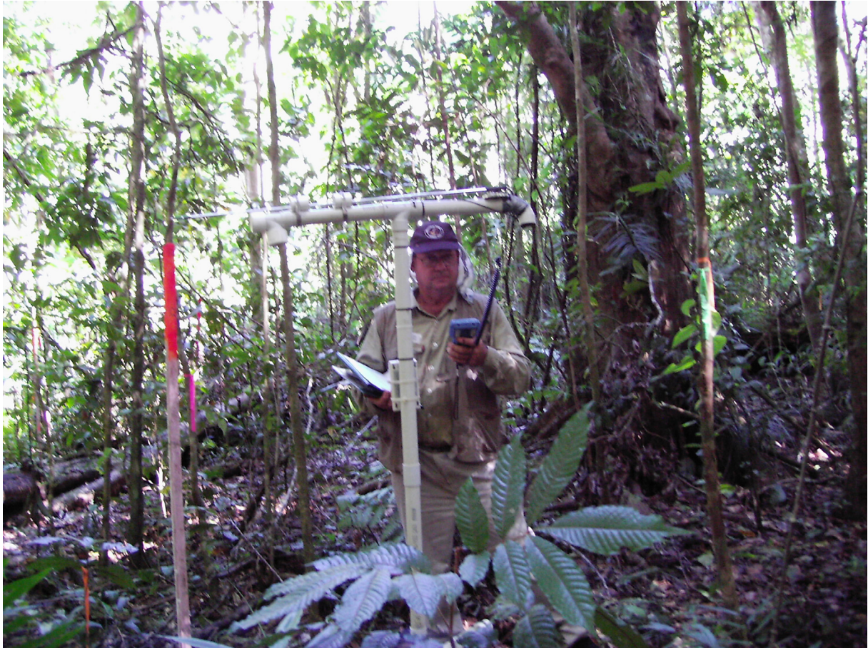
Figure 3: The instruments used for the traverse microclimate measurements were supported on a PVC frame. The quantum sensor was attached to the top of the frame (on a levelling mount). The person pictured is Stephen Pohlman. Photo by Catherine Pohlman.
