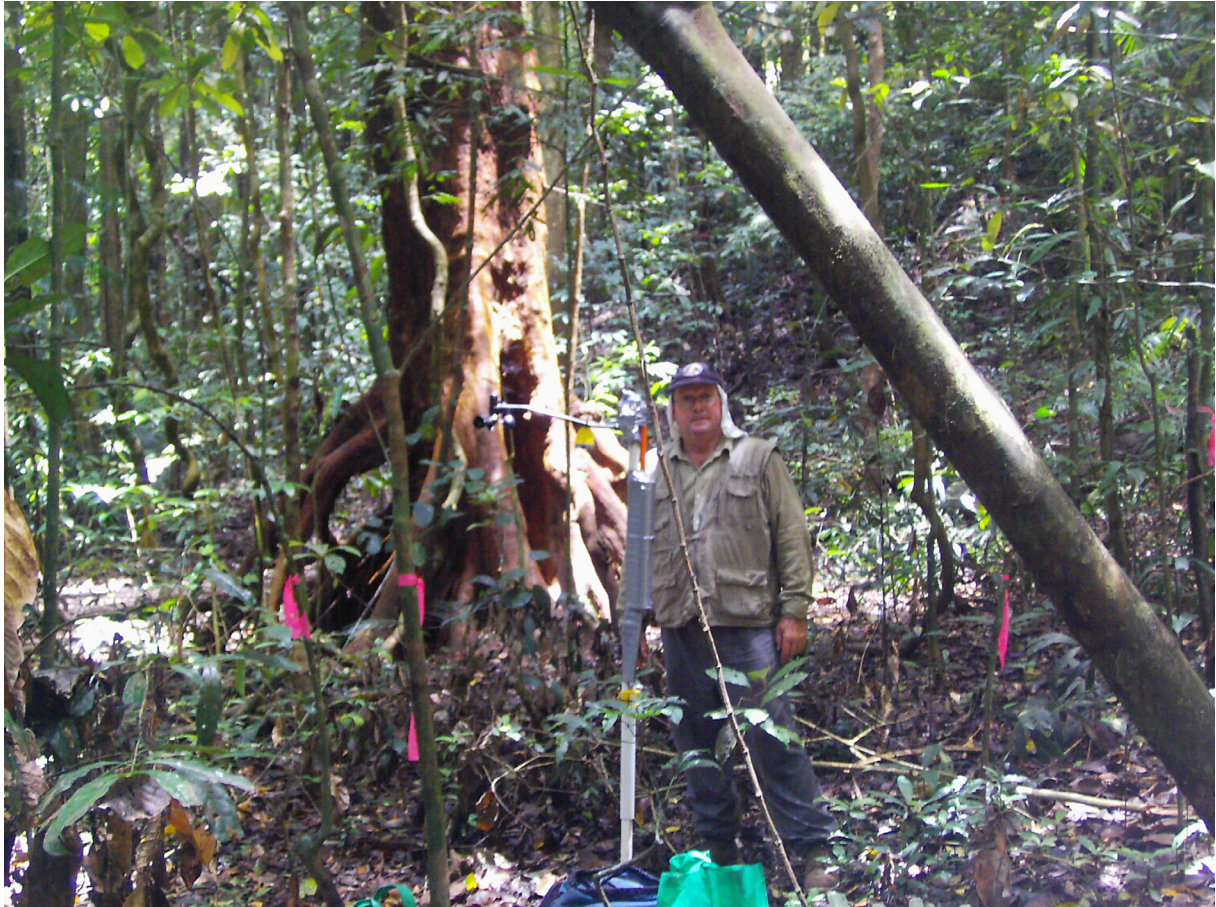
Figure 4: The instruments used to measure diurnal variation in microclimate were supported on a PVC frame resting on a wooden post. Instruments were attached at a height of 170 cm above the ground surface. The person pictured is Stephen Pohlman, who is standing behind and slightly upslope of the apparatus. Photo by Catherine Pohlman.
