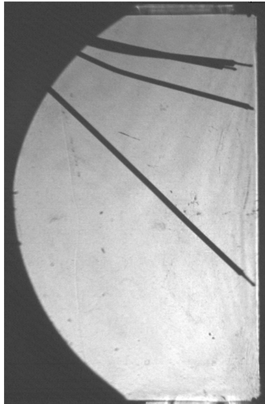
Figure 2.11 Thermistors mounted in the cavity
