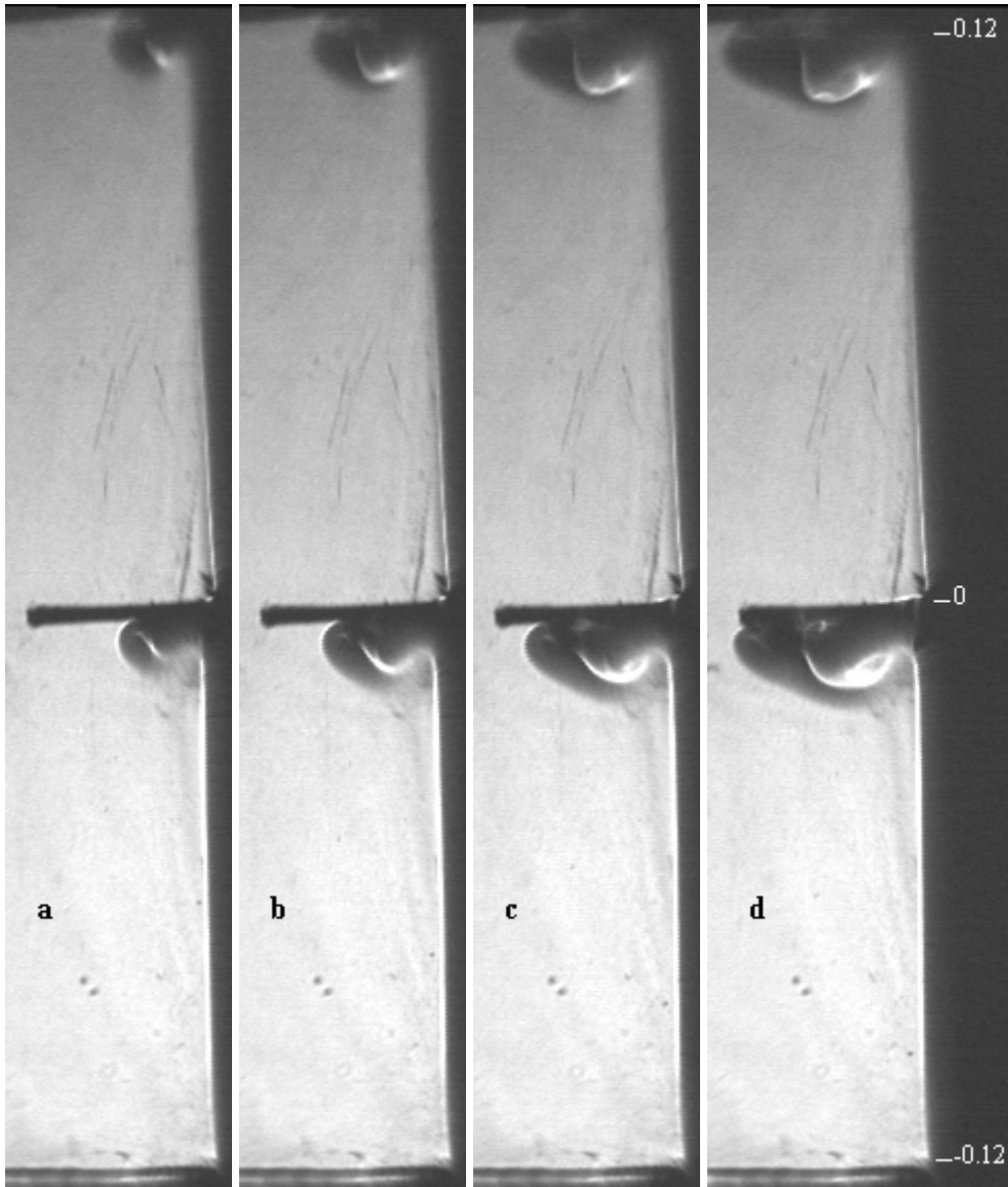
Figure 6.11 Formation of the lower intrusion front (a) t = 14 s. (b) t = 16 s. (c) t = 18 s. (d) t = 20 s
