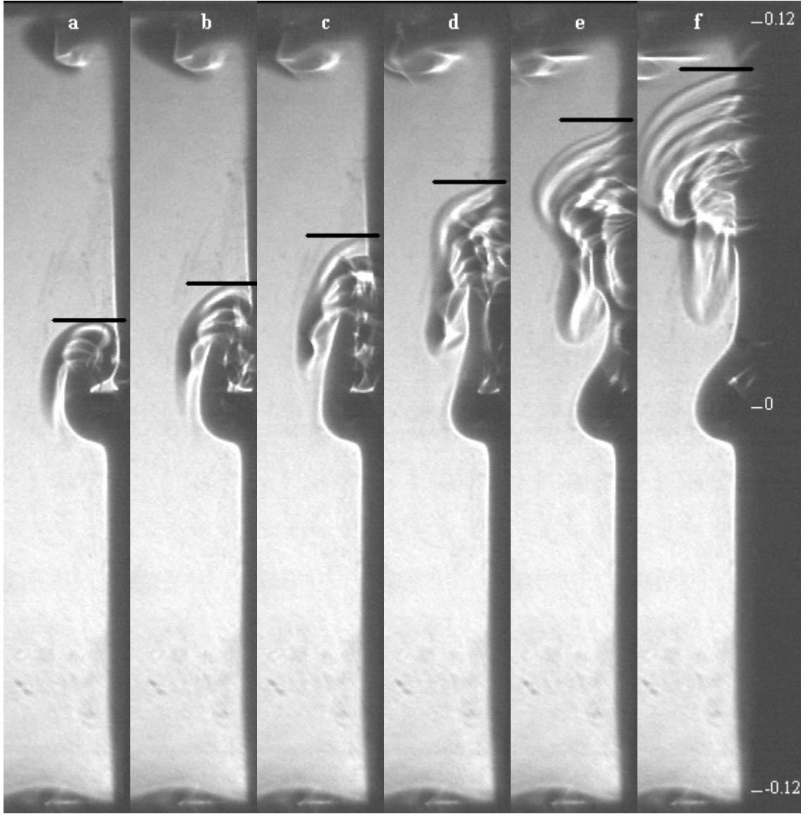
Figure 6.2 Reattachment of the lower intrusion front
