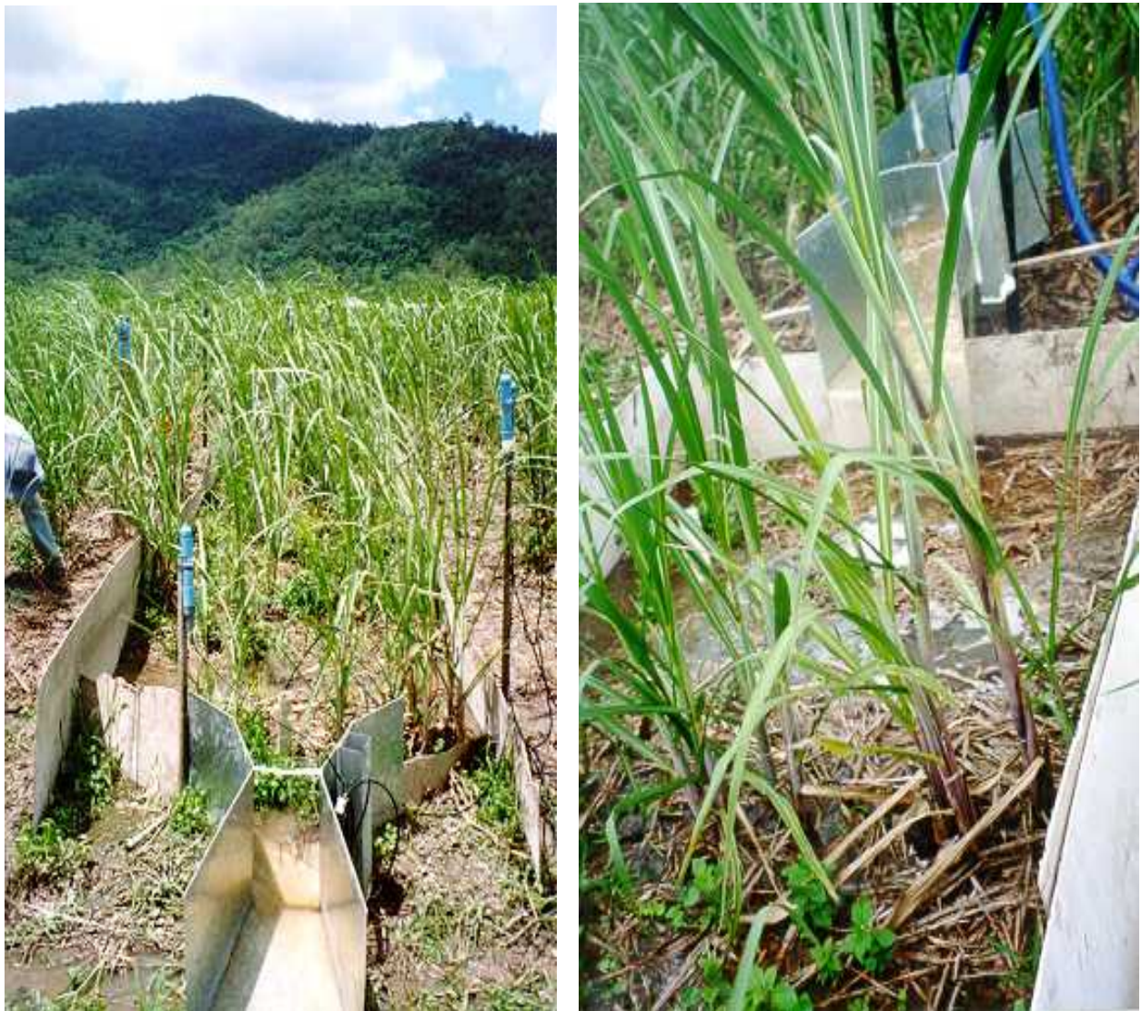
Figure 3.6 Cross furrow (45°) flow experiment showing fibre panels and outflow flume (left) and inflow flume (right).
