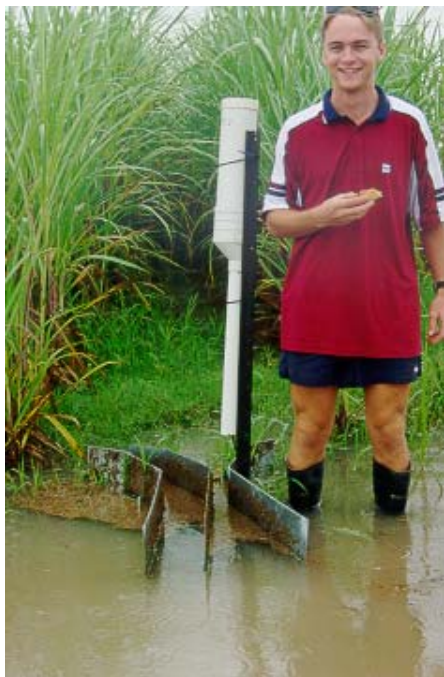
Figure 3.28 An 201 mm (eight inch) flume at the bottom of the Palmas Site inundated by high rainfall
