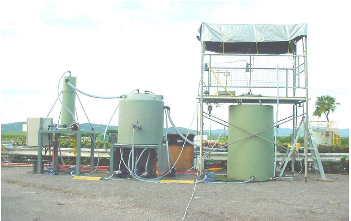
Fig. 3.8 Pilot scale SMBR
