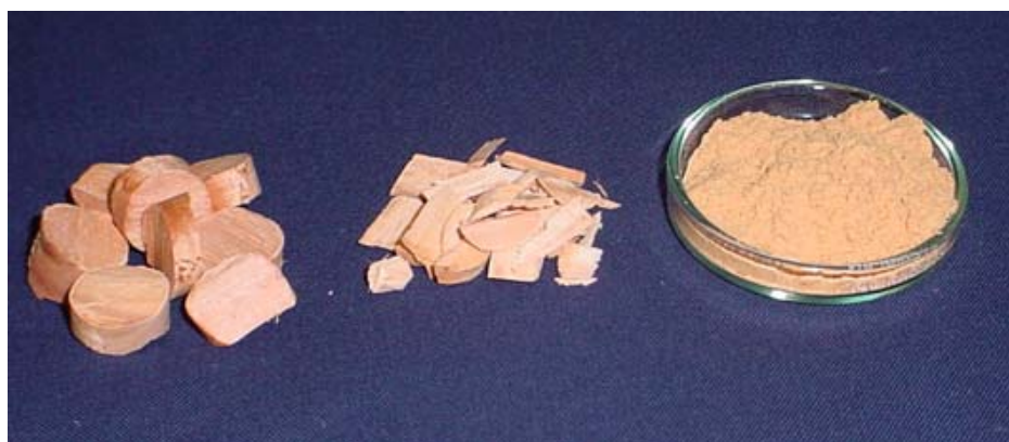
Figure 1. Sandalwood core samples prepared as sliced cores (left) medium chips (centre) and milled powder (right)
