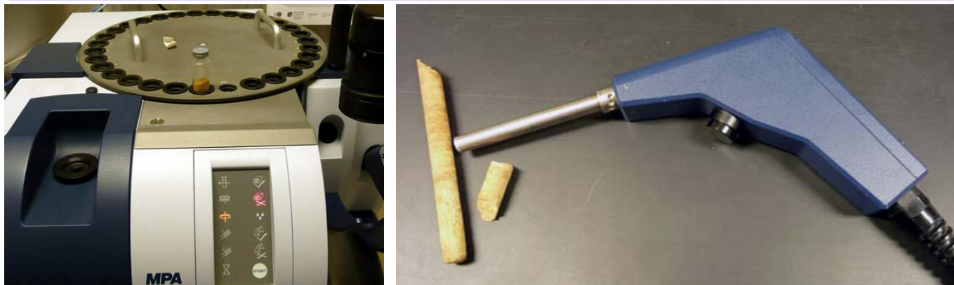
Figure 2. Near infrared bench-top research spectrometer (left) and hand-held solids probe (right) used to evaluate the sandalwood samples.
