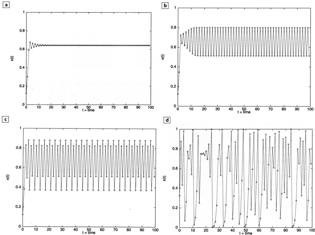
Fig. 7.3 Plots of logistic function for different values of ( $r$ ). (a) Logistic map with  $r=7/10$ . The time series stabilised to a constant value  $x(t)$ . (b) Logistic map with  $r=8/10$ . The time series evolves into a periodic two limits cycle. (c) Case similar to b, with  $r=88/10$ , except that the period has four limits per cycle. (d) Logistic map with  $r=1$ . This latter example has a chaotic time series approximating noise (adapted from Flake, 1998).
