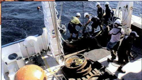
(Below) Deploying a deepwater in-line mooring from the AIMS research vessel RV Solander.
