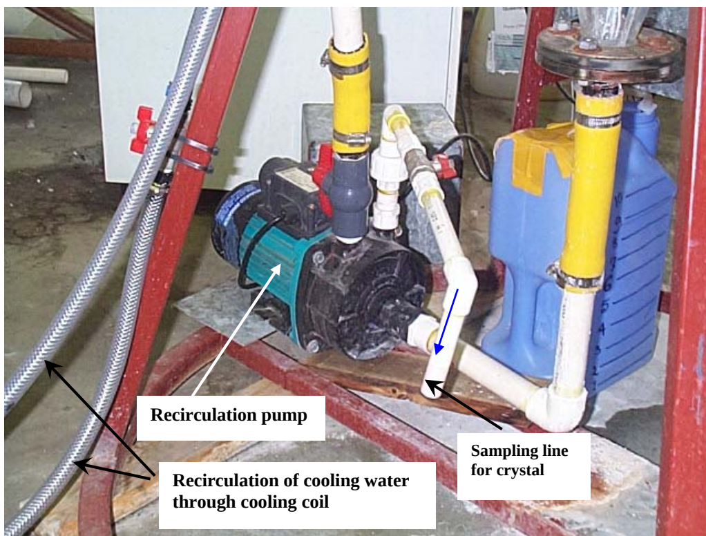
Figure 4. 4 Sampling of struvite crystal through recirculation pump
