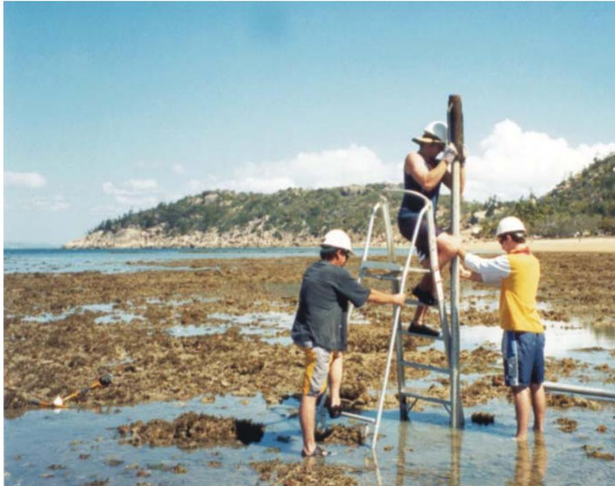
Figure 4.3a. Sediment coring in Nelly Bay. Aluminium pipes were driven into the ground surface with a star picket driver. To gain extra height a 2 m stepladder was used. Average penetration was about 2 m.
