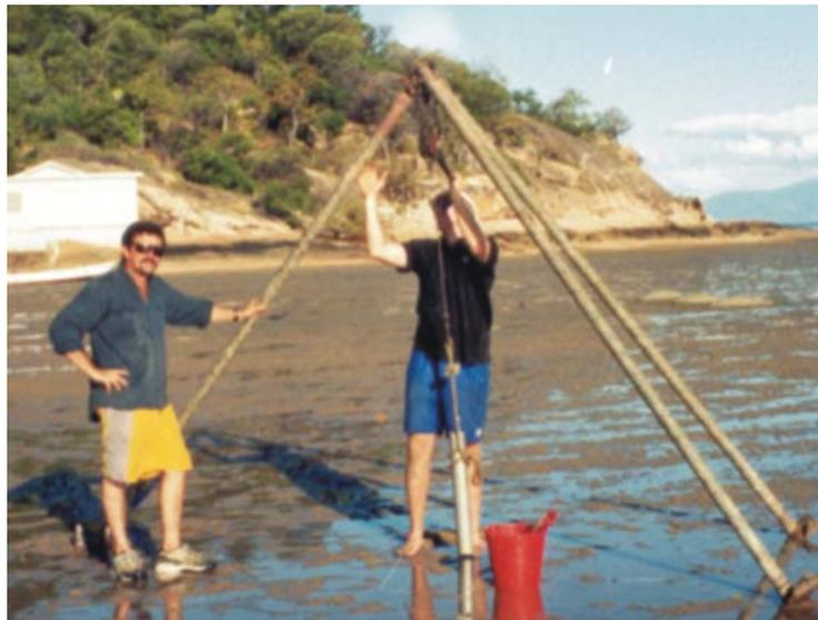
Figure 4.3b. The sediment cores were retrieved using a tripod. The cores were filled with water and sealed with a rubber plug. Typical recovery was approximately 1.5 m.
