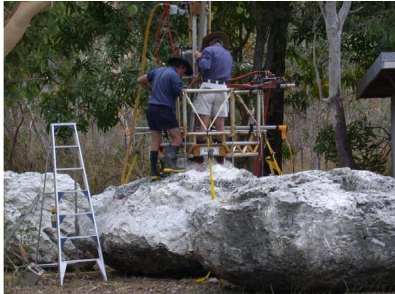
Figure 4.5. The mid-Holocene corals were cored using a hydraulic drill and pump with an aluminium frame (Photo: AIMS).
