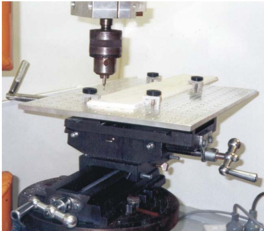
Figure 4.13. Sampling the coral slices. The corals slices were mounted on a moveable stage and, using a stainless steel drill, sampled to 2-5-yearly homogenised increments. The samples were recovered and stored in sterile 5 mL vials. Any residual powder on the slice was removed with pressurised air between samples.
