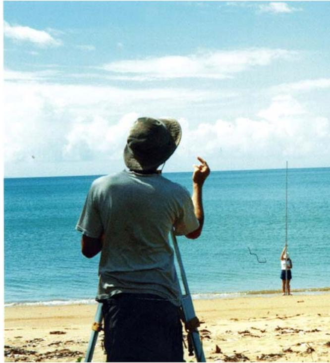
Figure 4.2. Topographical surveying in Nelly Bay using a theodolite.
