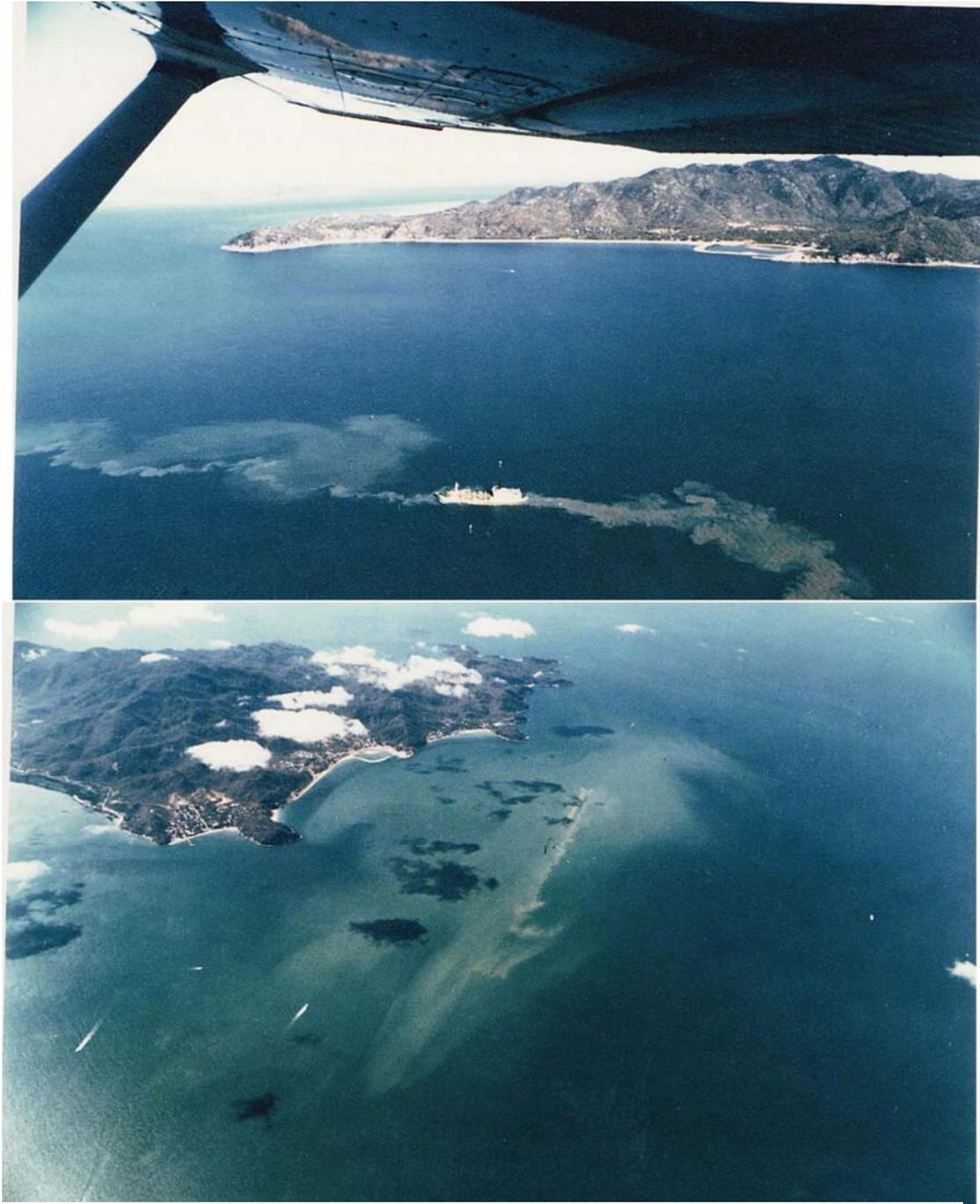
Figure 3.16. The dredge in operation causing turbid water to drift in towards Nelly Bay (Photo: Sinclair Knight Merz; taken from Reichelt, 1993).
