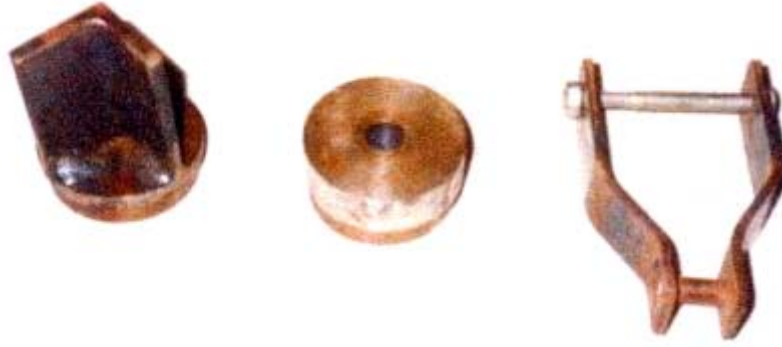
Figure 7.4: Oblique loading cap, axial loading cap and horizontal loading saddle, respectively
