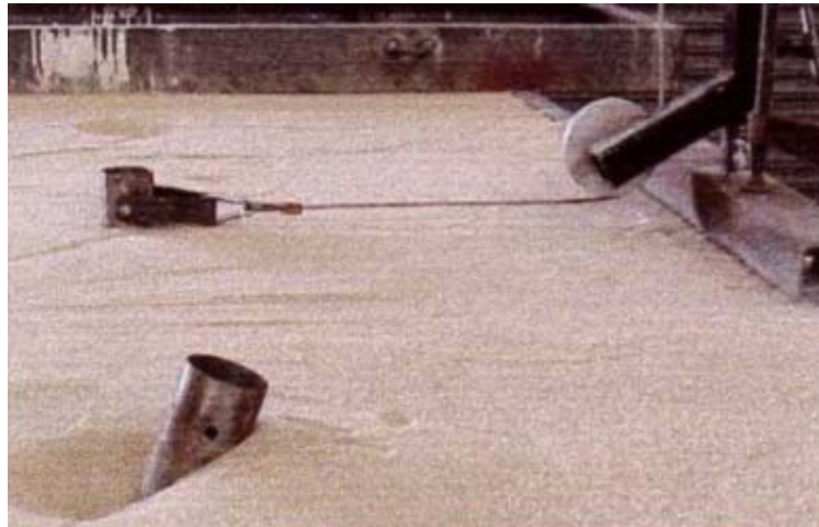
Figure 7.21: Horizontal load on pile with failed pile in foreground
