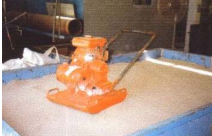
Figure 7.8: Vibrating plate for compaction
