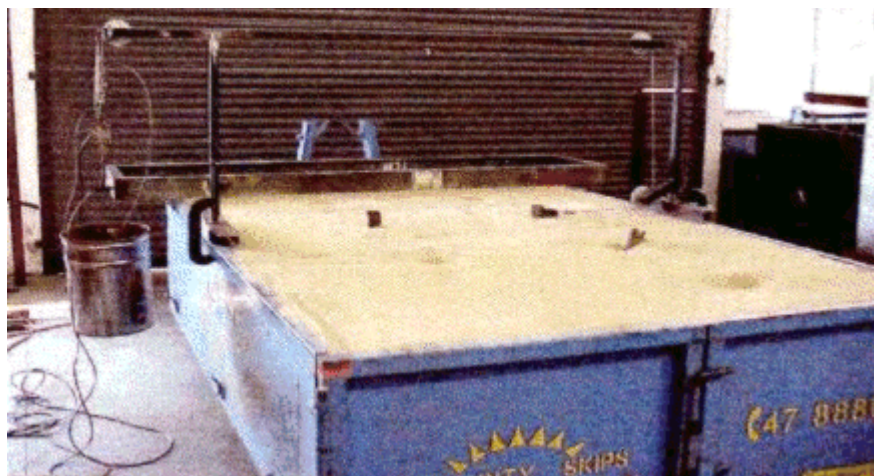
Figure 7.5 (a): Photo of lateral loading arrangement
