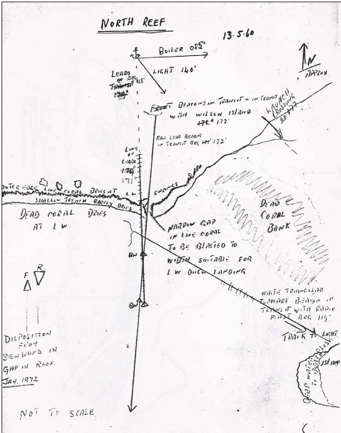
Figure 5.31. The access track to be created for the lighthouse supply vessel at North Reef, 1960.
