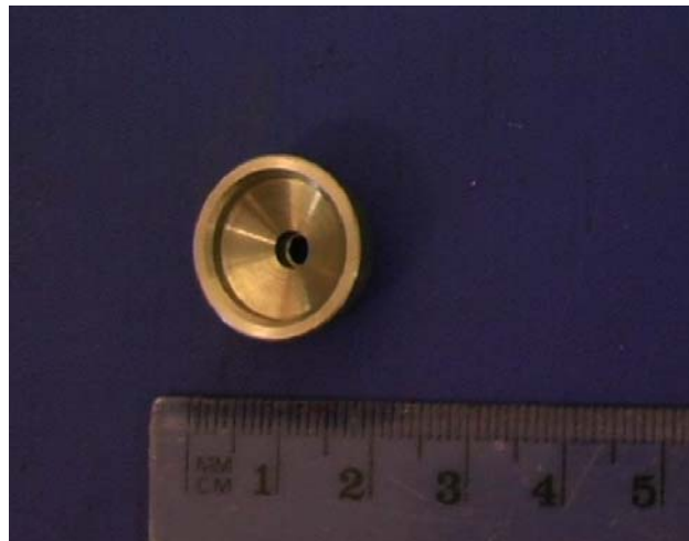
Fig. 3.8 A and B. Spraying combination: Head bore orifice 2 mm bore (A) and nozzle cap 3.5 mm bore/ 2.75 mm bore step nozzle cap (B).
