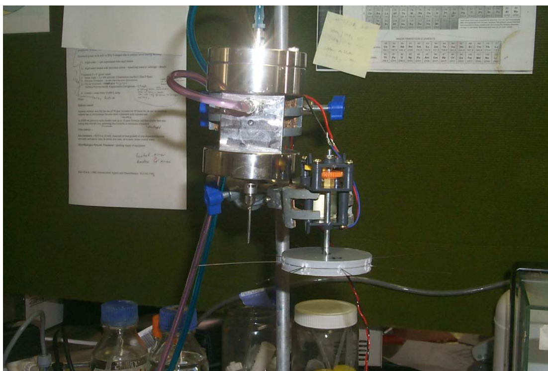
Fig. 4.3. The extruder and mechanical cutting device using to produced complex MC.
