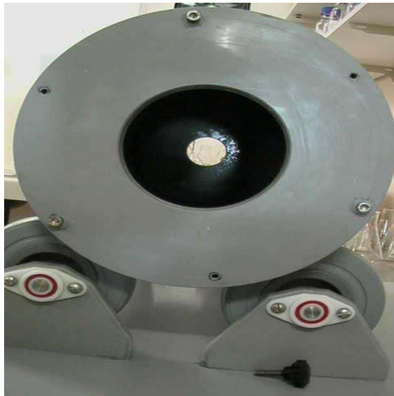
Fig. 3.2 (A and B). The rotating curing chamber/cylinder used to cure sprayed beadlets, containing the curing \text{CaCl}_2 solution. A, Top/ front view of rotating chamber; B, Side view and opening to chamber bath (Design based on C.J. Langdon and M.A. Buchal, 1998). The chamber volume for the curing bath is 2 L. The rotation speed of the chamber is determined by the user.
