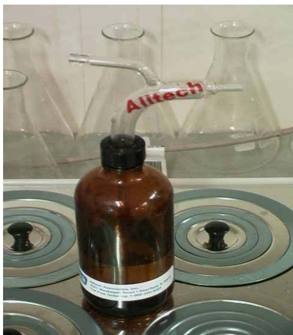
Fig. 3.1 (A and B). The Alltech Inc. hand held glass atomisers. A, Apparatus used for production of fine particles and B, Coarse particles. The atomisers each held 250 mL. The diet mixture can be preheated within a water bath prior to spraying.
