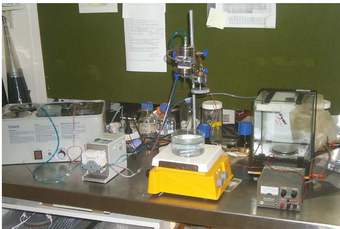
Fig. 4.2. The production device used to produced complex MC, including extruder, cutting device and curing bath.
