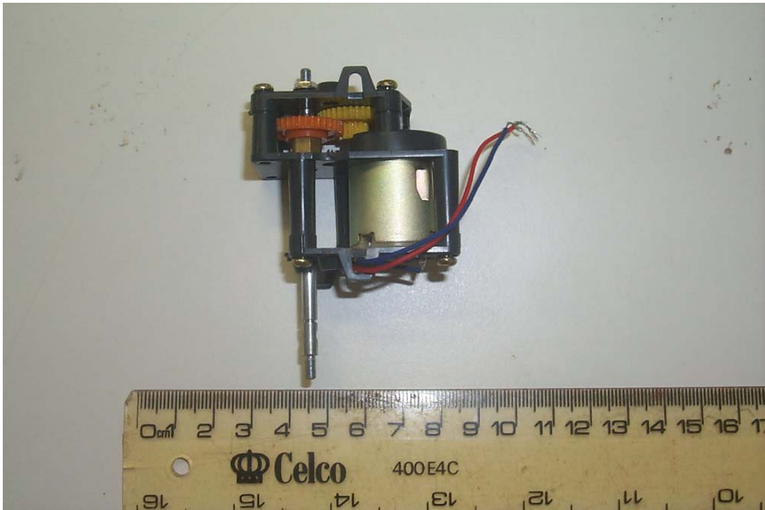
Fig. 4.4. The motor that drives the mechanical cutting discs. (Operating range of 200-1000 RPM).
