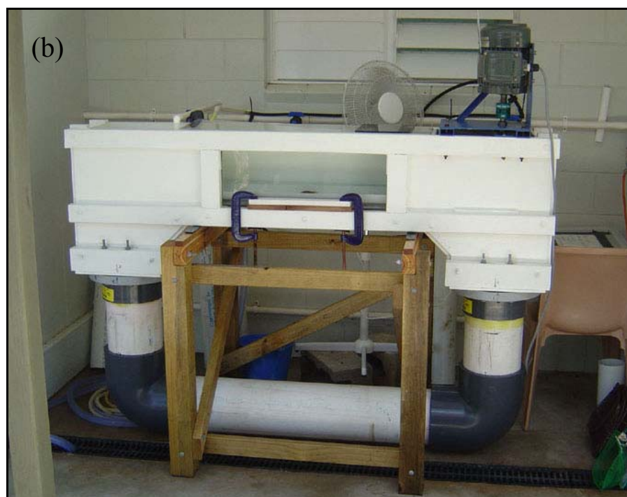
Fig. 1.1. (a) Cross-sectional diagram of 194 L recirculating flow tank used for gypsum calibration trials. (b) During operation the tank is oriented vertically with the working section open at the top. Design and construction followed Vogel & LaBarbera (1978).
