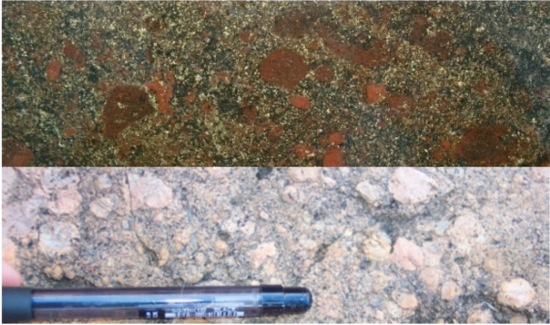
Figure 5. a) Top – typical Ernest Henry ore breccia with hematite-K-feldspar altered clasts in a magnetite-chalcopyrite-pyrite-K-feldspar-calcite±barite-titanite matrix. b) Bottom – typical breccia from a breccia pipe emanating from the Mt Angelay Granite and crosscutting Soldiers Cap Group schists, from the western edge of the Snake Ck anticline, with albite-actinolite-magnetite±K-feldspar-chlorite clasts set in an albite-magnetite-hematite-actinolite matrix. Scale is similar in both photographs.
