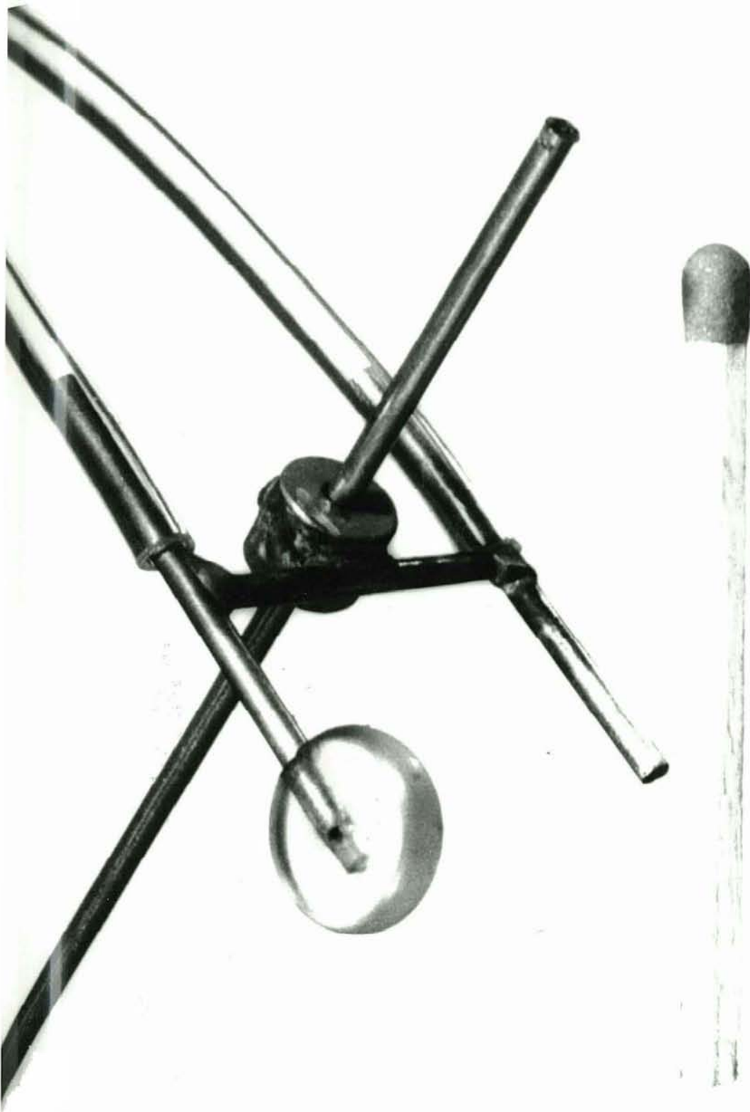
Figure 4.15 Photograph of pressure probes.
