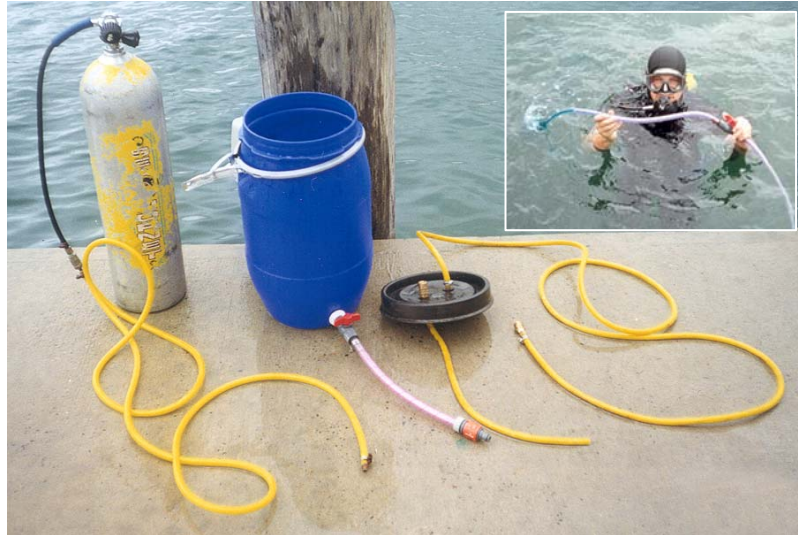
Plate 4.1 The deployment pump consisting of (from left to right); SCUBA tank with air inlet hose; 35 L drum fitted with on/off tap (red tap) at the start of the hose; lid, fitted with coupling for connection to air inlet and internal hose (attached air-stone not shown) and external hose fitted with pressure relief valve (42 Kpa). Inset: diver holding the end of the hose with diver controlled on/off tap.
