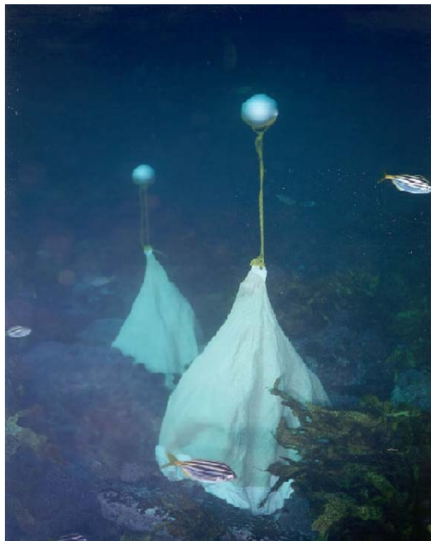
Plate 4.2 Two of the five physical shelters, each covering 1 m 2 of substrata and consisting of a weighted skirt (chain filled light coloured material at base) and the body of the shelter (woven plastic cloth) fitted with an eyelet and attached buoy, positioned on the reef.
