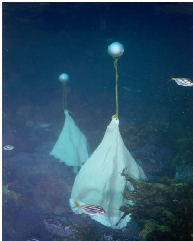
Plate 4.2 Two of the five physical shelters, each covering 1 m 2 of substrata and consisting of a weighted skirt (chain filled light coloured material at base) and the body of the shelter (woven plastic cloth) fitted with an eyelet and attached buoy, positioned on the reef.
