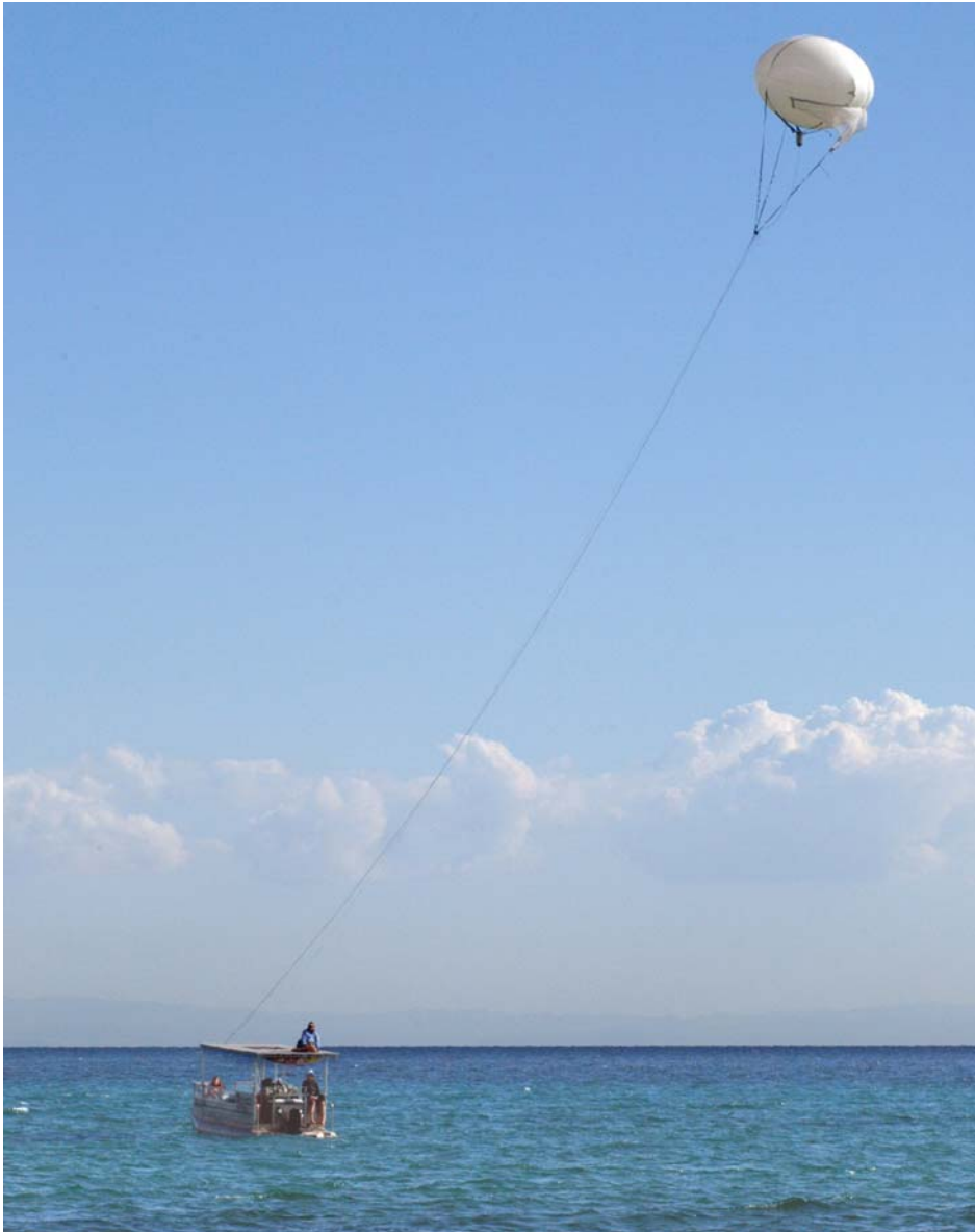
Figure 3.3. At study site MB1 I evaluated the use of a remote-controlled aerial video system, supported by a helium-filled balloon. The equipment had originally been developed for studying herds of dugong ( Dugong dugon ) and had served well in that role (Hodgson, 2004). In contrast the equipment proved unsatisfactory for behavioural studies of green turtles. Photo courtesy K. Stockin.
