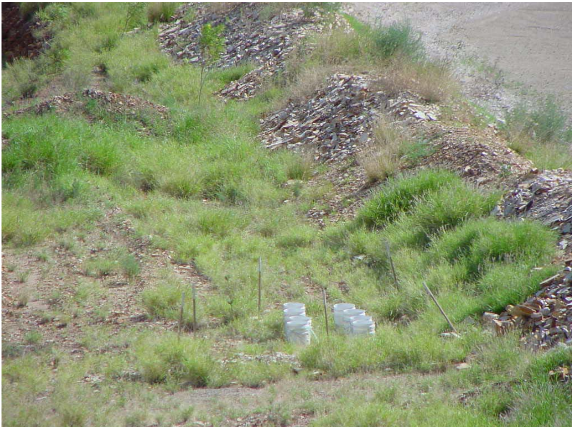
Plate 3.6. Field leach columns in place, Galah North pit.
