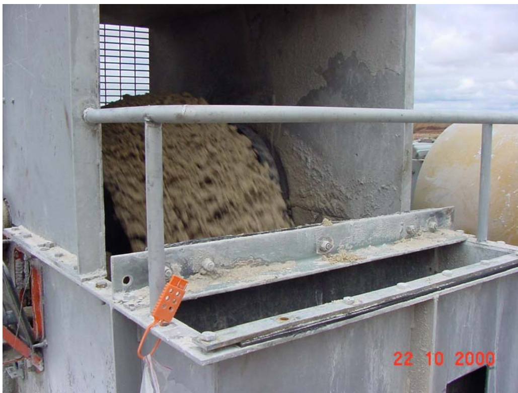
Plate 3.5. Sampling point: HH PG being discharged from overland conveyor into re-slurry tank.
