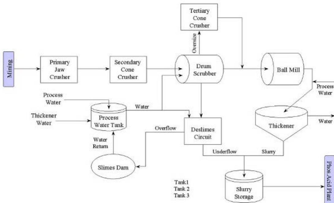
**Figure 2.11. Phosphate Hill beneficiation plant process flow chart (from WMCF Intranet live production pages).**
