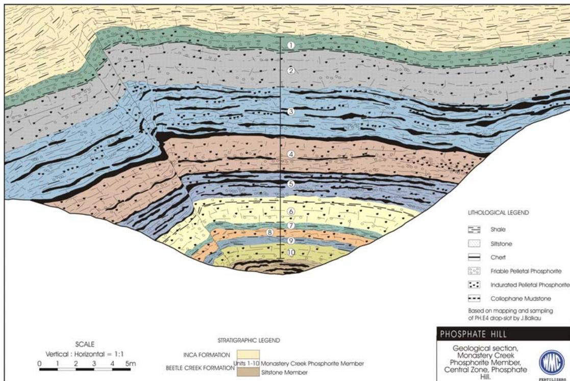
**Figure 2.6. Cross-section of exploration trench showing typical mining sequence, Phosphate Hill (north and central zones): Inca Shale (overburden), Monastery Creek Phosphorite Member (ore, divided in 10 units of variable grade) and Lower Siltstone Member (footwall). After Rogers and Crase 1979.**
