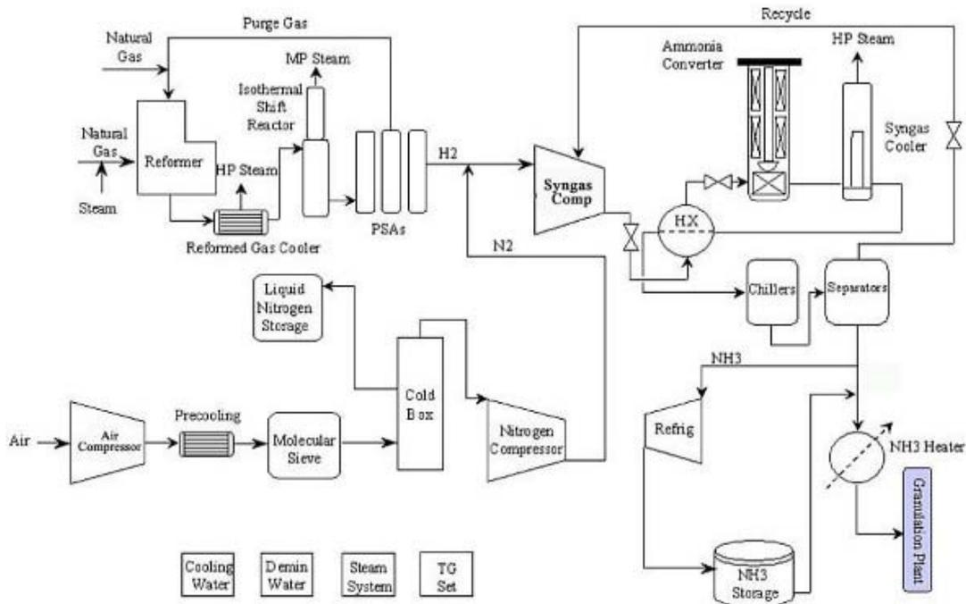
**Figure 2.14. Phosphate Hill ammonia plant process flow chart (from WMCF Intranet live production pages). Hot processing side in the upper half of the diagram, cold in the lower half.**
