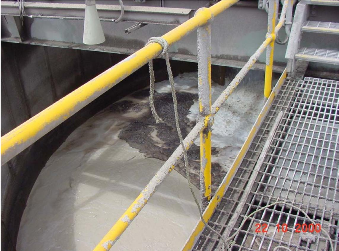
**Plate 2.13. Hemihydrate PG and acid process water being mixed in the re-slurry tank. The black substance floating on the top is believed to be of organic origin.**
