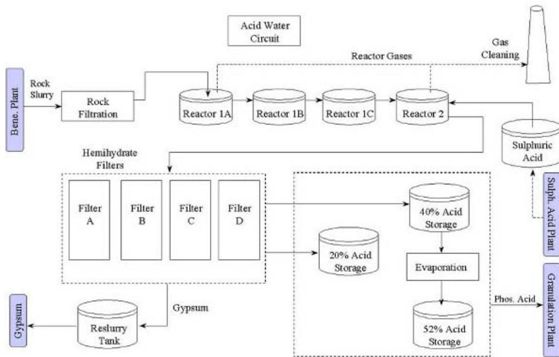
**Figure 2.12. Phosphate Hill phosphoric acid plant process flow chart (from WMCF Intranet live production pages).**
