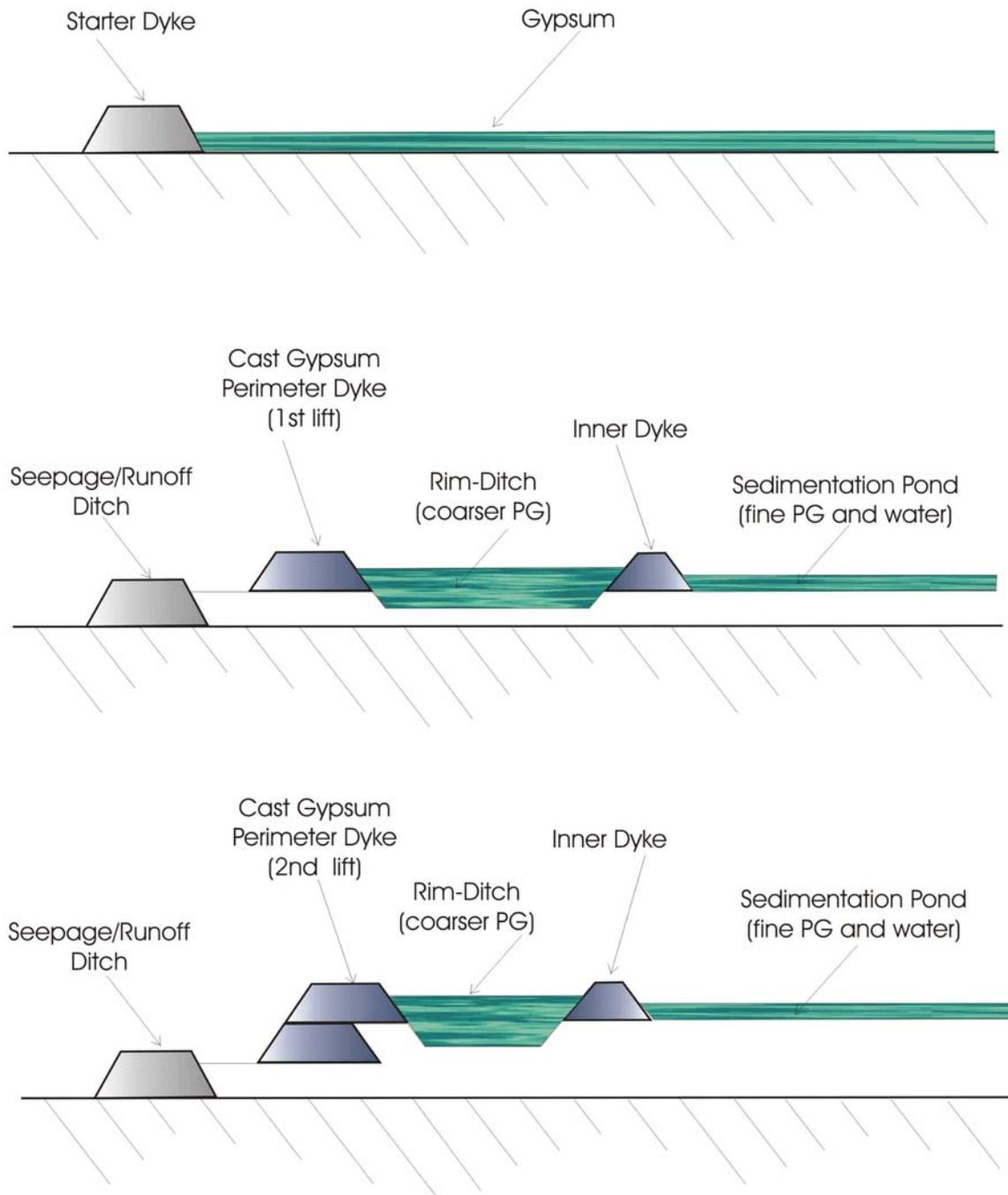
**Figure 2.18. Schematic of PG wet-stack construction method as used at Phosphate Hill (adapted from Ardaman 1999).**
