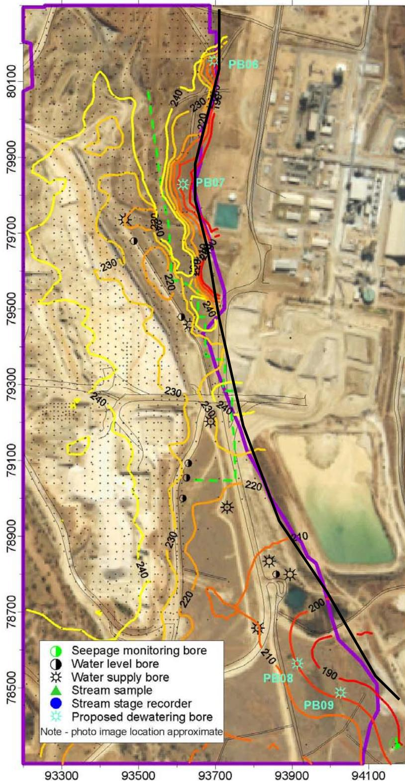
**Figure 2.9. Phosphate Hill production bore field as at June 2004. Coloured contours = hanging wall mRL, dashed green line = projected final Galah Pit outline. Black line = approximate position of Mehaffey Creek Fault. North is to the top of the page. Fertilizer plant and slimes dam east of Mehaffey Creek Fault, Galah Pit to the west. Image from Berry *pers. comm.*, 2004.**
