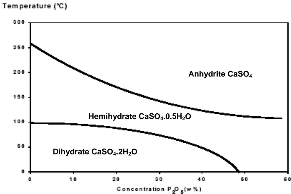
**Figure 2.13 Phase diagram controlling gypsum species formation in phosphoric acid plants (from Gobbitt and van Ede 2004).**
