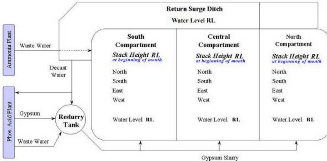
**Figure 2.17. Phosphate Hill PG stack process flow chart (from WMCF Intranet live production pages).**
