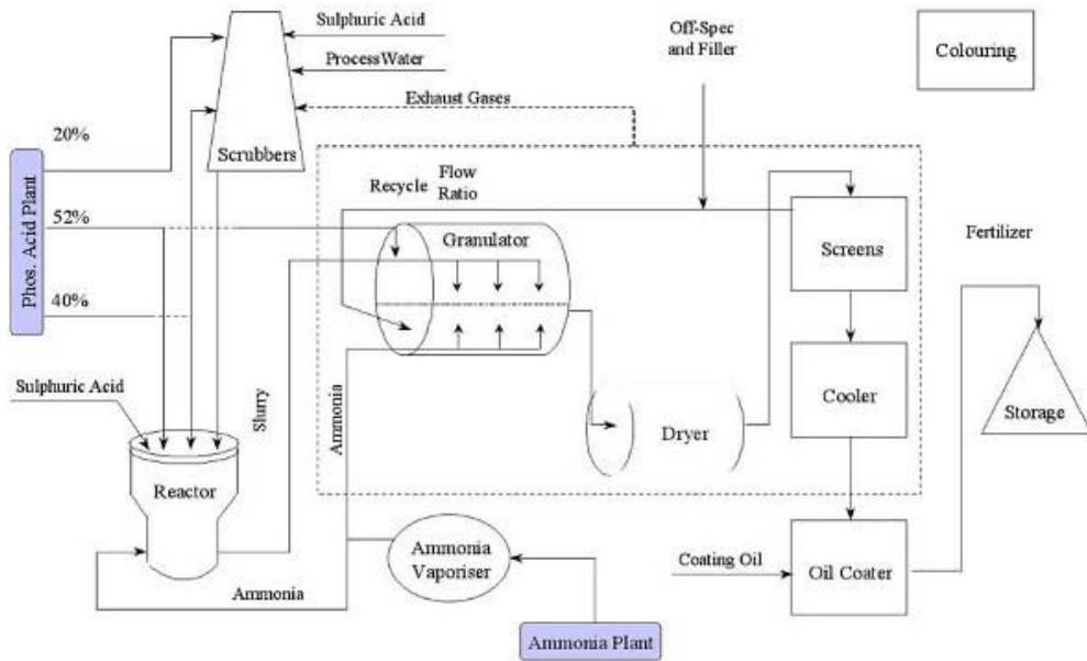
**Figure 2.15. Phosphate Hill granulation plant process flow chart (from WMCF Intranet live production pages).**
