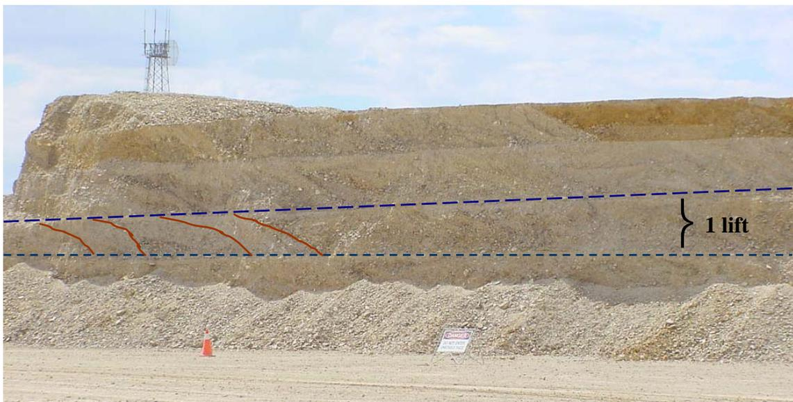
**Plate 2.7. Partially recovered ROM stockpile 2. 4.5 lifts are visible with a fifth obscured behind the rill at the base of the stockpile. Individual truck dumps that have been flattened by a bulldozer are also visible (brown lines). Stockpile construction is orthogonal to this face. Ore affected by iron hydroxide alteration appears as orange in the upper lifts.**
