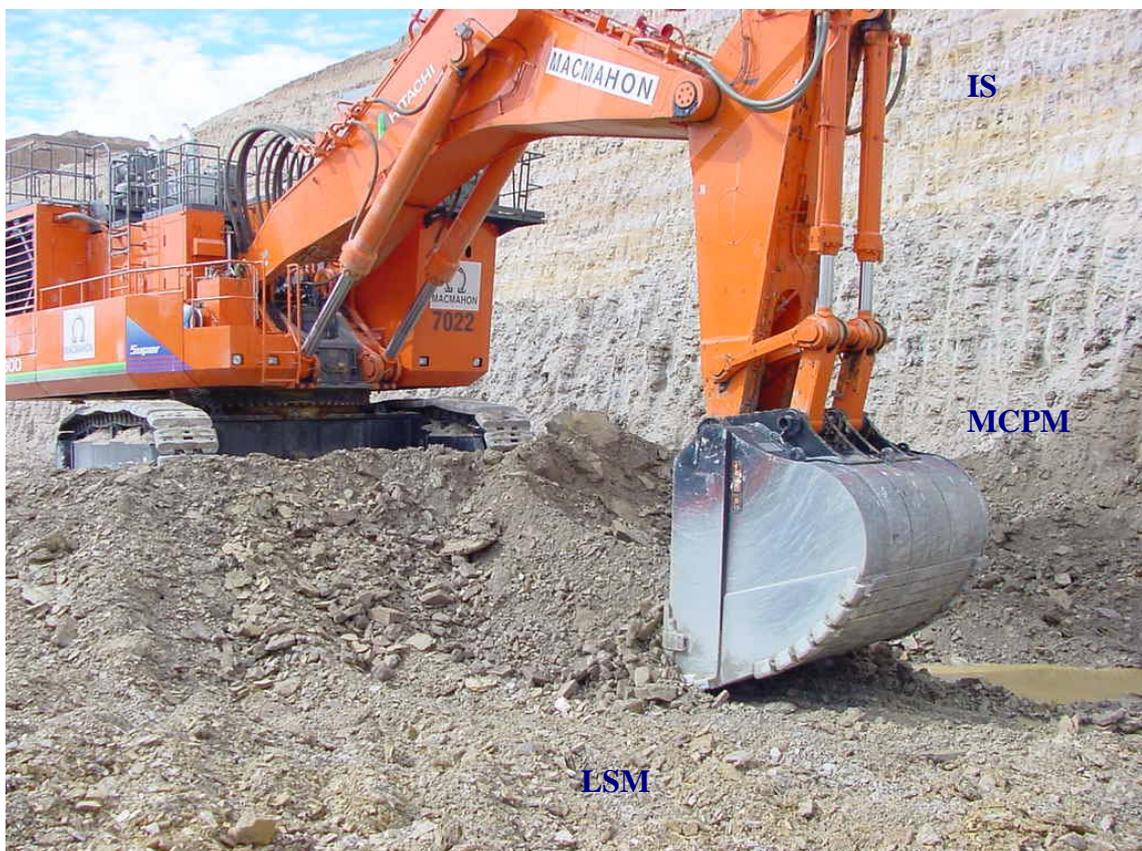
**Plate 2.6. Footwall cleanup, Galah pit parcel 602, September 2003. The 200 tonne excavator peels the ore (grey MCPM) from the footwall (yellow LSM), following the contours of the contact. Also visible in the background is the Inca Shale overburden.**
