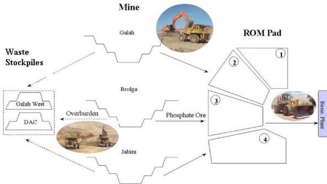
**Figure 2.10. Phosphate Hill mining process flow chart (from WMCF Intranet live production pages).**
