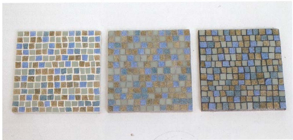
Plate 4.4.3 Grout study, each tile is the same colour in the same place with different grouts, (King, 2003: 97).
