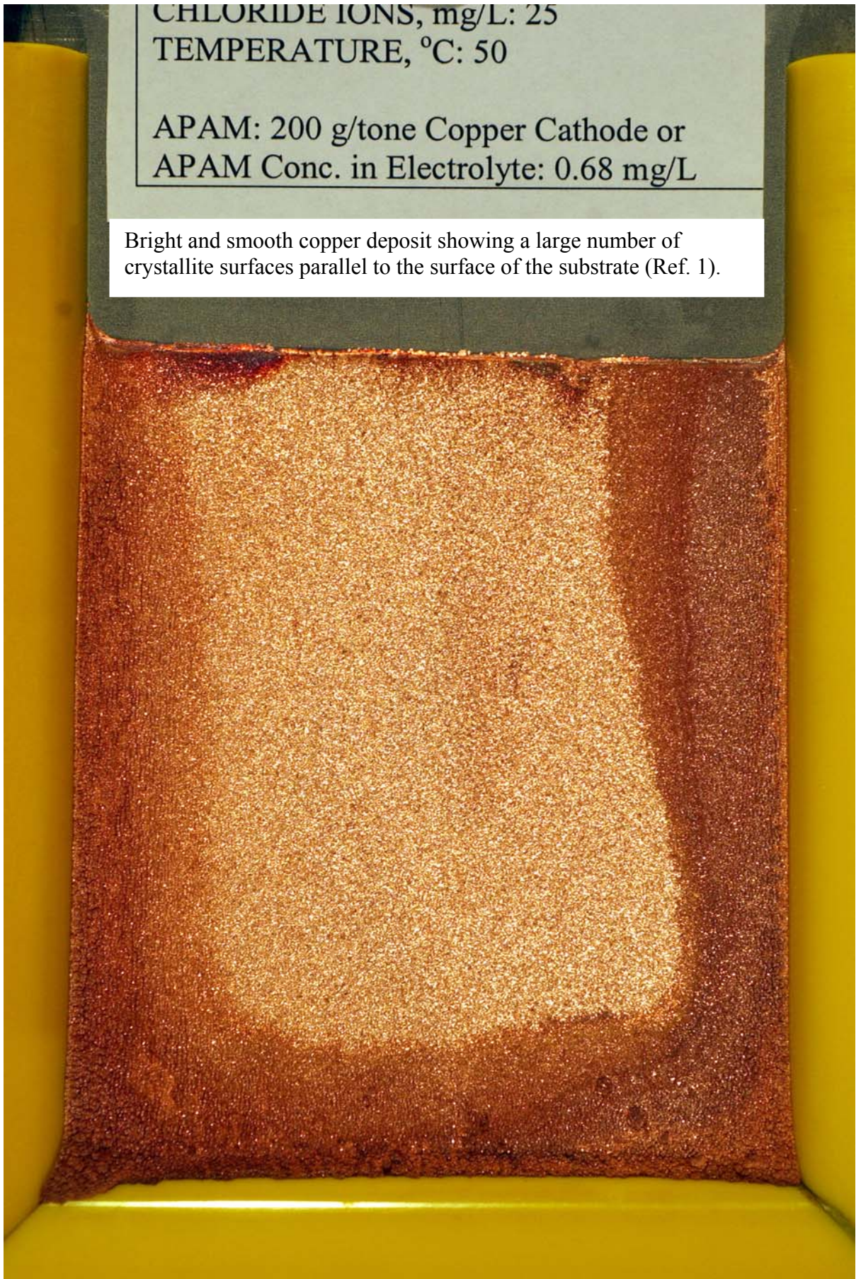
Figure 6-90: Copper Deposit Obtained with APAM at 340\text{A/m}^2 and 44hours-35minutes
