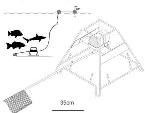
Figure 1: Up to 12 BRUVS were set simultaneously on the seabed to identify and count shoal fishes in paired, "fished-unfished" comparisons. Each replicate produced one hour of footage. *Survey design and analyses*
