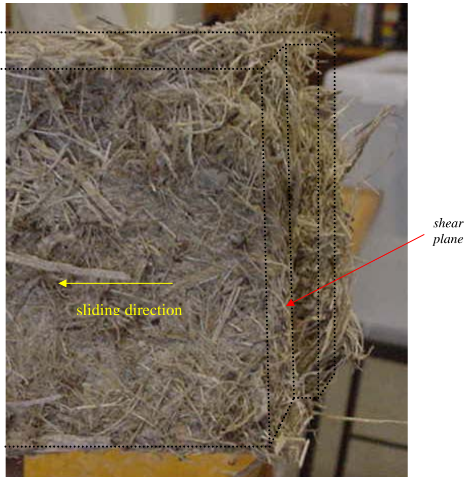
Figure 6.2 Evidence of the shear failure of bagasse after having been pushed 14 mm.
