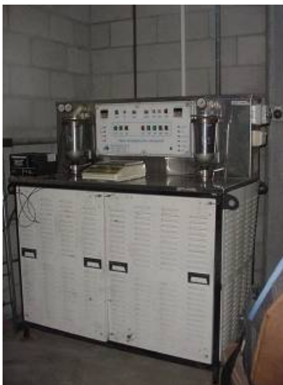
Figure 4.2 Fibre machine, apparatus for determining the fibre content in bagasse (after Loughran et., al. 1988).
