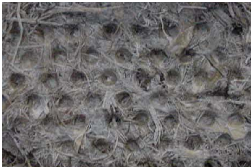
Figure 6.1 Traces left by asperities on bagasse after contacting a roughened steel flat platen at 1000 \text{ kg/m}^3 compaction.
