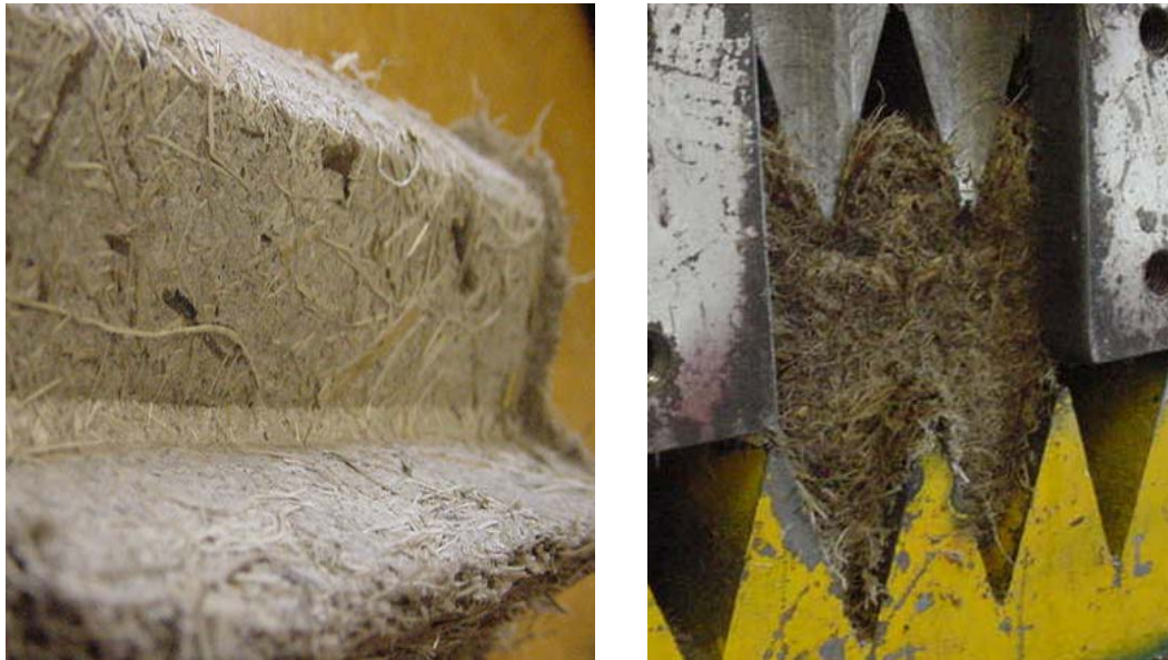
Figure 6.8 (a) Aligned appearance of fibres under 1000 \text{ kg/m}^3 compaction, smooth, 100^\circ groove angle. (b) Randomised appearance of fibres under 400 \text{ kg/m}^3 compaction, 2.25mm height of asperity, and 35^\circ groove angle.
