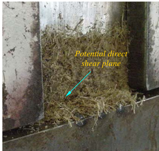
Figure 6.5 The friction coefficient test at 1000 \text{ kg/m}^3 compaction, 180^\circ groove angle, and 2.25 \text{ mm} average roughness. Potential slippage outside the interface.
