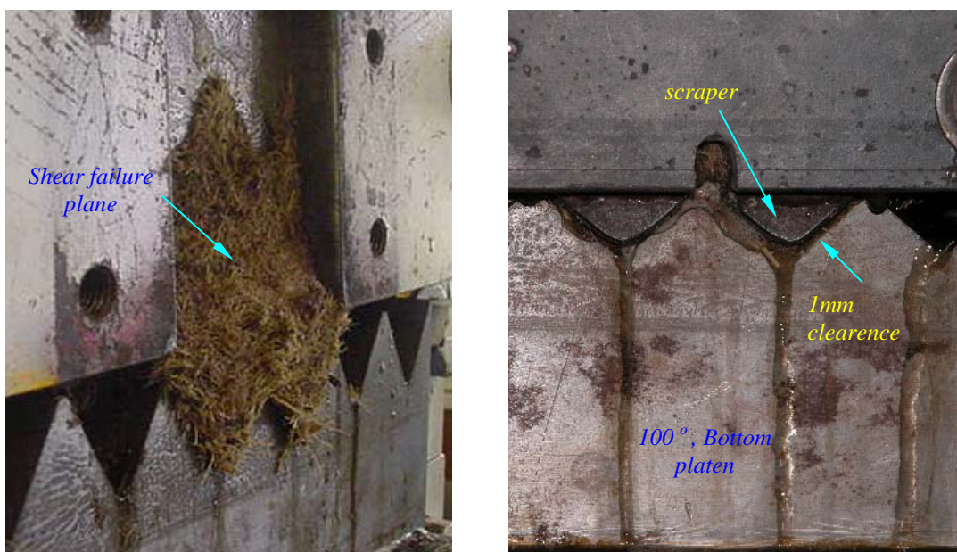
Figure 5.25 Shear and friction coefficient measurements: (a) shear test without scraper; (b) friction coefficient test using scraper to avoid internal shear failure.
