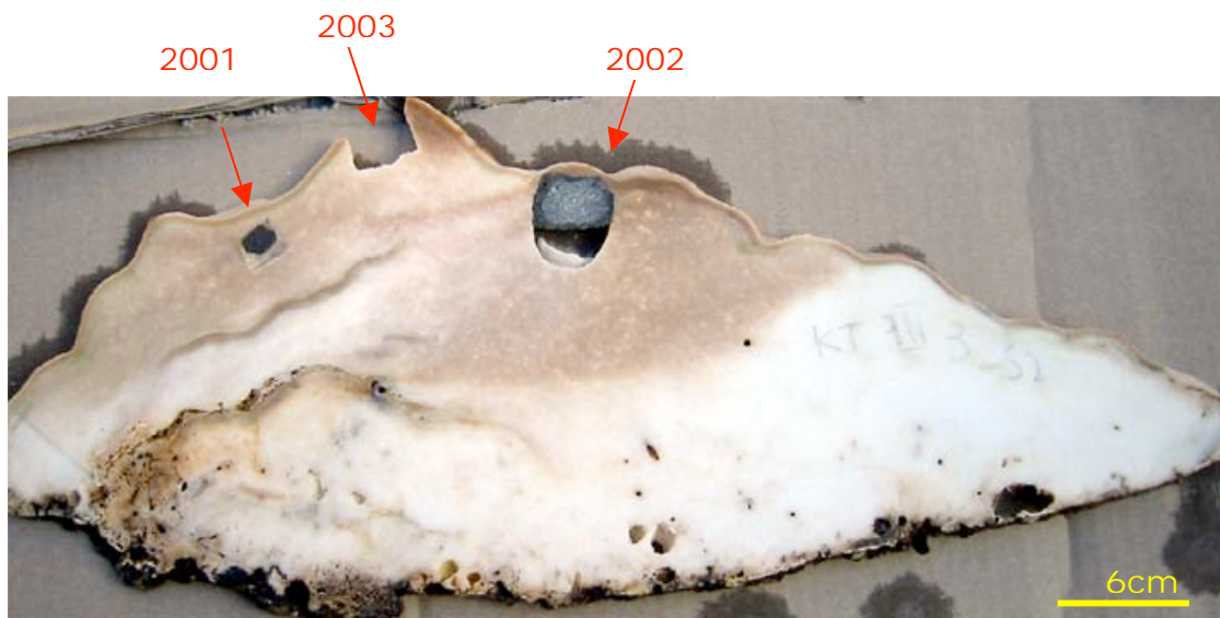
Plate 5. Slice through coral skeleton from a colony from deep water at an impact site. Arrows indicate cores taken in respective years. The overgrown concrete plug from 2002 is obvious. Tissue thickness can be seen as the thin brown band on the surface of the colony.
