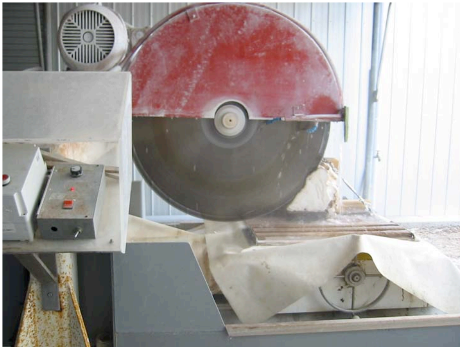
Plate 6. Circular saw with masonry blade cutting coral colony at AIMS.
