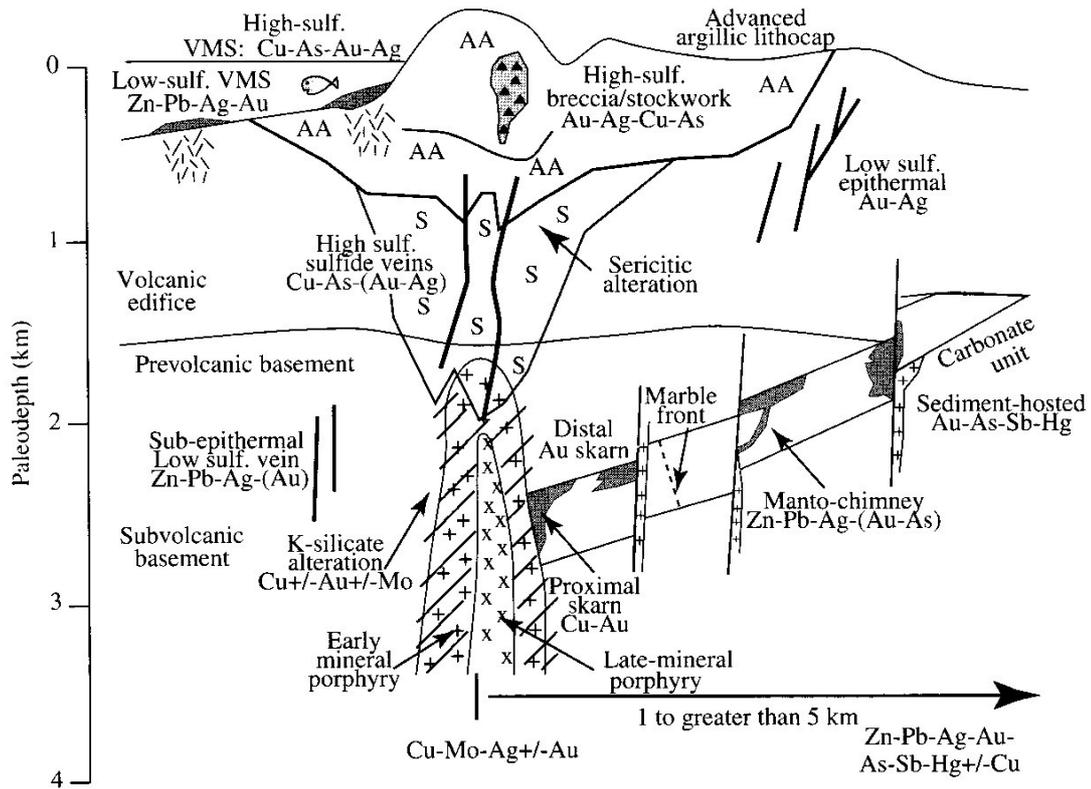
Figure 1-2 Ore deposit environments related to porphyritic intrusions
