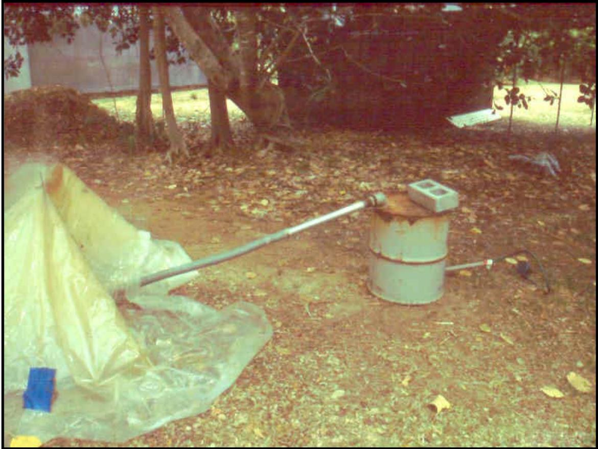
**Figure 4.3.** Apparatus used to produce smoke at ambient temperature. Smoke was produced within the drum and pumped through the metal pipe into the tent, in which seeds were exposed to the smoke.
