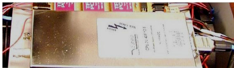
Figure 5.26. High Voltage Power Supply for ION Getter Pump
