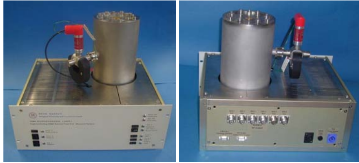
Figure 7.1. Pictures of D7 front and back showing the new N-type connectors for RF input (top of cryostat) and output (back panel)
