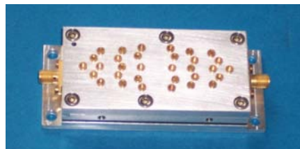
Figure 5.12. Filter Housing with Small Air Hole in the Top Left Hand Corner
